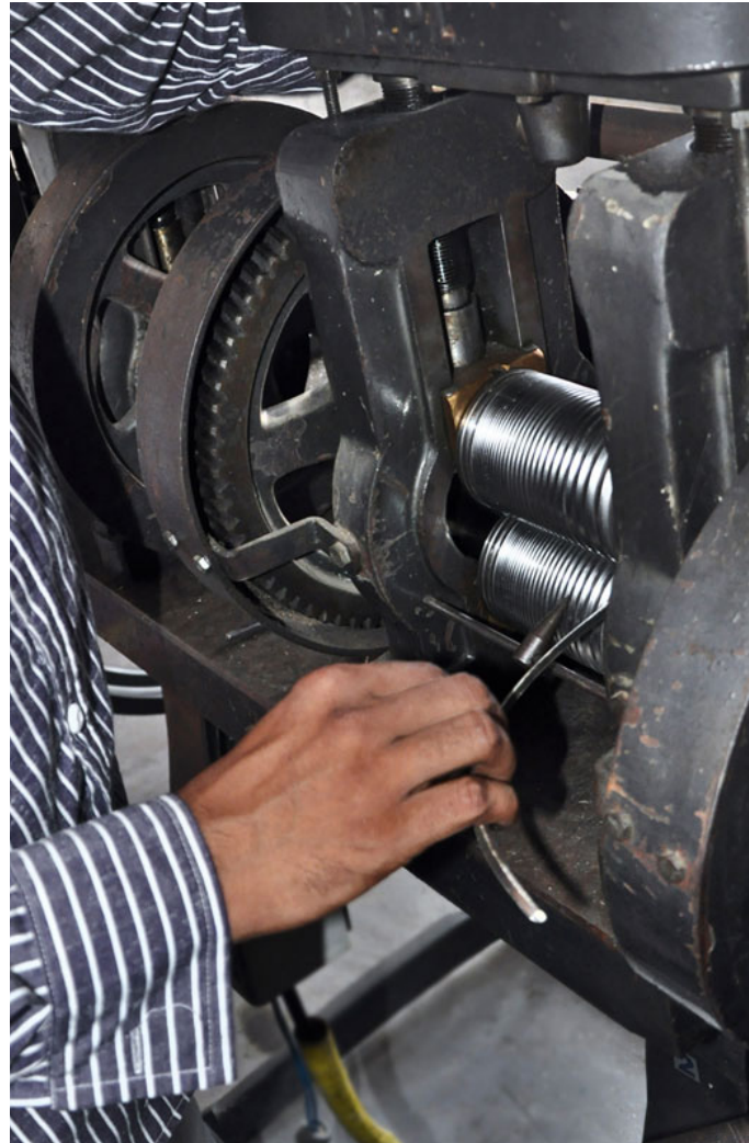
Here the silver rods are stretched to make it thin in size.
