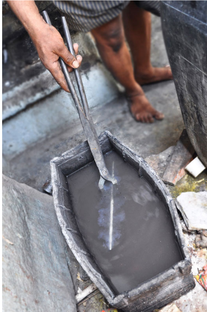
The silver rod is removed and dipped in the cold water to make it cool.
