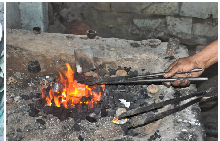
With the help of the iron tongs, biscuits are lifted and checked to ensure proper melting of silver.
