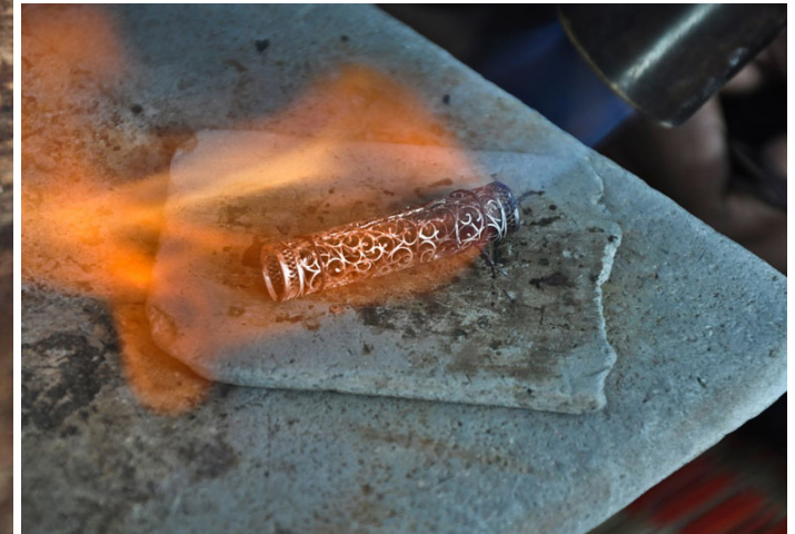
Burning process is done repeatedly for proper binding.
