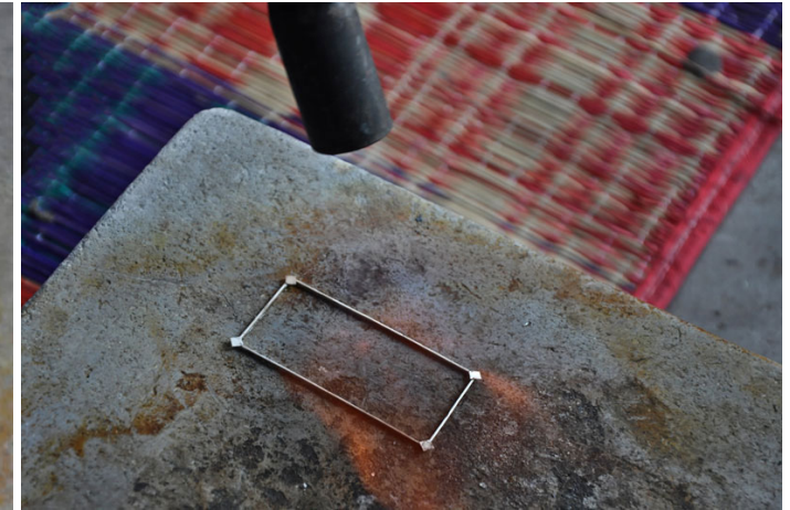
The edges are welded to join.
