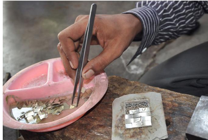
Small thin silver pieces are placed on the frame for welding.
