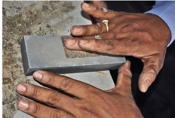
The worked piece is rubbed over the sand stone to make it smooth.
