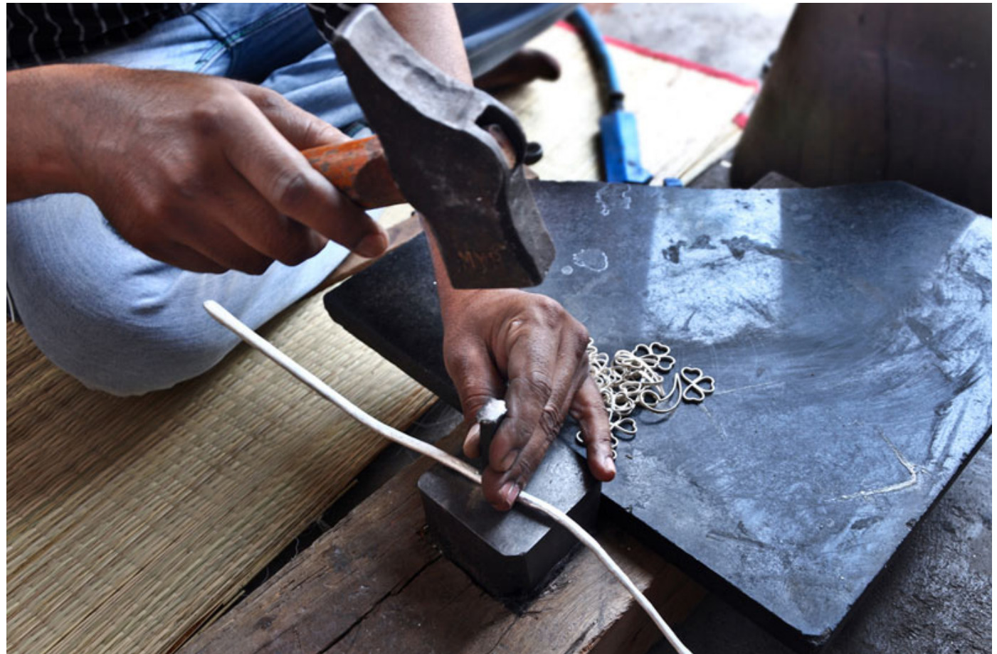
Using hammer, silver rods are cut into small pieces.
