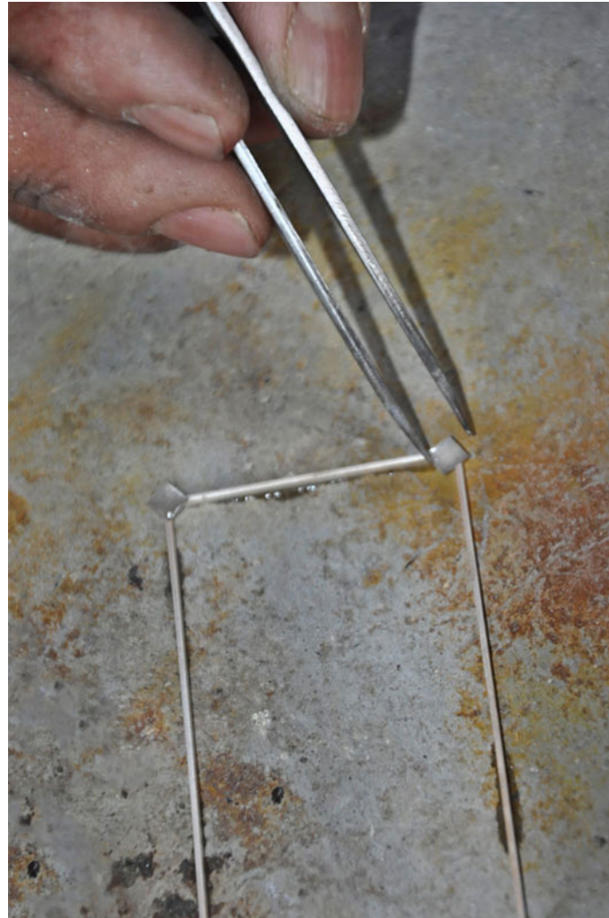
Four silver strips are aligned to form rectangular shape. Basic frame is ready for designing process.
