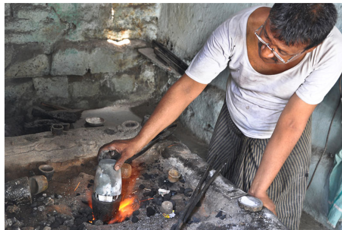
To get the temperature high another crucible is closed on top of it.
