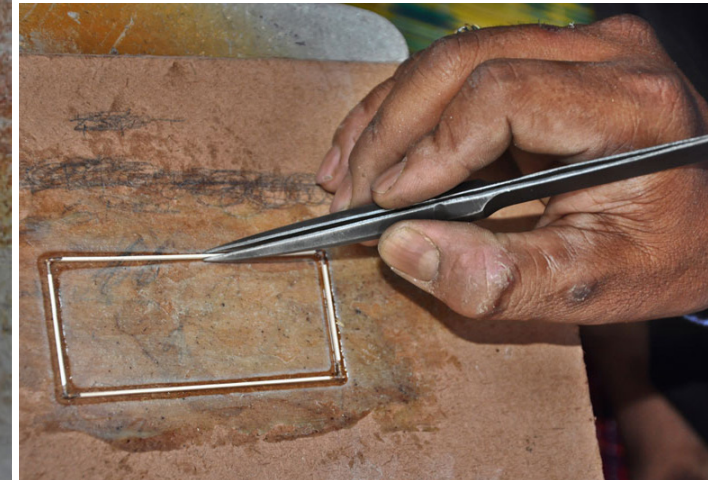
Four silver strips are aligned to form rectangular shape. Basic frame is ready for designing process.
