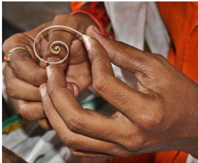
Silver wire is twisted to make design.
