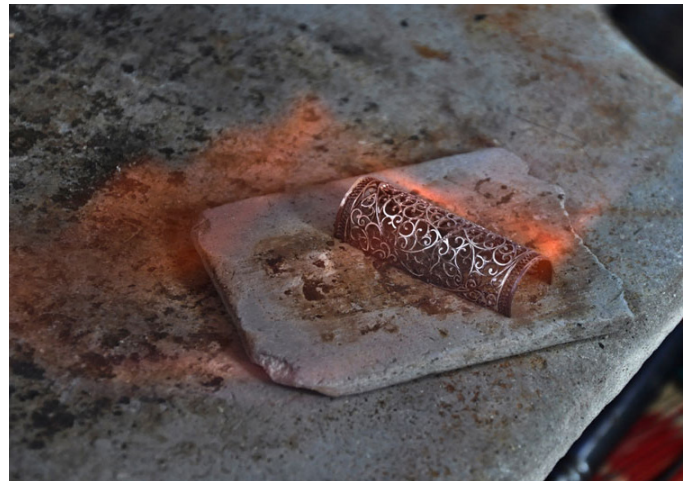
Silver is easily bended, when it is slightly heated.
