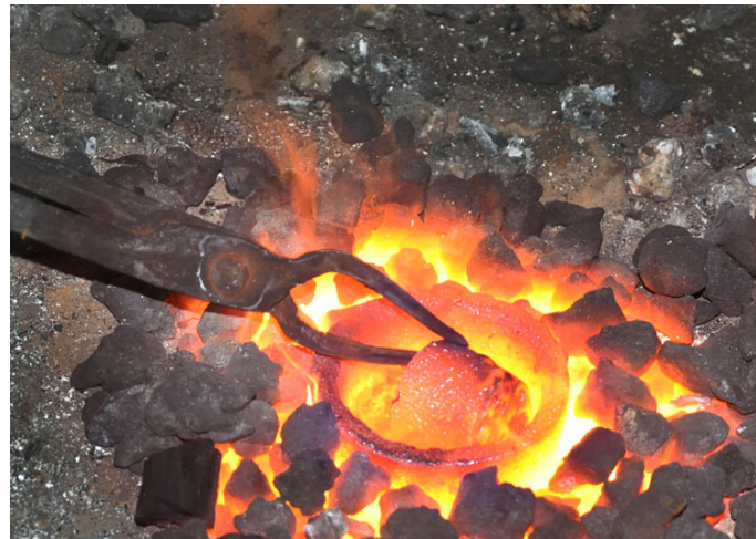
Melted silver is taken out using small crucible for the further process.
