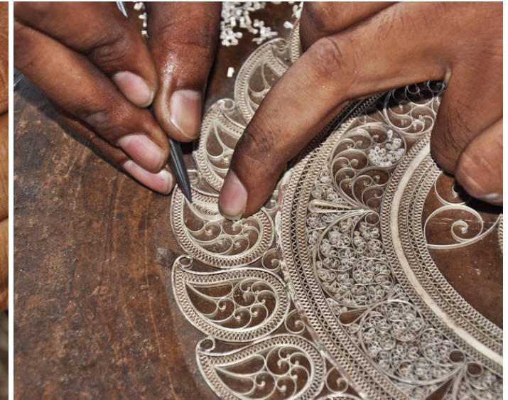
The coiled design is inserted to create mango motif.
