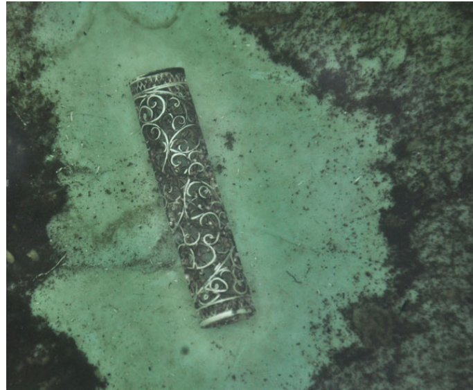
The product is dipped into the diluted sulphuric acid.
