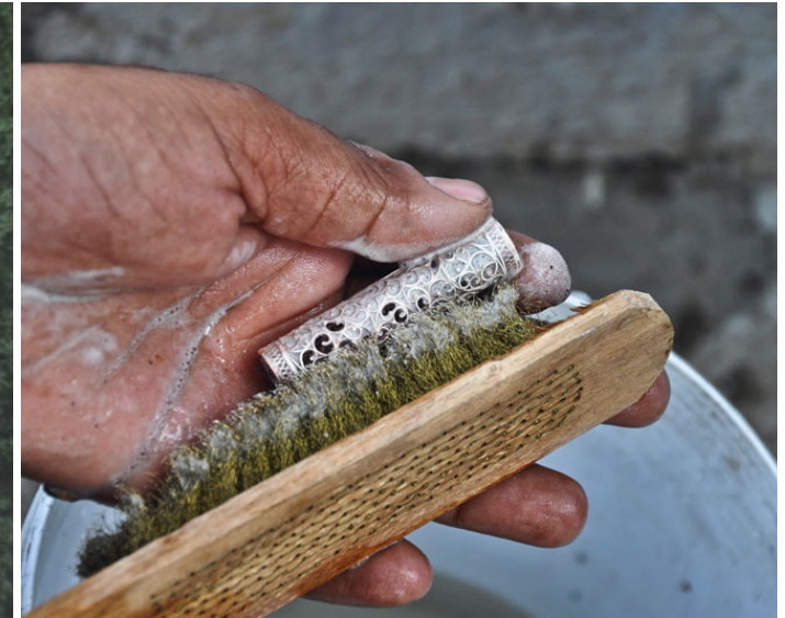
Using brass metal brush the product is polished for shining.
