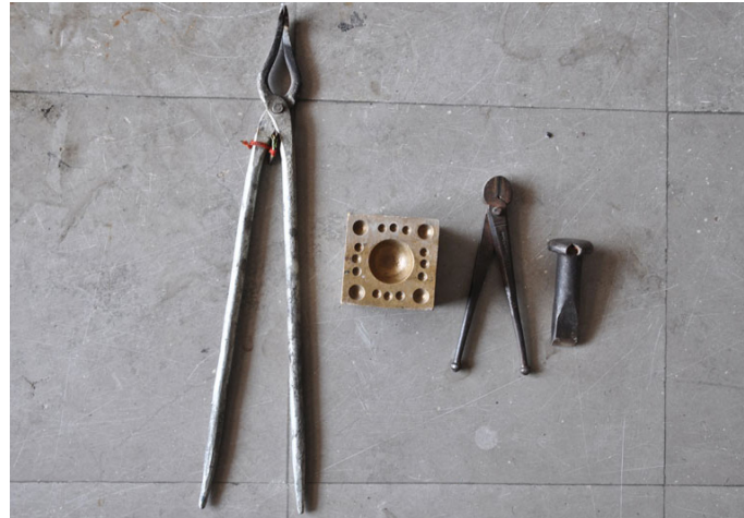
Geajaldhim (called locally) cubical shaped tool. It is used to make the sheets into curved shapes.
