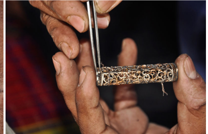
The edges are binded together using small silver beads.
