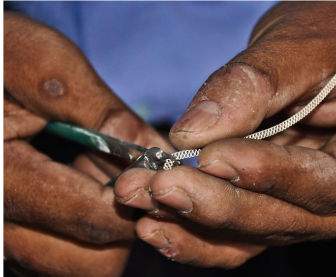
Early prepared spring is cut and fixed to the borders.
