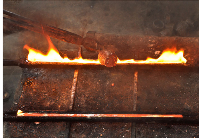
Melted silver liquid is being poured into the molds.
