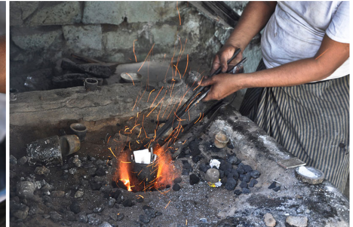
The biscuits are placed in a crucible and melted.
