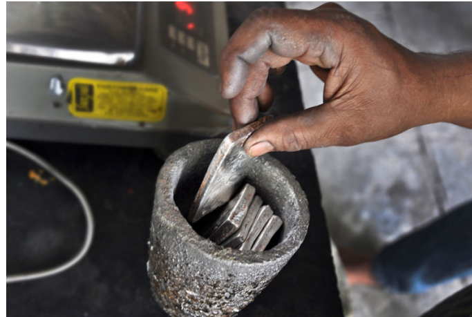
Silver biscuits used to create rods and different shapes.
