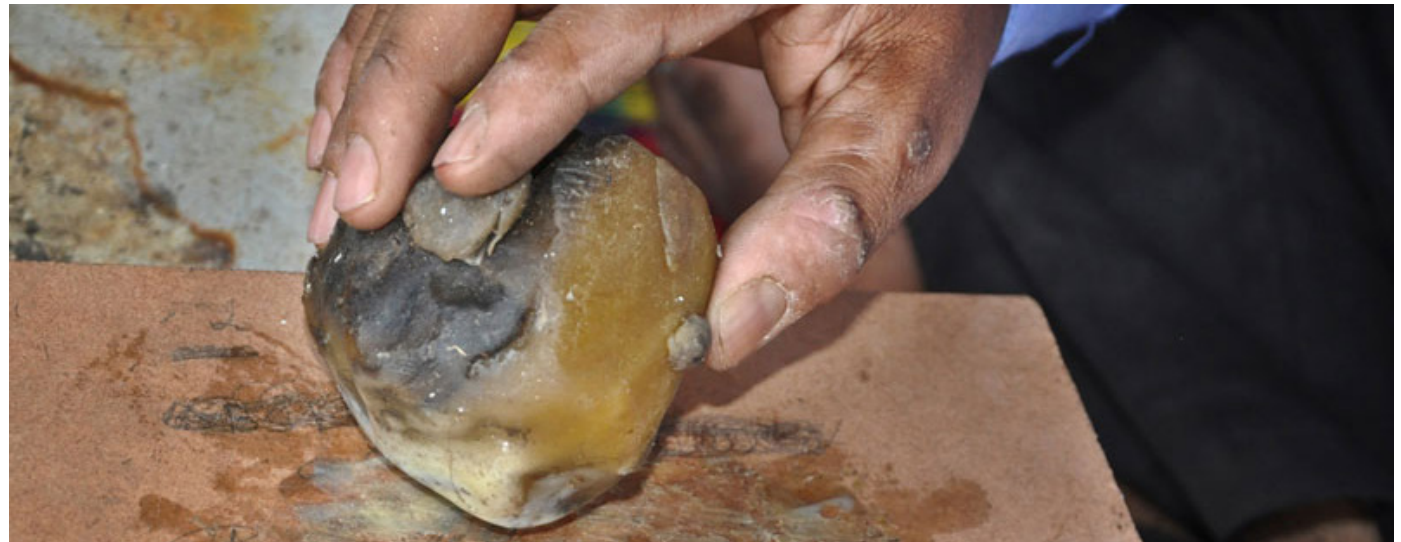
Wax is applied on the base where the product is to be made.
