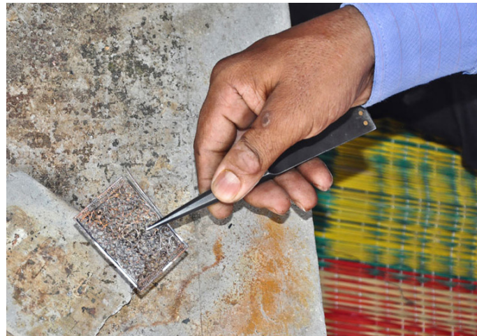
After heating, the jaali work is properly set in the frame.
