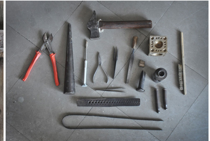
Variety of tools for twisting and cutting of the silver.
