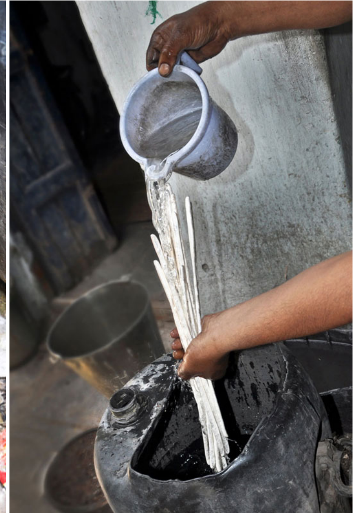
The silver rods are washed to remove the stains.
