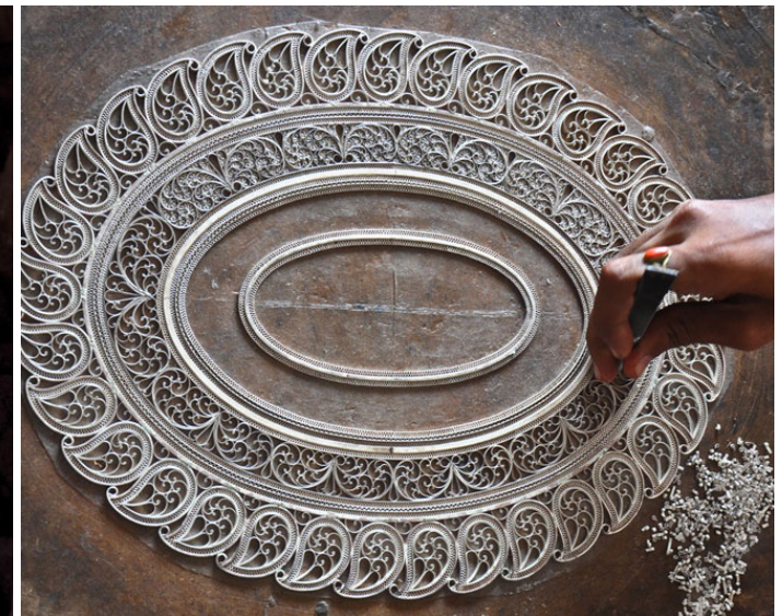
Small beads and grains made of silver are filled in the unique master piece.
