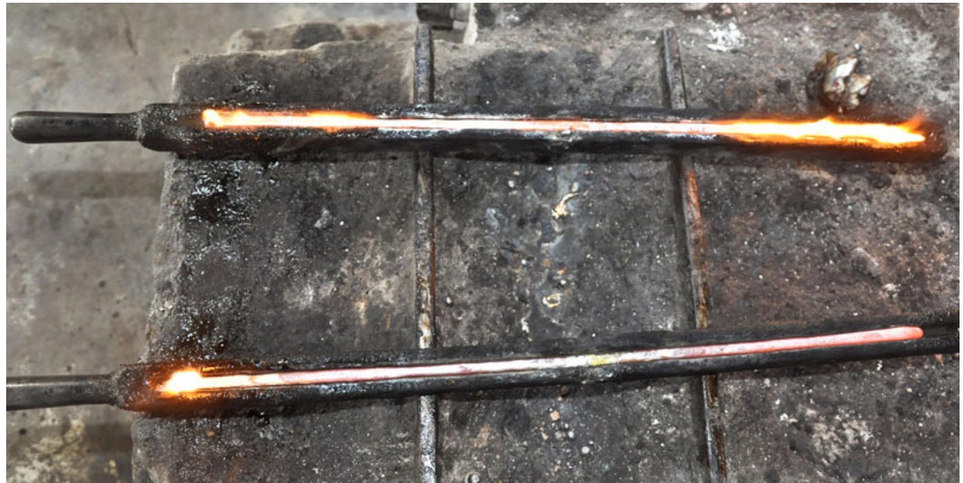
Moulds used to pour the melting liquid silver to make rods.
