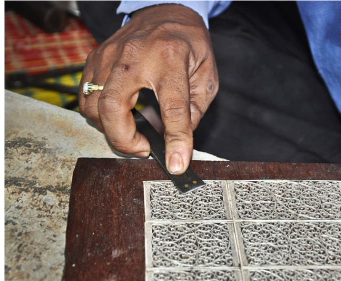
Flat edged tool is used to press on the designs to set the small beads stiffly.
