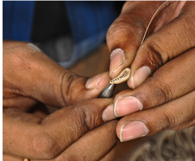
The silver is coiled and pressed to form leaf shape.
