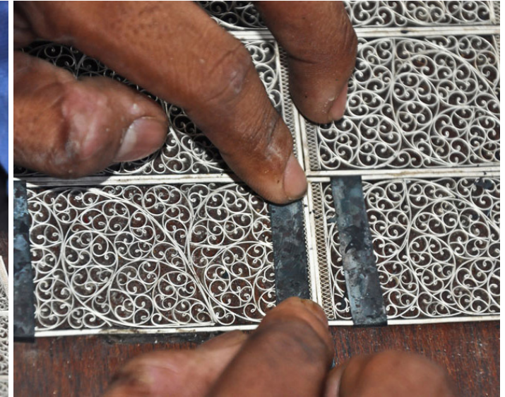
Metal sheet is tied to the frame for the better support.
