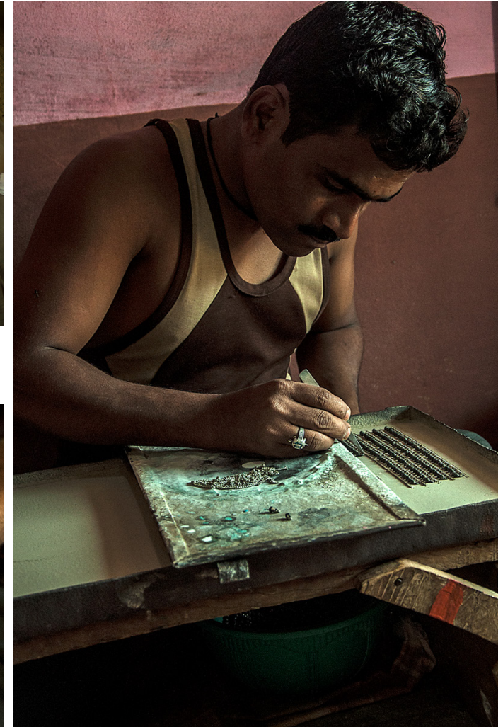
Pieces are arranged using a tweezers and this process is referred as the Chaadi process.
