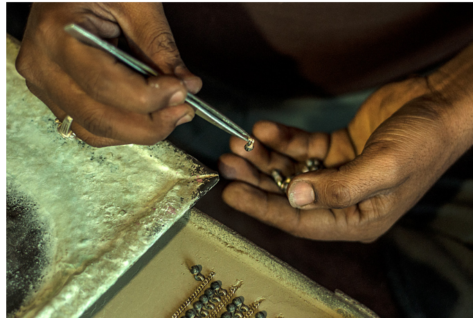
Silver beads and chain are arranged accordingly for soldering process.
