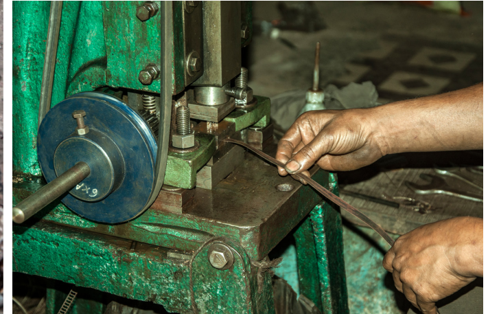
Using dye machine silver sheet is cut as per requirement.
