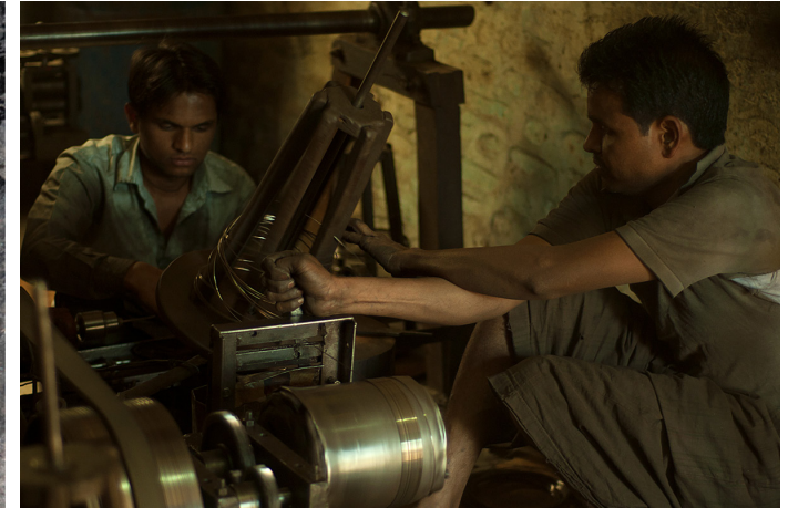
The silver rods are passed through rolling machine and converted into silver strips and wires.
