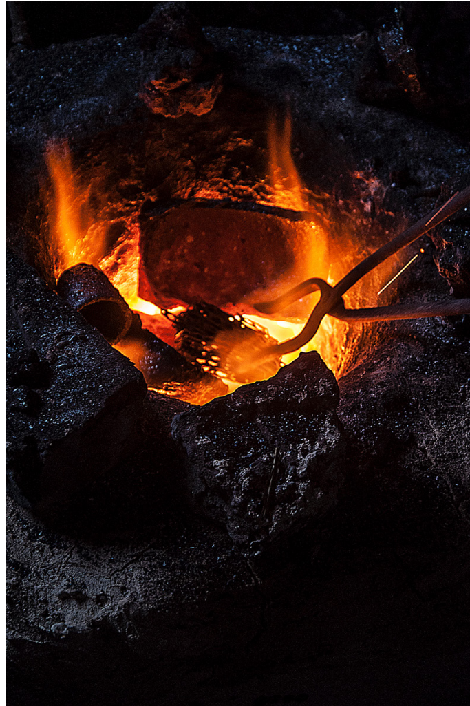
Silver biscuit and copper pieces are melted in crucible at high temperature.
