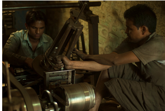
Silver rods are passed through the rolling machine and converted into wire.
