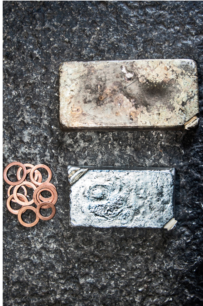
Gold and copper is added to silver as raw material to make silver anklet.
