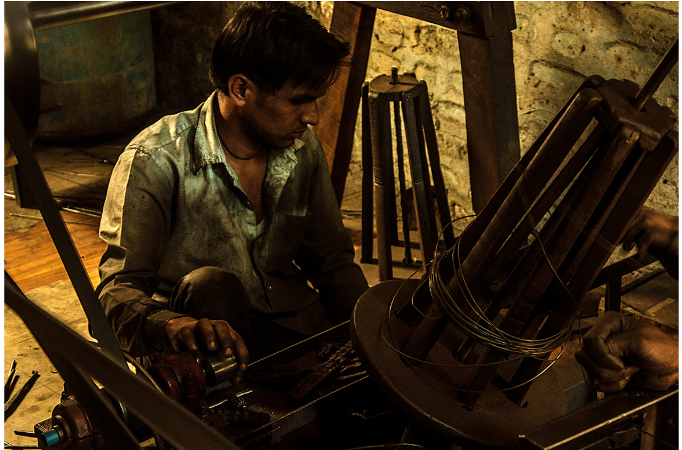
Rolling machine used to convert the silver rods into wires.
