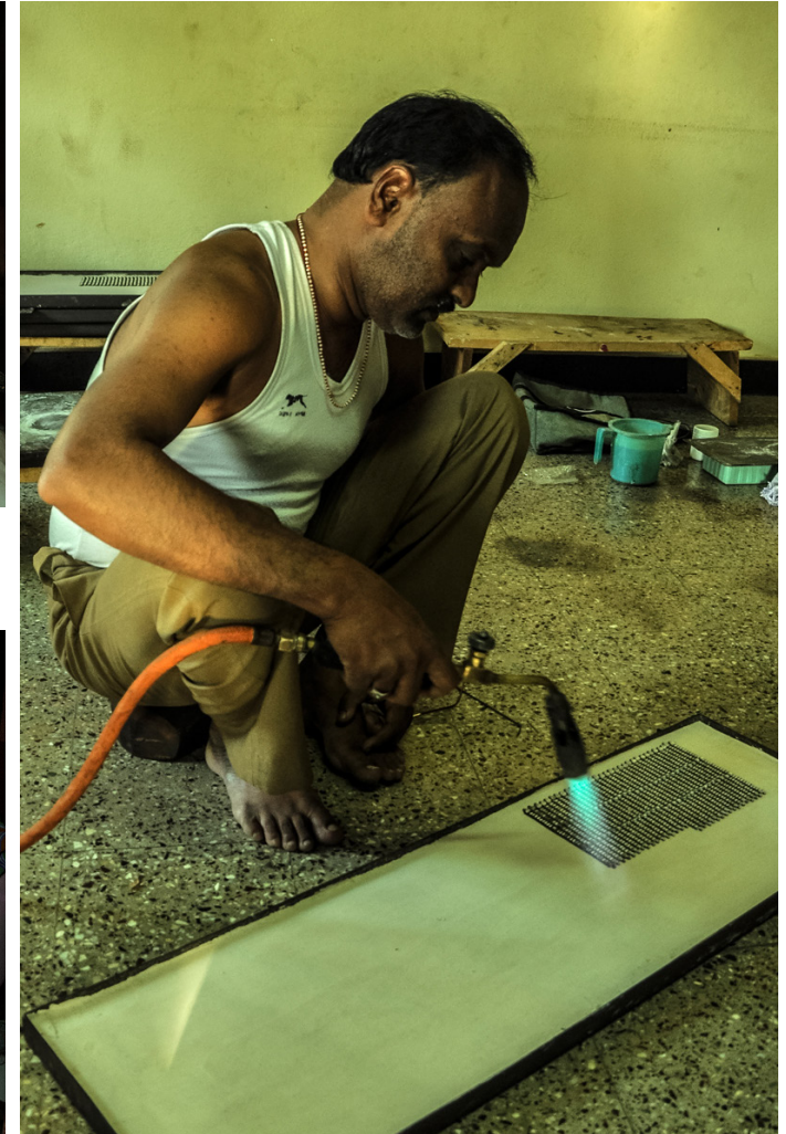
The arranged pieces are heated to solder using flame torch.
