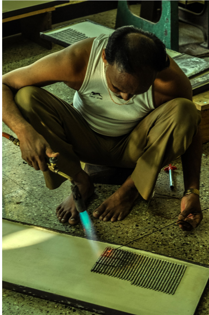
A metal wire is used as support to hold the pieces together.
