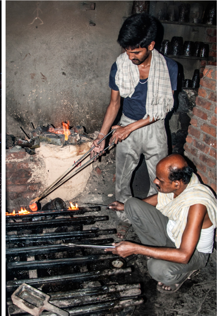
These iron molds are specially made for jewelry making process.
