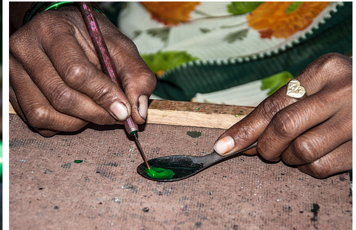
Meena color is mixed with hardener to stick to anklet.
