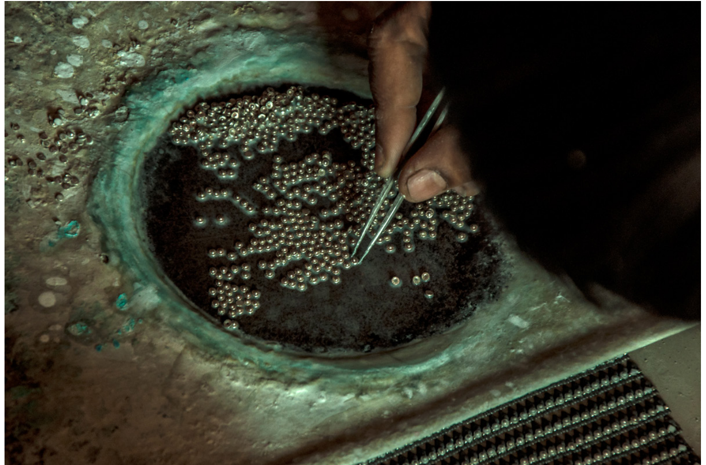
Design piece, which has to be placed on the chain, are soaked in soldering solution.
