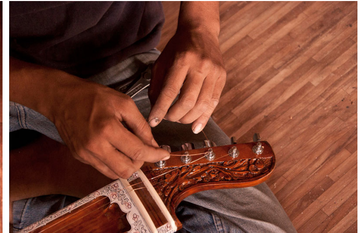
The strings are attached to the tuning pegs.
