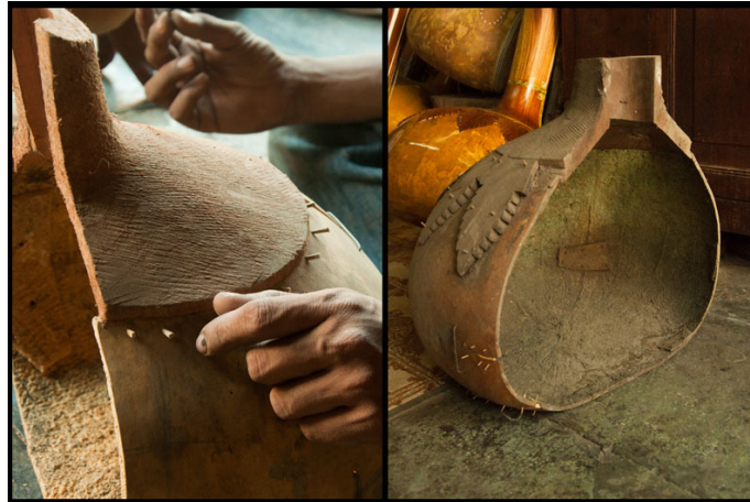
Dry gourd is cut to \frac{3}{4} size, to which wooden gulu (neck of resonator) is attached.
