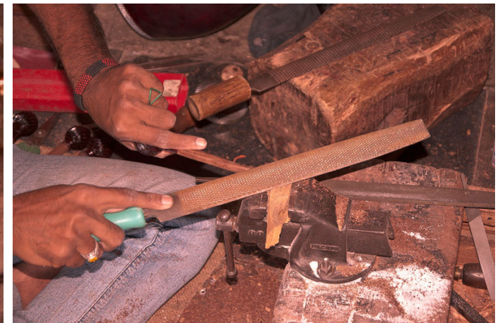
Pegs are made of rose wood and filed.
