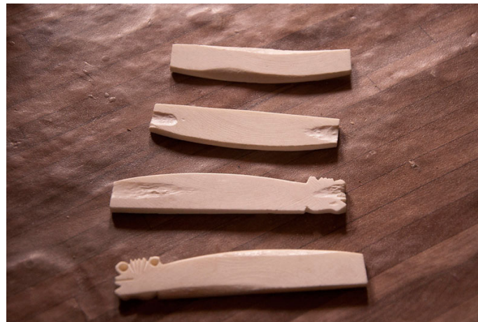
Camel bone or stag horn is used to make the bridge for strings.
