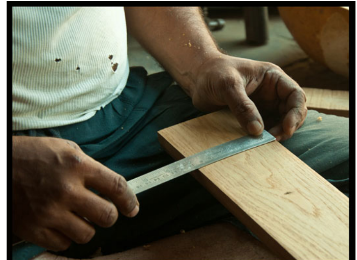
Long rectangular block is used to make neck of sitar.
