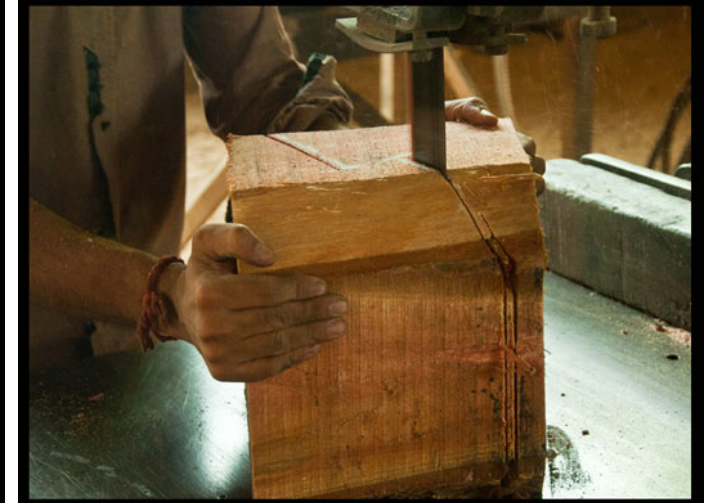
Blocks are cut according to the marking.
