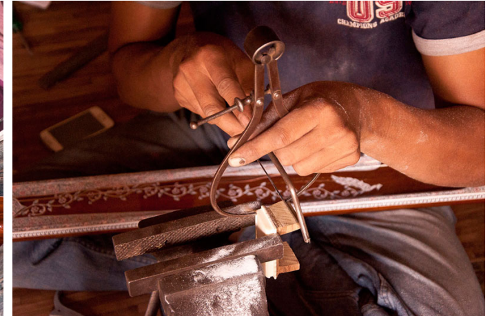
Divider is used to measure the main bridge height, which is made of stag horn or camel bone, which acts as a tonal enhancer.
