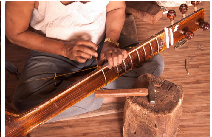
Frets are assembled with help of nylon threads (which are adjustable).
