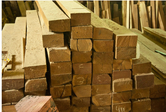
Long rectangular block is used to make neck of sitar.
