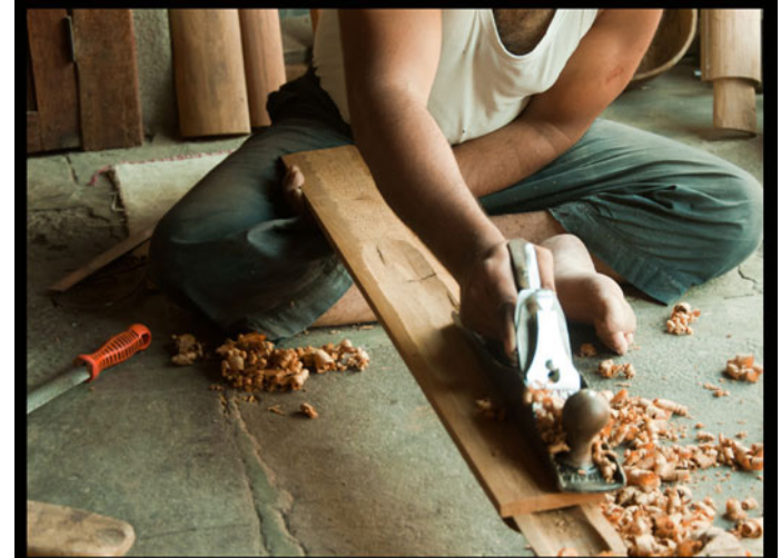
The excess wood is removed by measuring using wood scraper.
