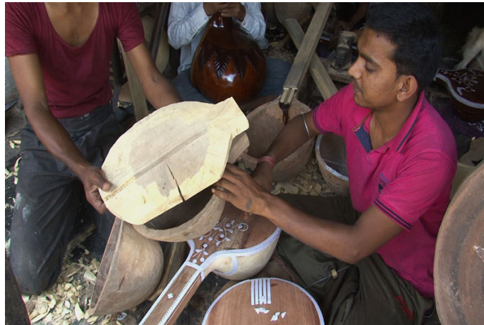
Resonator is covered with wood plate called tabli.
