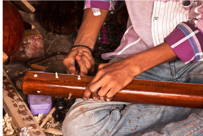
The peg is inserted at the end of the sitar on which the strings are wound.
