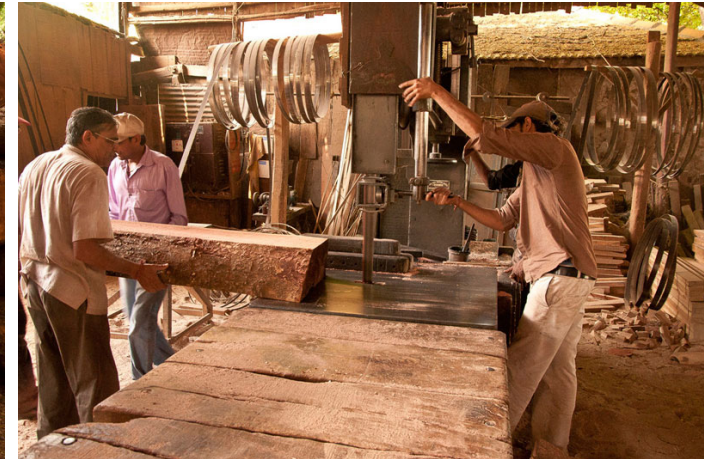
The log is cut into basic shape in saw mill.
