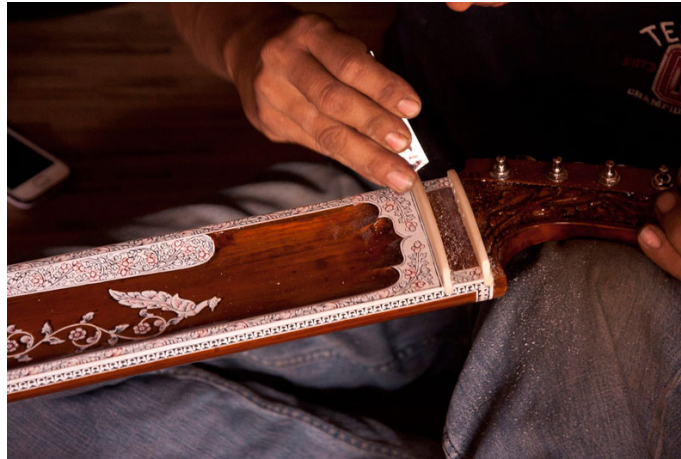
Two pieces of the bone is place parallel at the end of the finer board which are known as Parti and Ard-parti.
