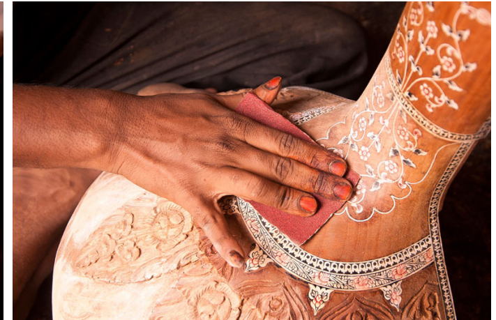
The sanding is done to remove the rough edges.
