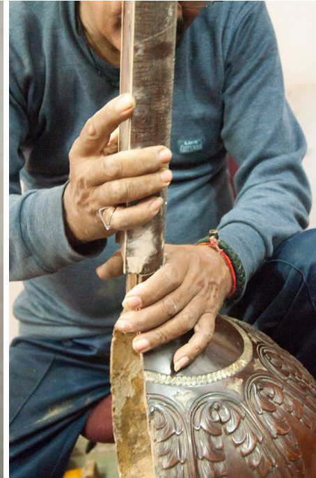
Wooden gulu (neck of resonator) is attached.
