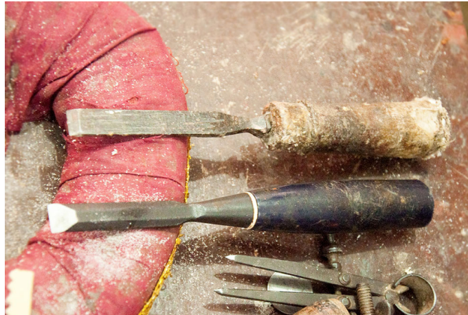
Chisel is used to carve the wood.
