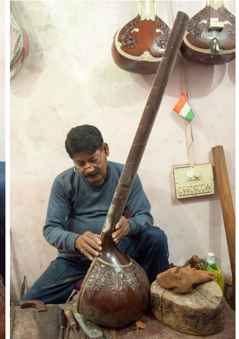
Artisan is checking the measurement of resonator cover called tabli.
