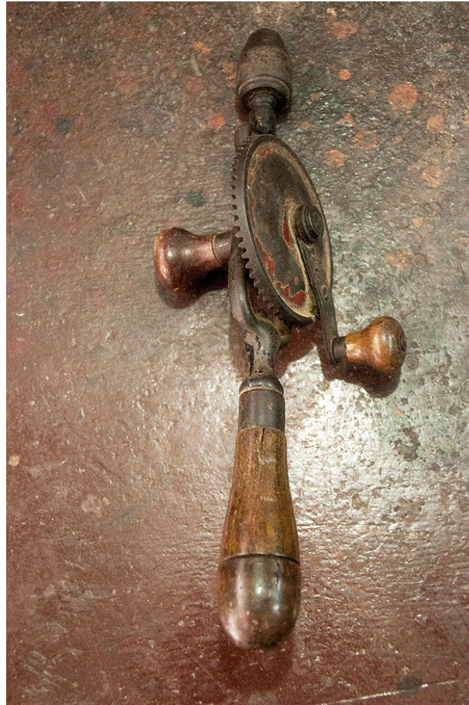
Hand drilling tools for making holes in wood.
