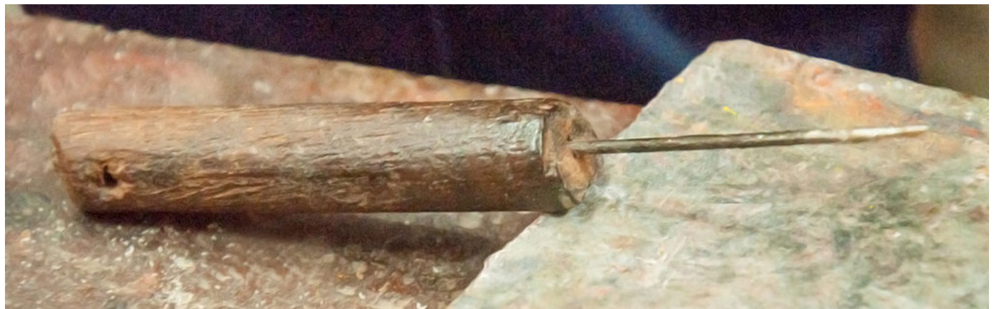
AWL tools used for marking and making holes in wood.
