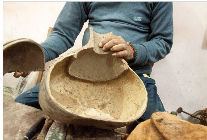
Wooden gulu (neck of resonator) is attached.
