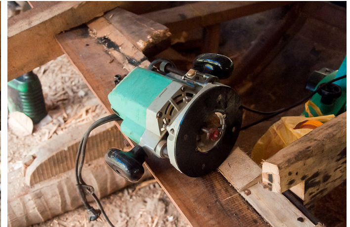
A Wood Router is used to shape the edges of the surface.
