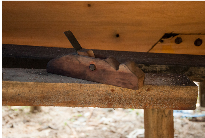
A Block Plane, which is used to trim the unwanted layers of the wood.
