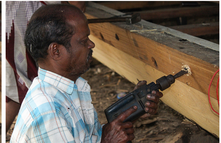
Artisan is drilling an in-depth hole on boat to fasten wooden plank with iron nail.
