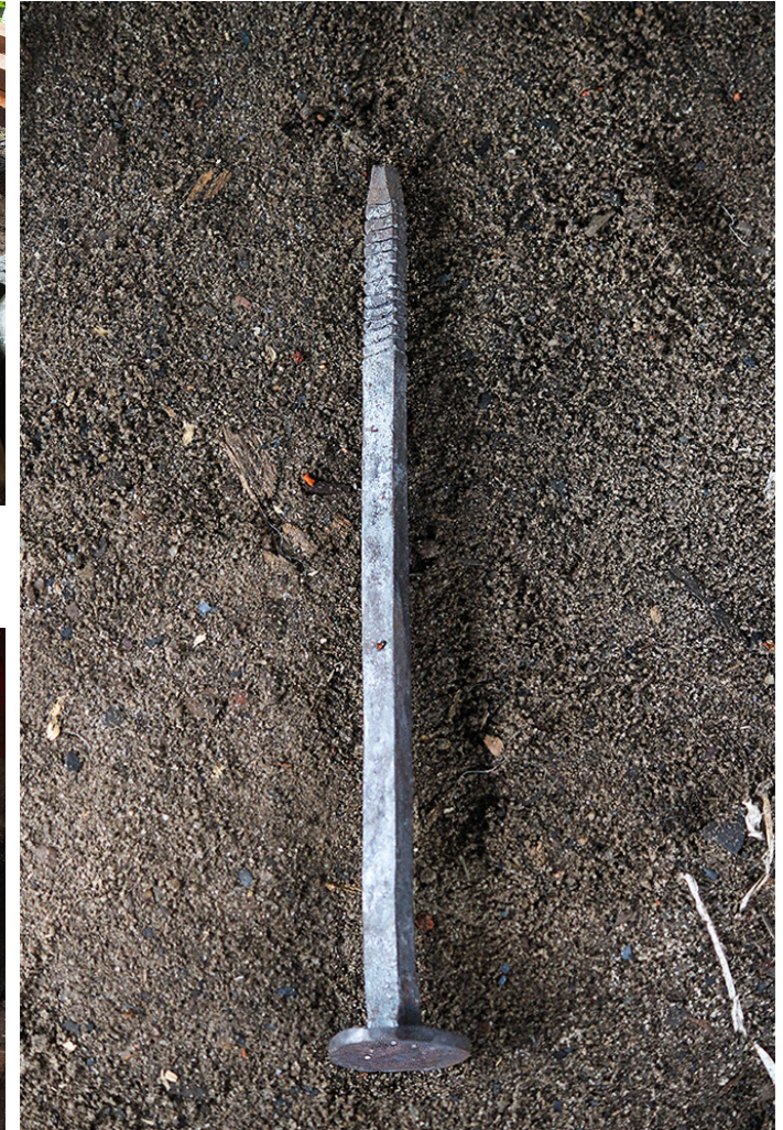
A big sized iron nail to give a strong hold on the wood.
