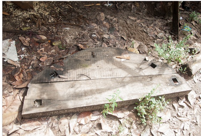
The reference frame that is made out of wood decides the shape and size of the boat.
