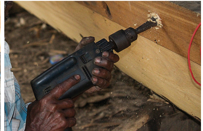
A Drilling machine is used to drill the holes on the wood in required shapes and depth.
