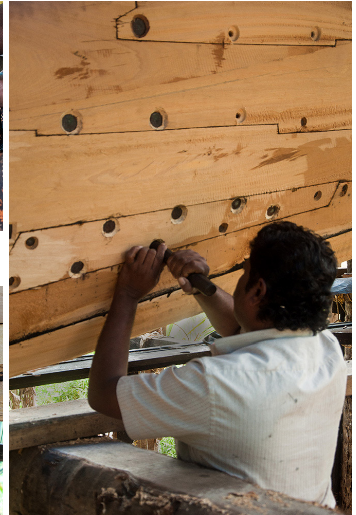
Artisan is hammering the iron nail to the boat without damaging the wood.
