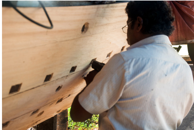
Artisan is hammering the rectangle headed nail to fit into the slot and give a strong hold.
