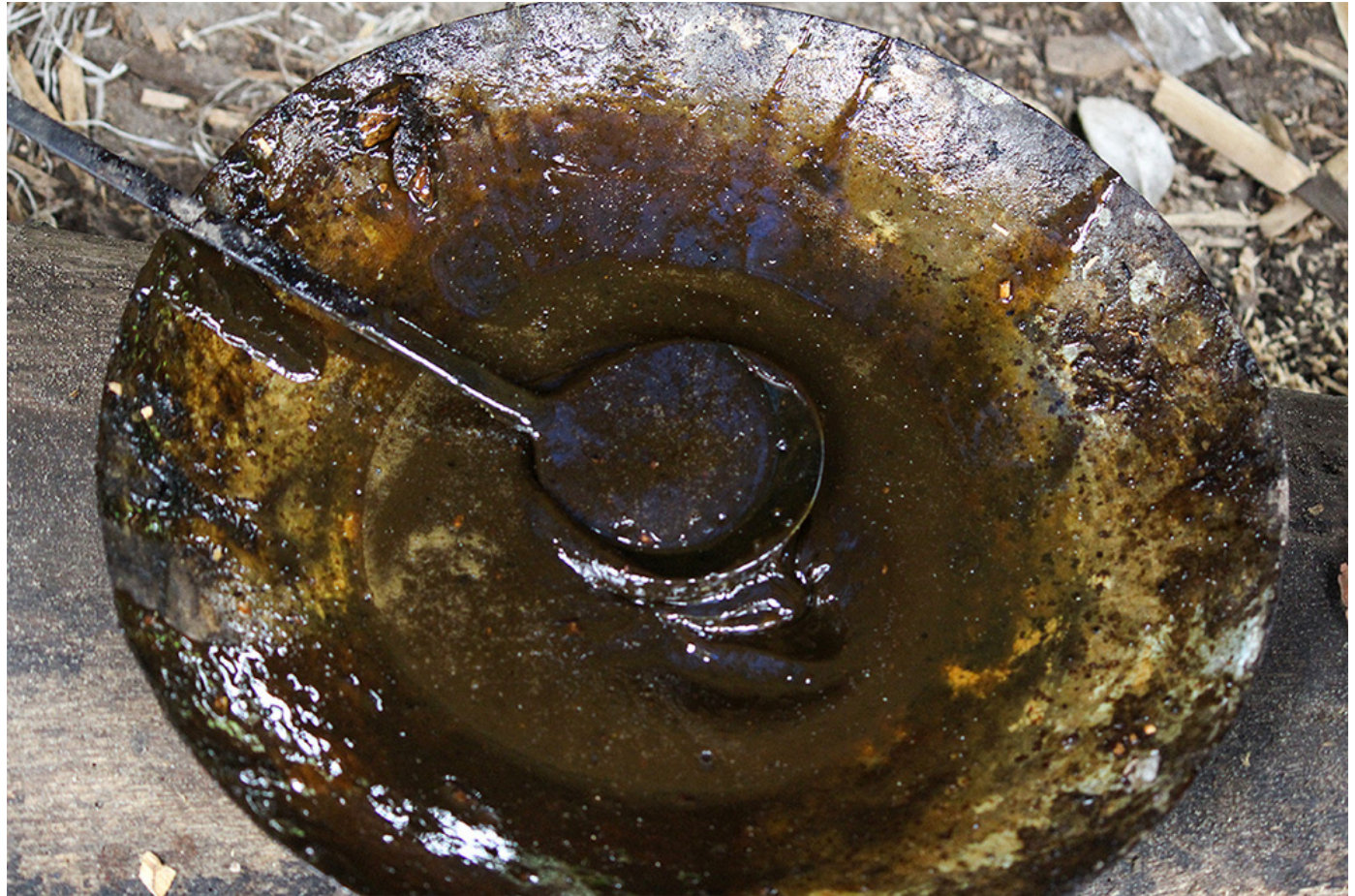
Glue made from wooden wax, cotton and coconut oil to fix the joint of two pieces.
