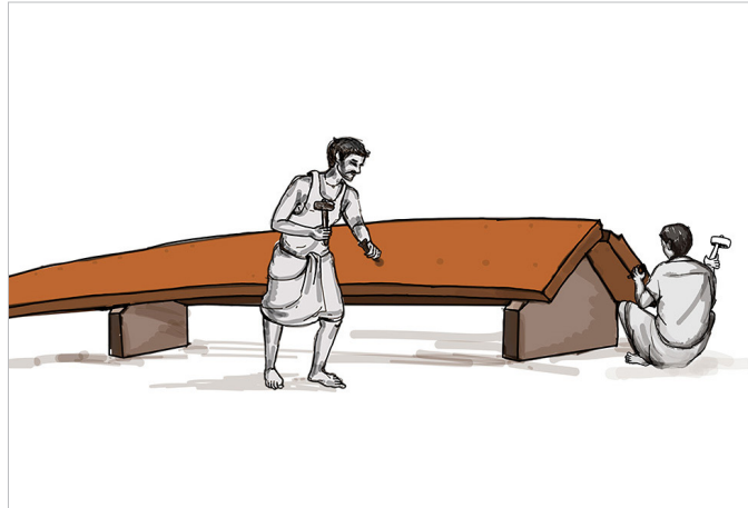
The side and bottom pieces are fixed together using customized iron nails.
