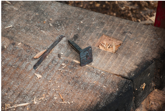
A rectangle head iron nail to fit in the boat according to the connected layers.
