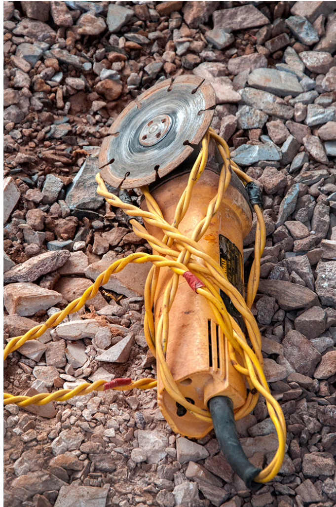
Electric cutting machine to cut the stone and ease the process of carving.
