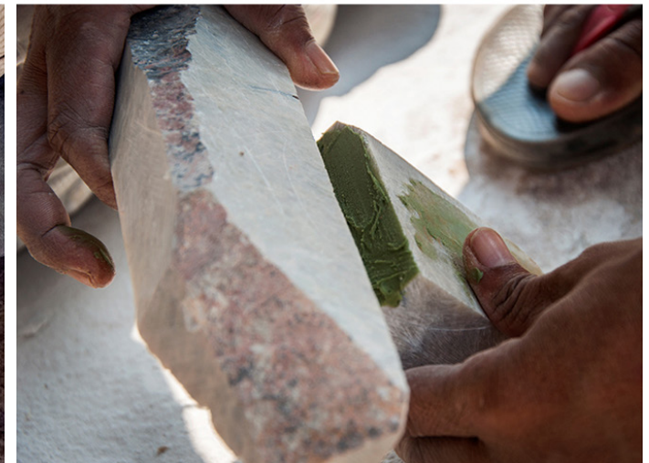
Applying metal patching paste on broken pieces of stone to stick together.
