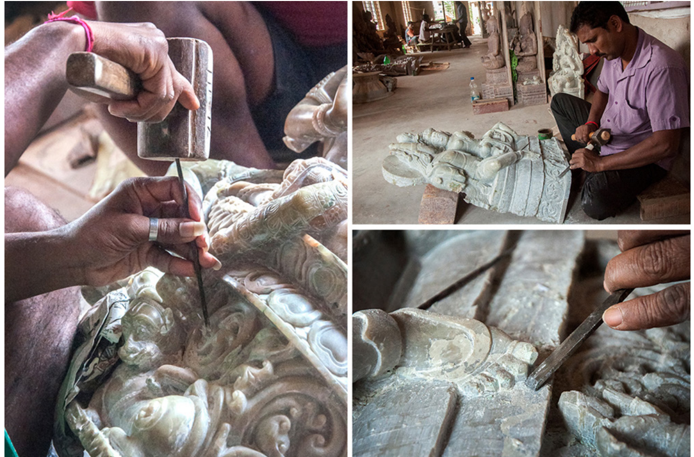
Fine details are created using flat chisels and hammers of various size.
