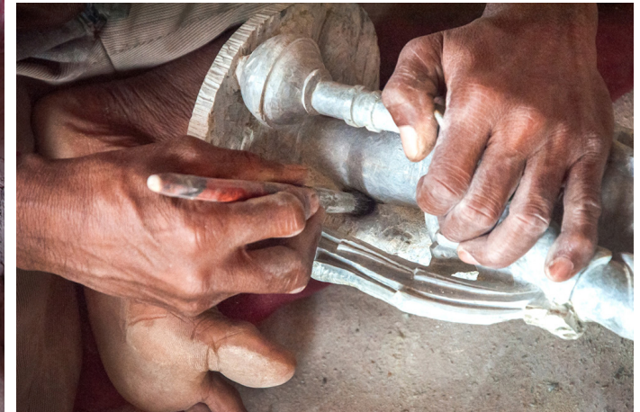
The excess of dust after carving is removed with a help of brush.
