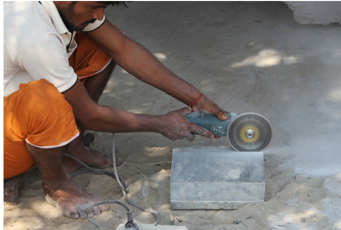
Automated cutting tool used to cut the granite stone evenly.
