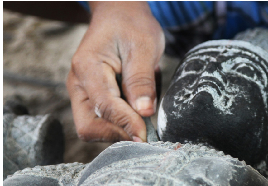
Sand stone is rubbed on the surface of idol to obtain smooth surface.
