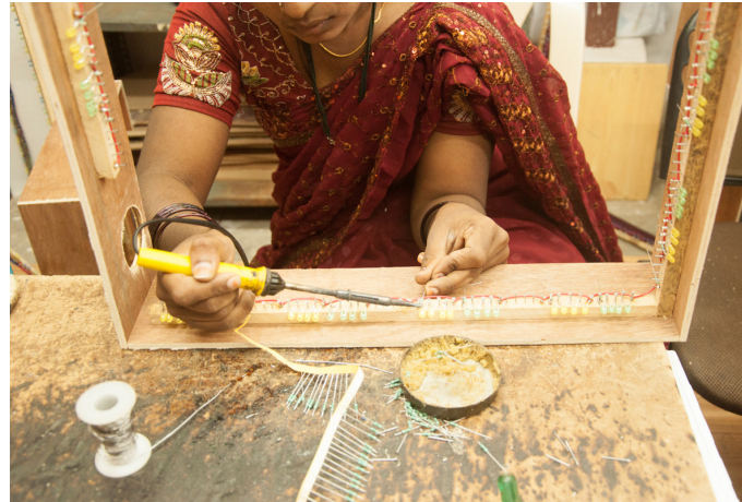
Artisan is fixing the serial lights into the frame.
