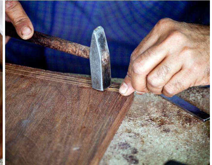
The metal wire is inlayed into the grooves with the help of gentle hammering.
