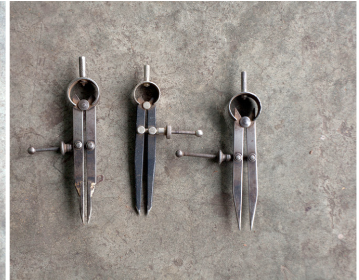
Compass is used for marking while cutting or drawing on the wood or metal
