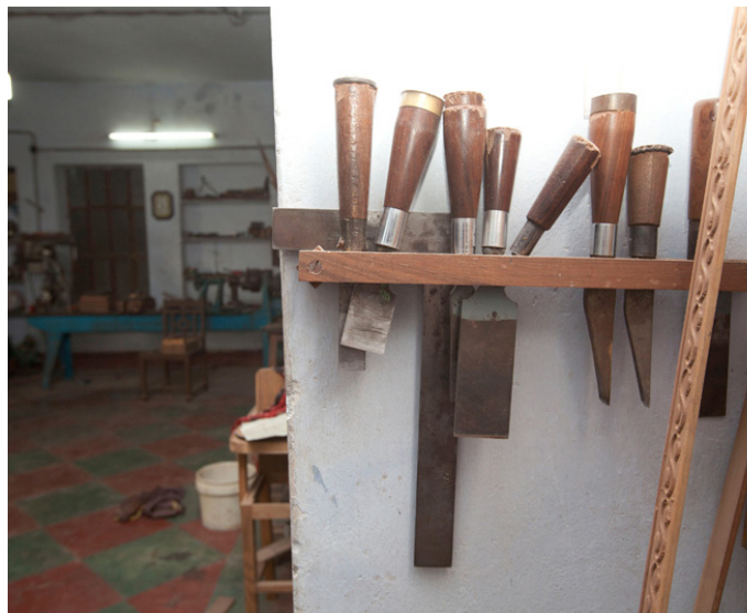
Big chisels for cutting and shaping the wood
