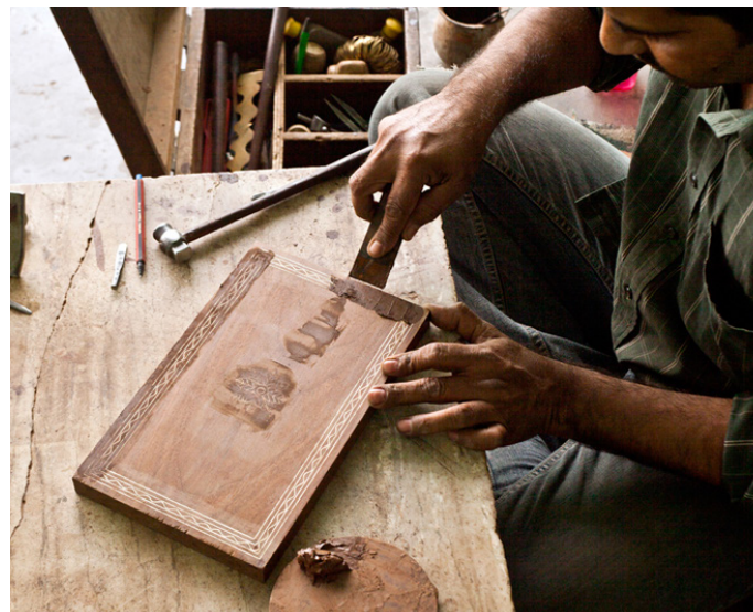
A paste of saw dust mixed with Fevicol is applied on the surface to fill the cracks and gaps.
