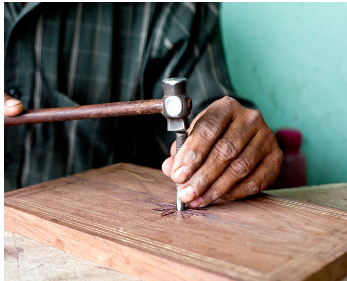
The circular grooves are made using half round chisel.
