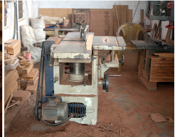
Machine used for cutting and planing the wood.
