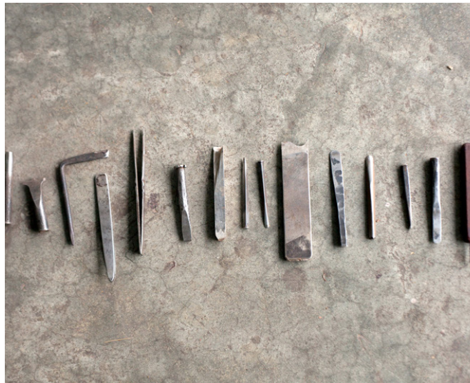
Various small chisels, forceps, awl etc. are used in Taarkashi works
