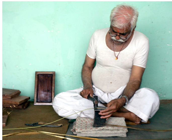
Shri. Hari Shanker ji making wires to be inlayed in the wood
