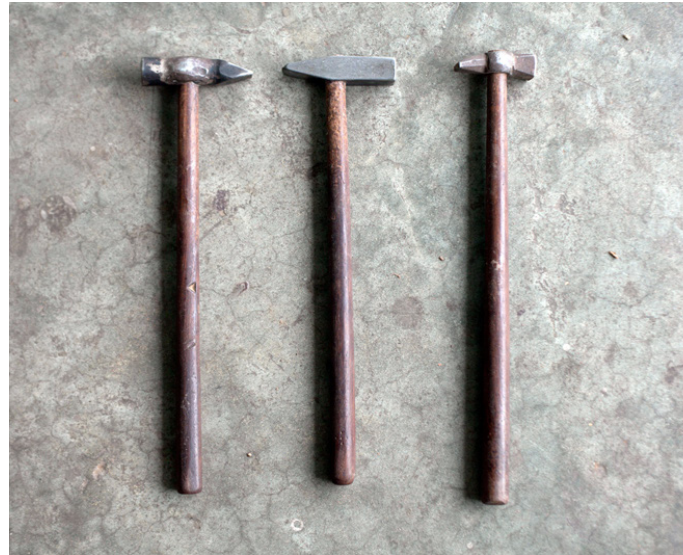
Hammers with small heads make it easy to beat on thin wires.
