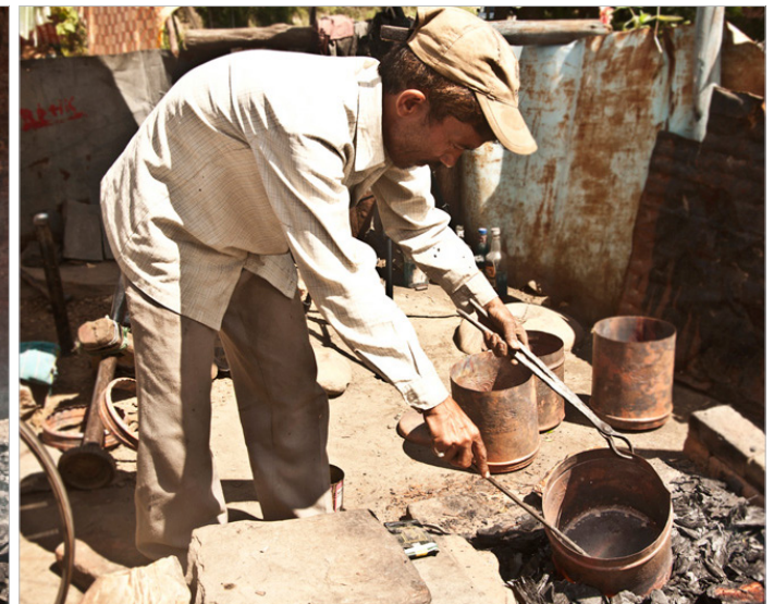
Object is rotated with the help of metal rods while heating.
