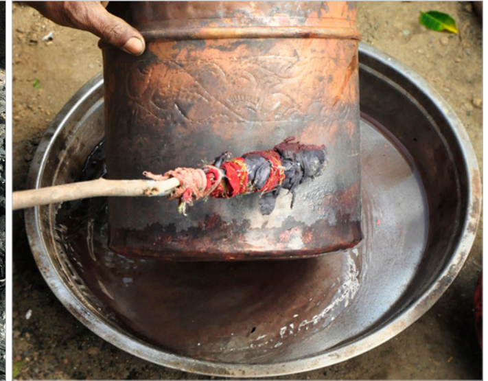
The finished product is washed with acid to get lustrous copper color.
