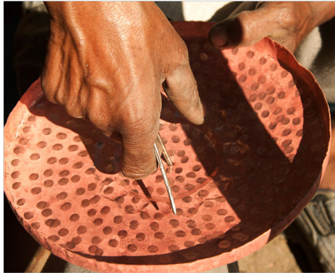
Lid of water container is pierced with sharp tool to create cavity.
