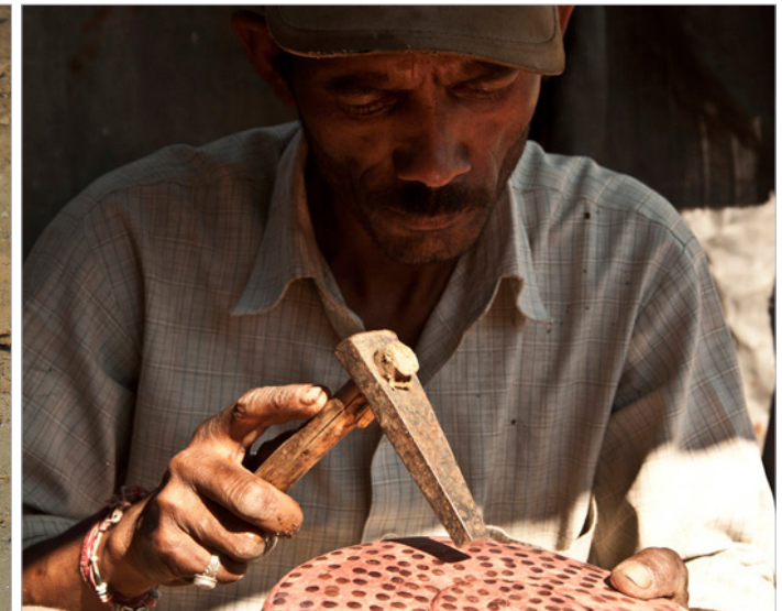
Beating the copper sheet makes it smooth, strong and sturdy.
