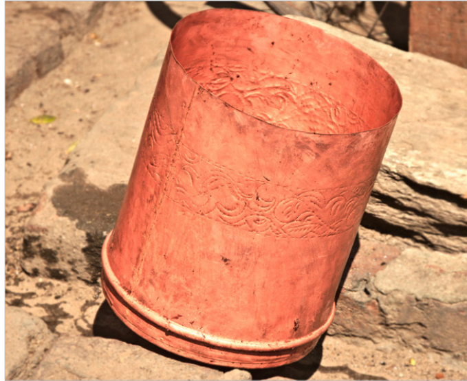
The product is coated with tamarind pulp and allowed to dry.
