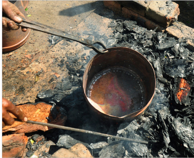
The base of the copper is soldered by heating.
