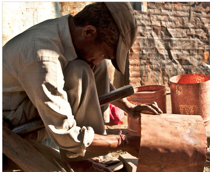
Sheet is bent to make cylindrical shaped container.
