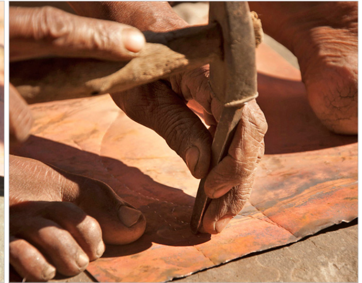
Motif designs are engraved on the surface of sheet.
