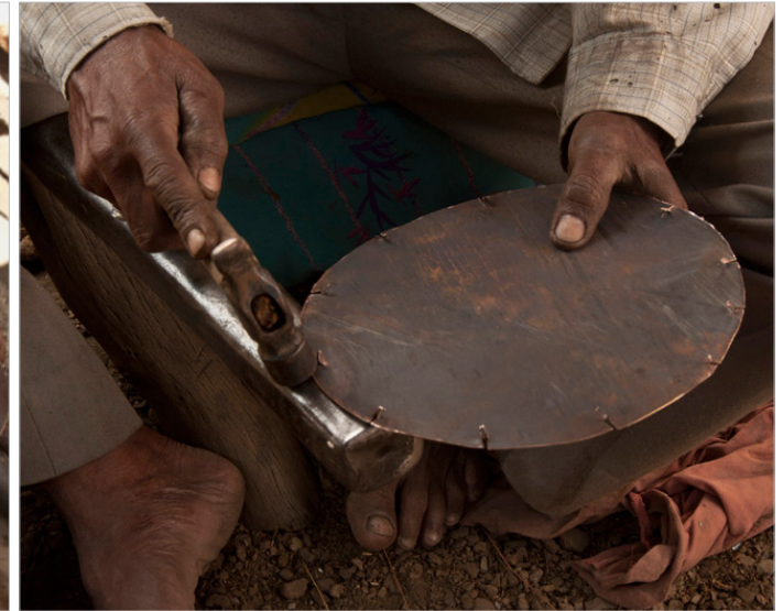
Copper plate is beaten to make flat.
