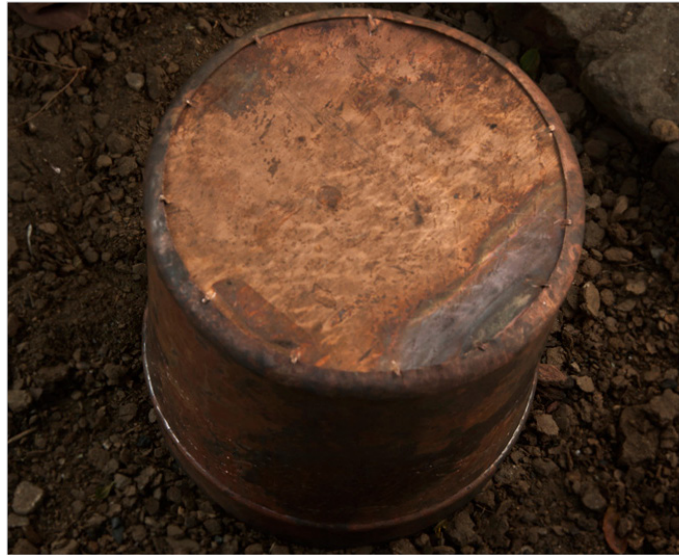
Nails are used to fix the base plate with border of container (the rounded container body).
