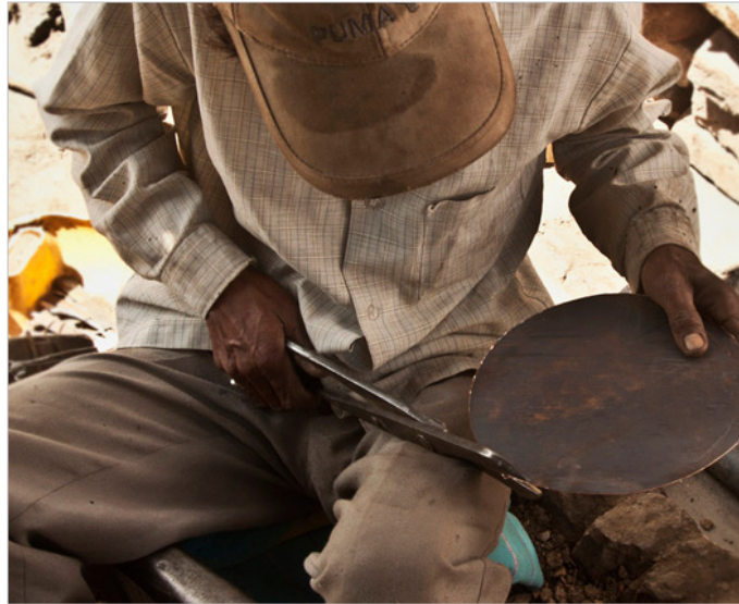
Sheet is cut in circular shape to fix it with container.
