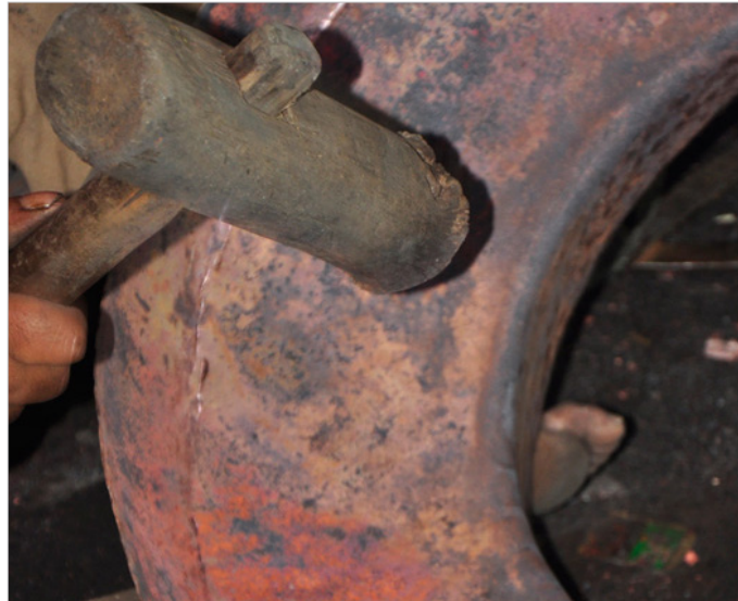
The base of pitcher is beaten by wooden mallet.
