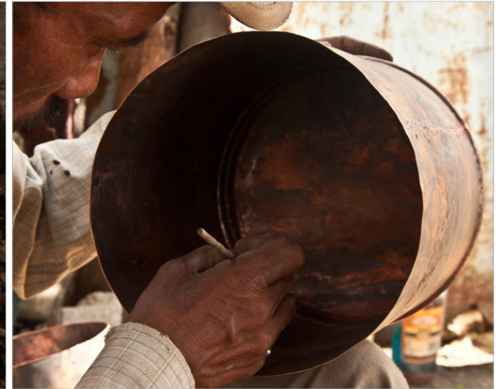
Artisan applying paste made of metal powders to seal the gaps, which helps to avoid leakage of water.
