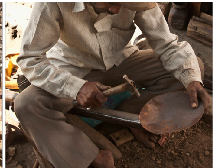
Base part is made using thick sheet of copper.
