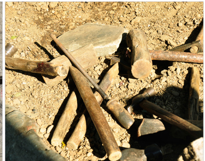
Varieties of Hammer are used until the copper takes desired shape.
