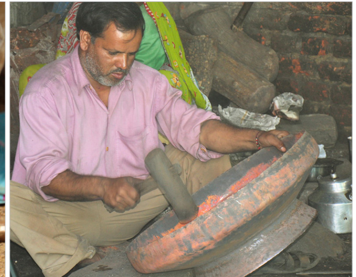
Artisan shaping the copper sheet to make to part of a container.
