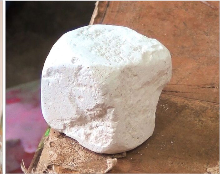
Limestone is used to apply completely on the wooden board before artisan starts to paint.
