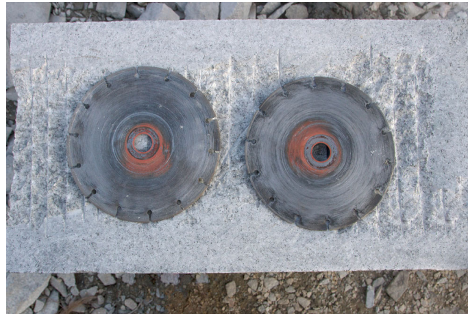
Diamond blades are fixed in the machine to cut the stone.
