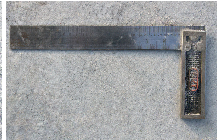
L shape ruler is used to measure the stone to a required length and cut.
