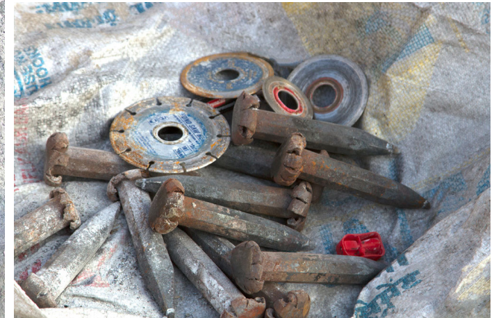
Different sizes of chisels are used according to the shape and thickness of the design.
