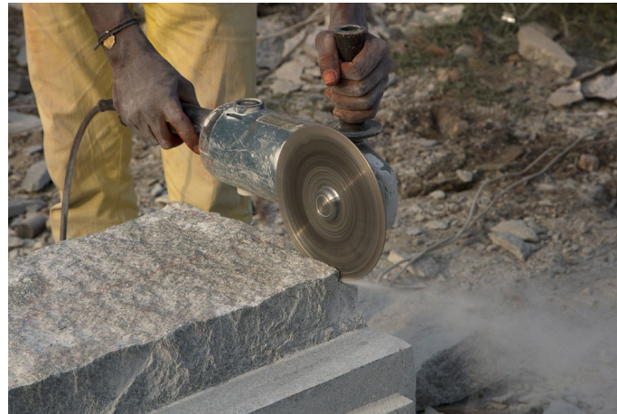
Using an electric stone cutter excess part of the stone is removed.
