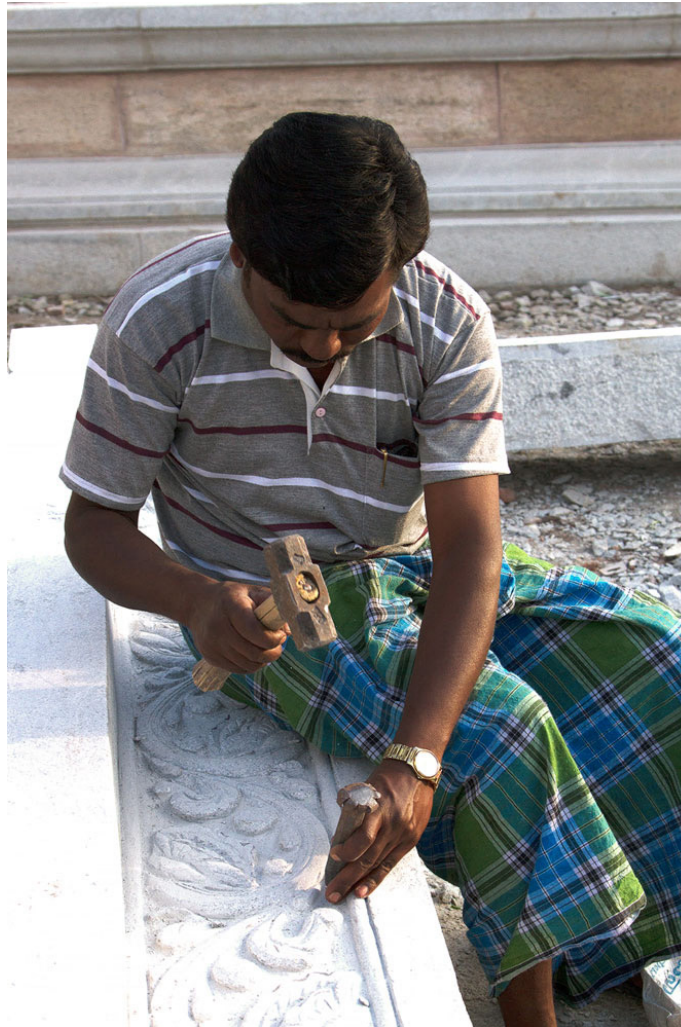
Big and small chisels are used for carving the respective design pattern.
