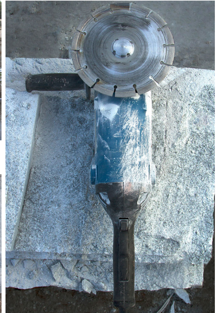
Electric stone cutter is used to cut the stone to the necessary length and shape.
