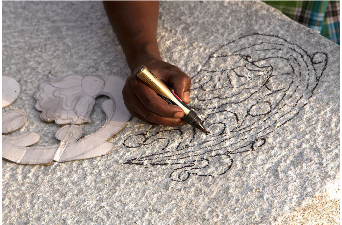
The design is outlined using a marker for better visibility while carving.
