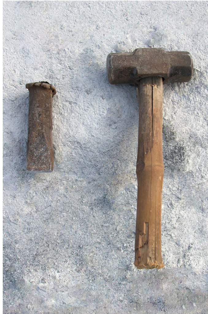
Hammer and chisel is used to carve out the design on the stone.
