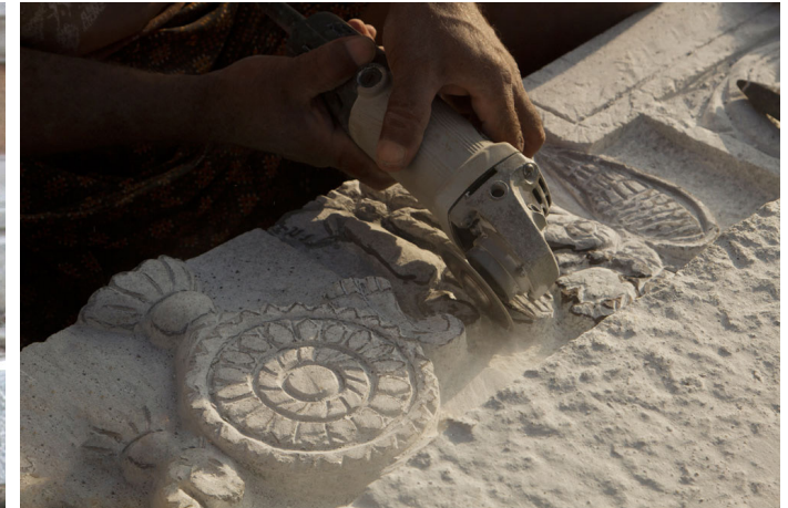
With the help of stone cutter carved edges of the design are leveled and smoothed.
