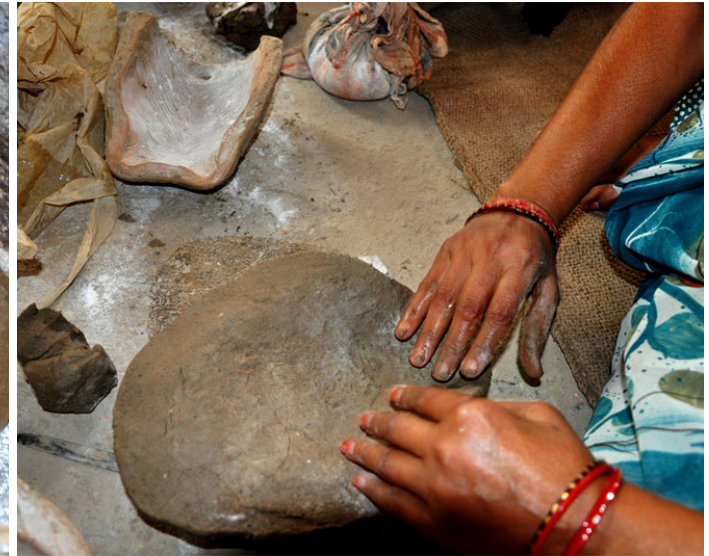
Clay slab is placed into the mould.
