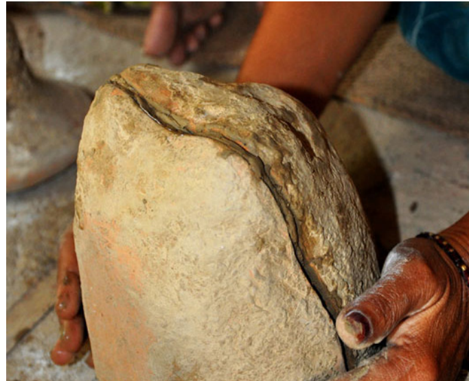
Joining the clay filled moulds.
