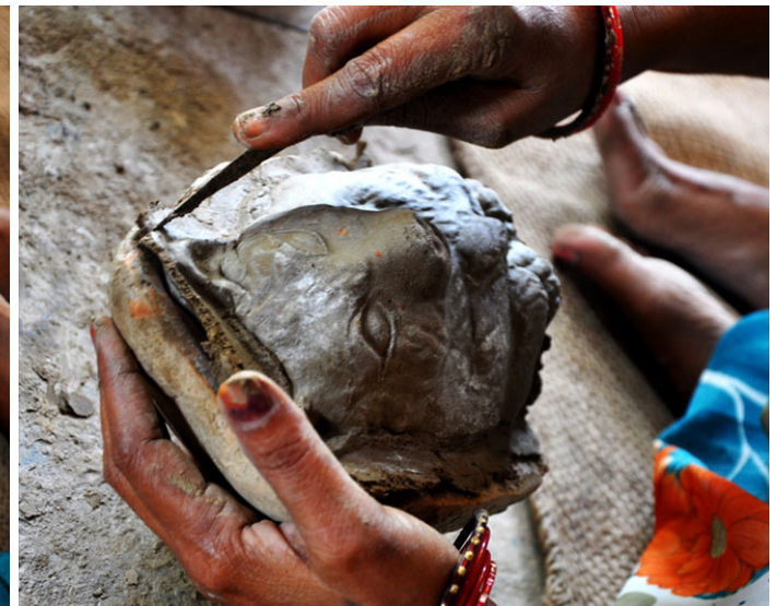
Corners are trimmed with an iron blade.
