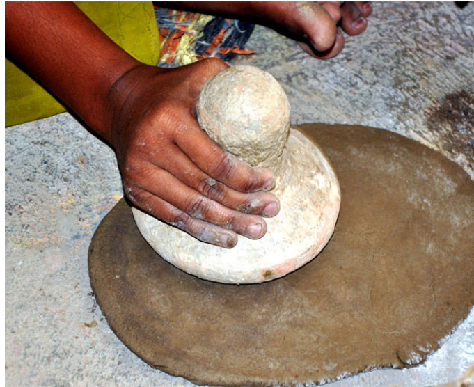
Flattening the clay to make the surface even.
