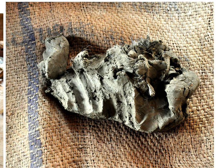
Kaali mitti -black soil used to make the clay products.
