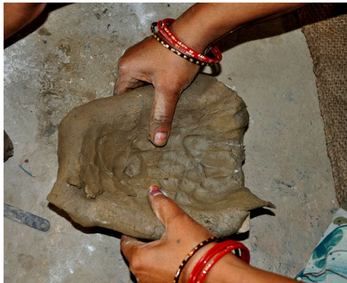
Then clay is pressed to take proper shape of mould.
