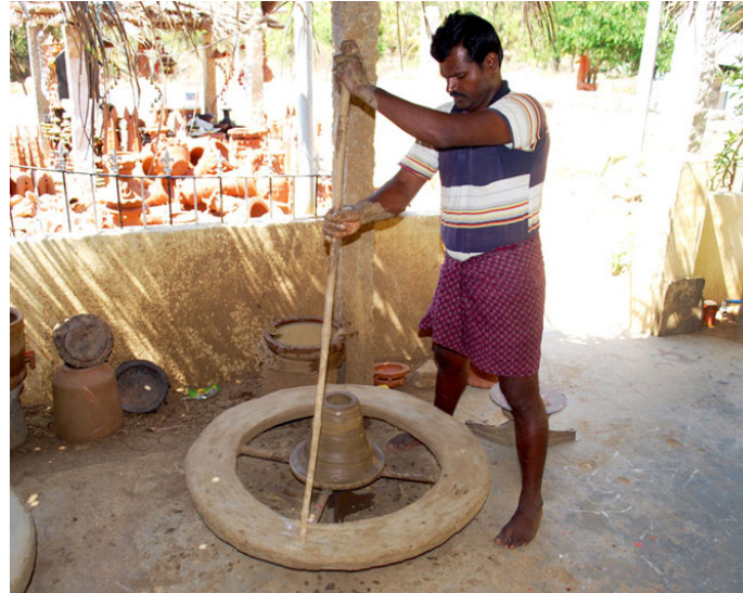
Veduru karra-bamboo stick used to rotate the wheel.
