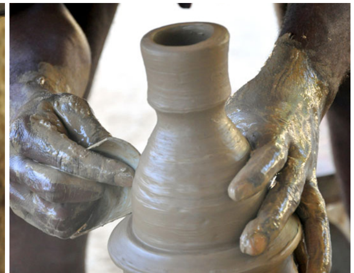
The outer surface is textured while the wheel is in motion.
