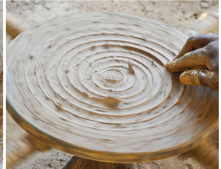
The mud is applied on the center of wheel which acts as an adhesive.
