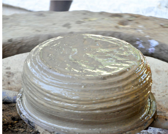
Water is applied before starting the shaping process.
