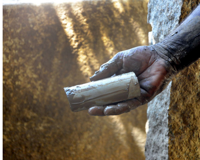
Semicircular piece of plastic used for texturing the surface of the object.
