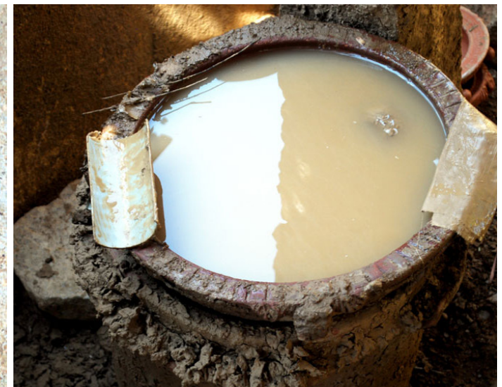
Wet cotton cloth is used to smoothen the surface of the object.
