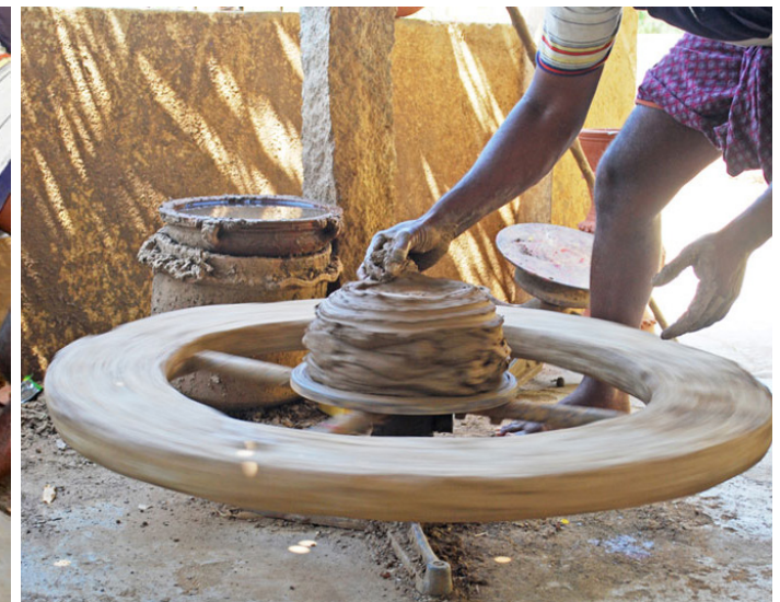
As the wheel rotates, the excess clay is removed.
