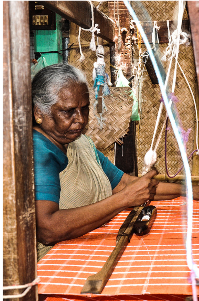
Experience artisan checks the smooth flow of fly-shuttle.
