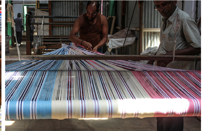
Segregating the different colored threads for continue the weaving process.
