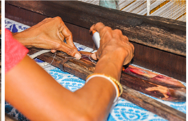
Artisan inserting the spindle to fly-shuttle.
