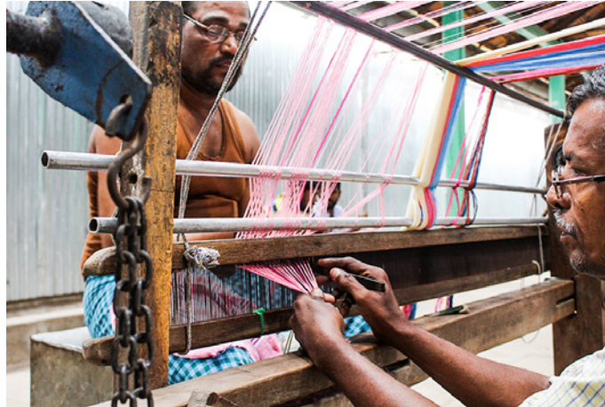
Arranging the threads to handloom.
