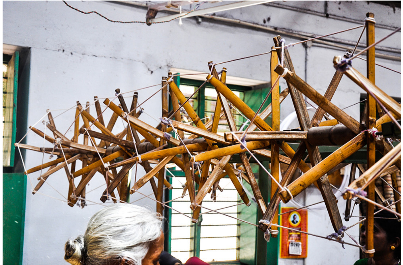
Artisan segregating the yarns for taking thread.
