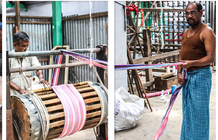
Combining the different colored threads to handloom beam.
