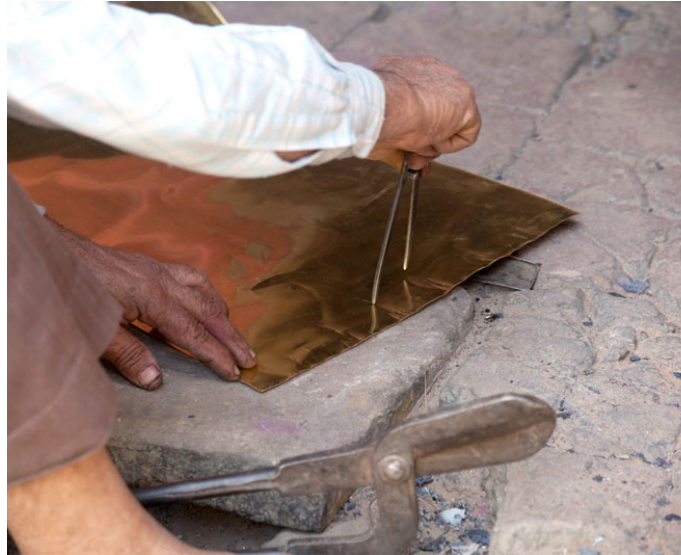
Sheet is marked as per the required shape/form.
