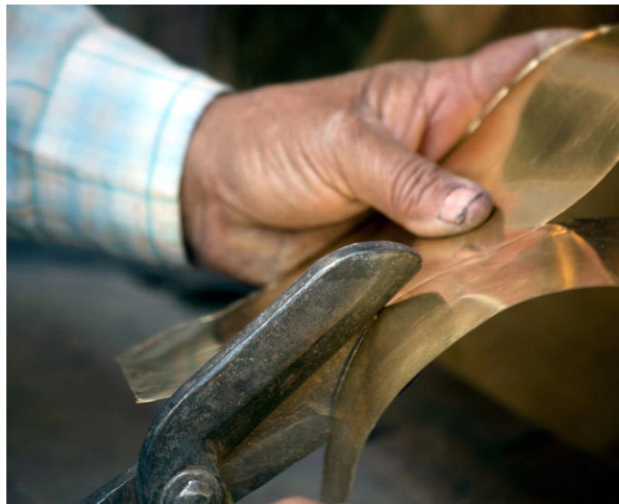
The metal sheet is being cut with the help of metal scissor.
