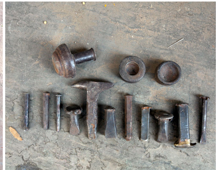
Cheni (Chisel) - Different shapes of chisels.
