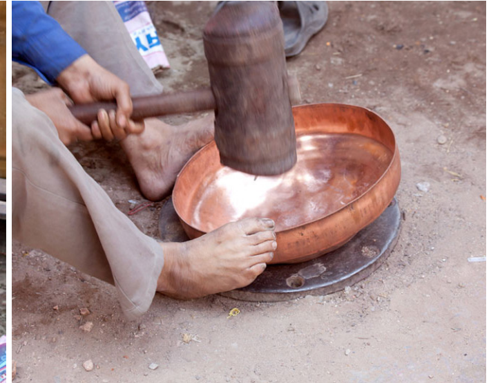
Concurrent use of legs and hands is done while hammering the metal product-in-process.
