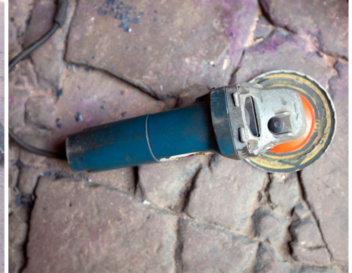
Cutting machine is used to remove the excess metal after welding process.
