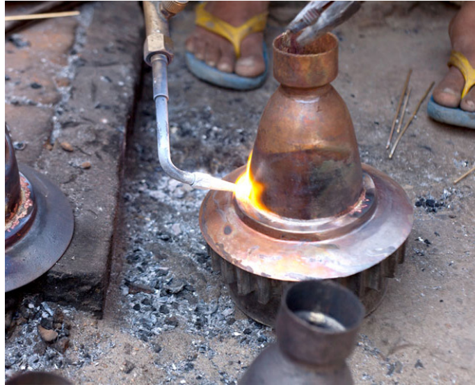
Article or different parts are being joined to make a whole product.
