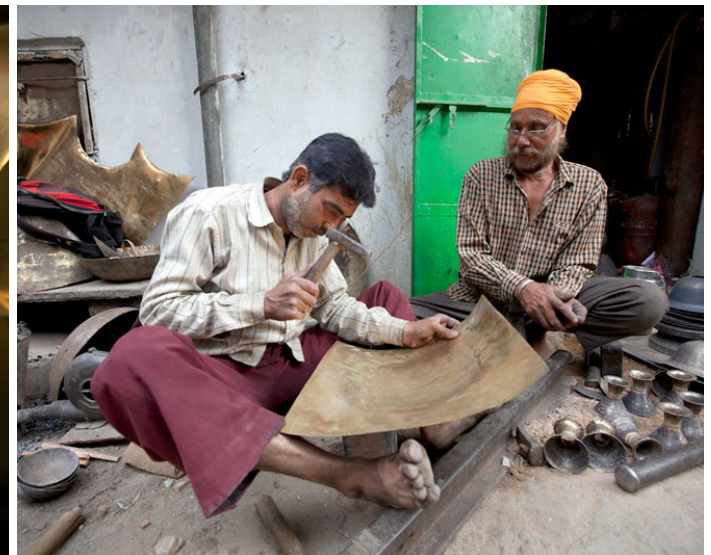
The sheet is beaten before bending it.
