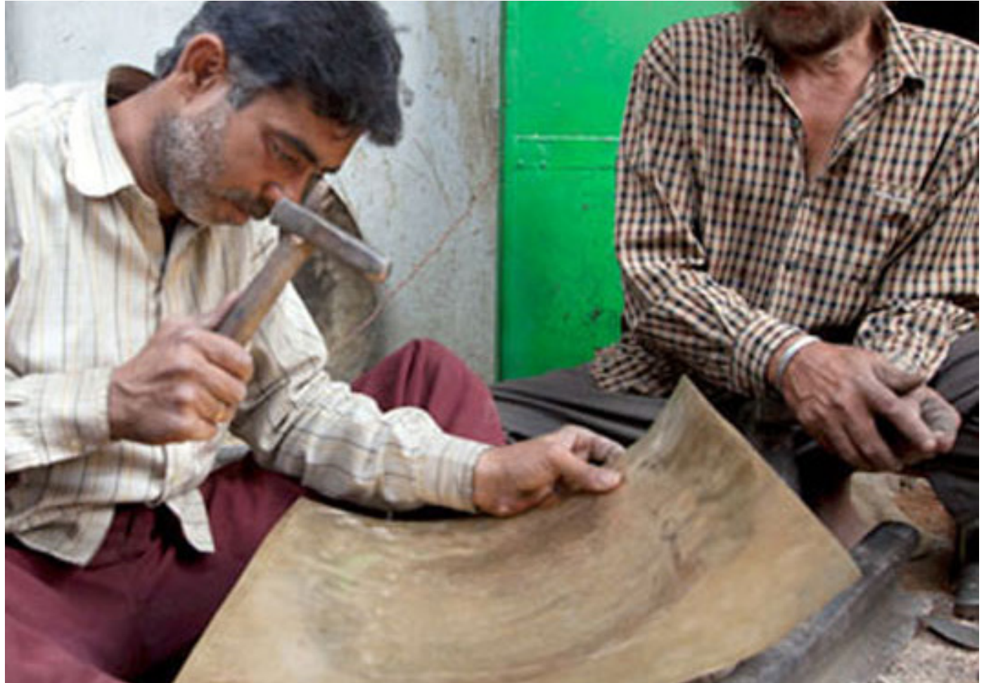
The sheet is beaten before bending it.
