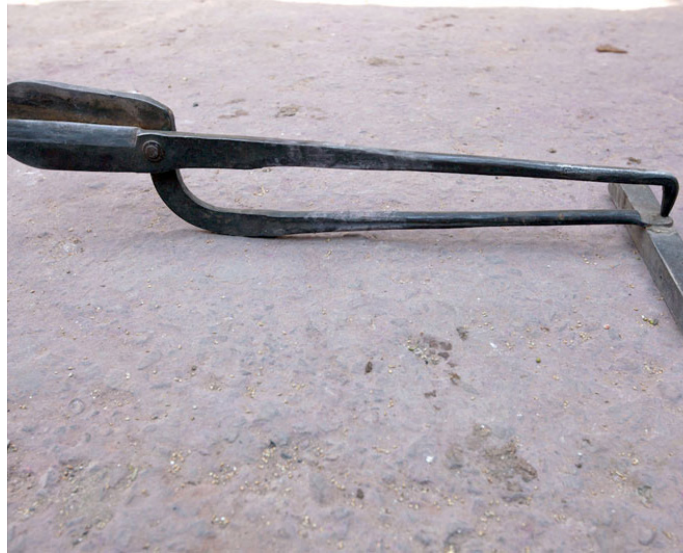
Metal Scissors used to cut the thick metal sheet.
