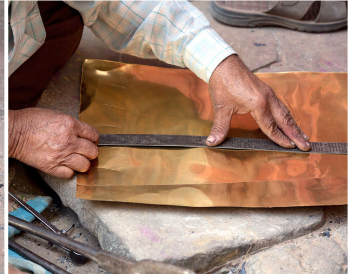
Scale is used to mark lines on the metal sheet accurately.
