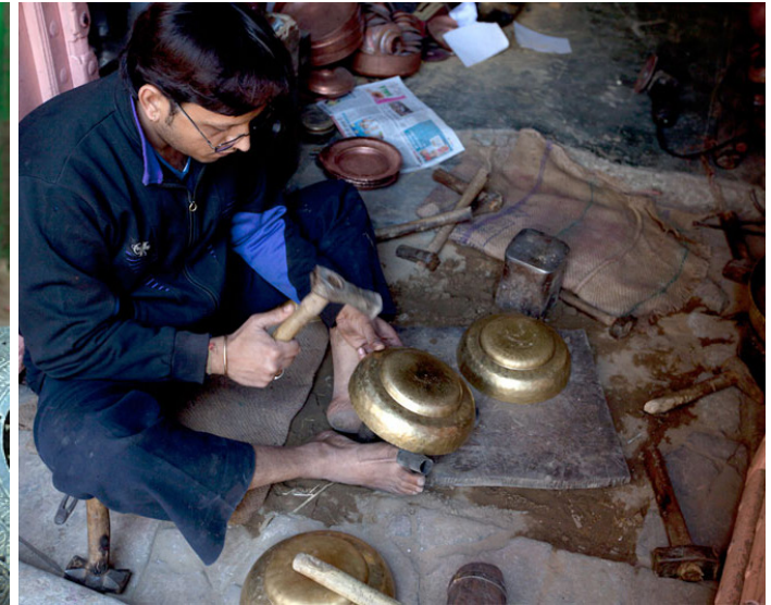
Artisan giving form and texture to a product with the help of hammer.
