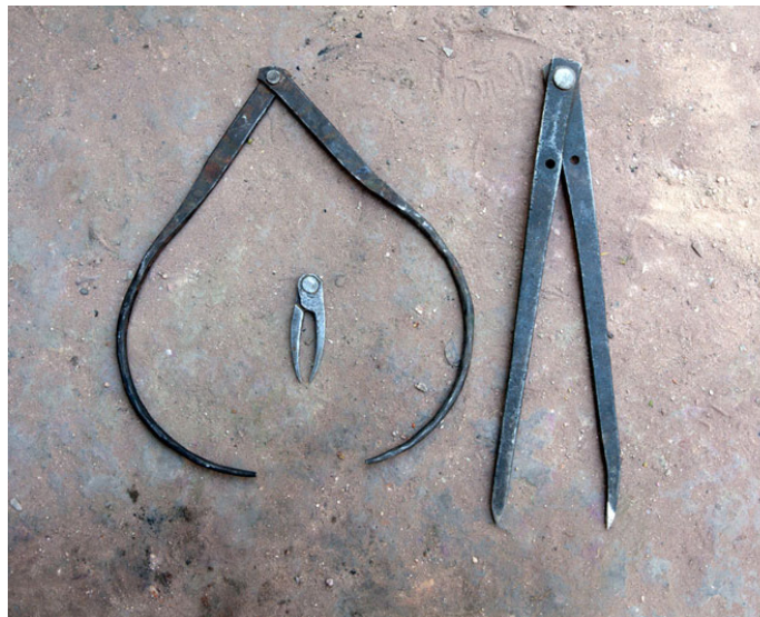
Prakaar (Compass) - Used for marking on the metal sheet.
