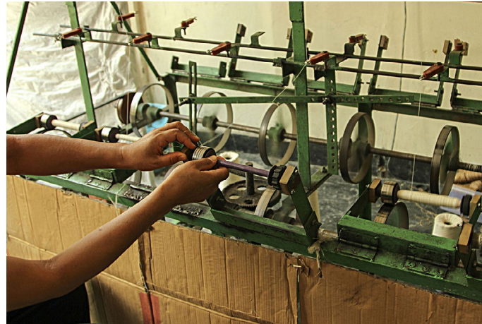
For bulk production semi-automatic winding machines are used.
