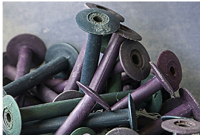
Cotton yarns are wound on plastic bobbins which are used for the warping creels.
