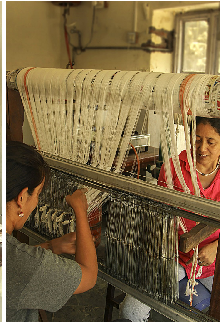
Minimum of two craftsmen are required to insert the yarn into the heddle wire.
