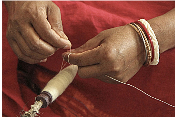
Pirns fully wound are knotted for locating the end.
