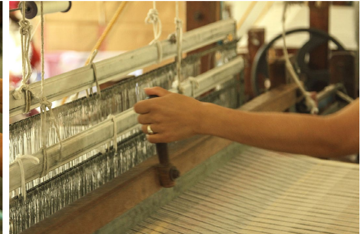
In Tibetan cotton weaving beater with handle is used to hold the yarns together.
