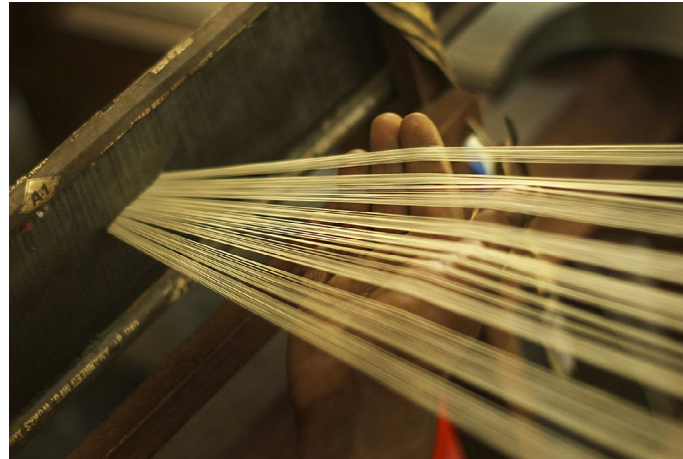
Cotton yarns are passed through the dents of the reed to beam.
