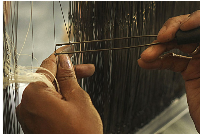
Each yarn is drawn through the heddle wire.
