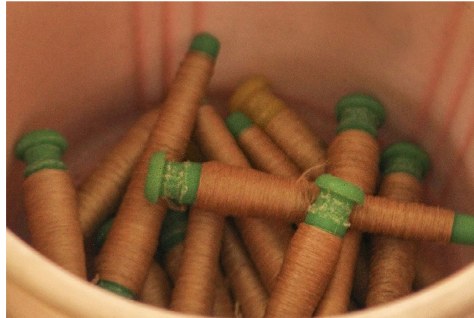
Plastic pirns are generally preferred for winding process.
