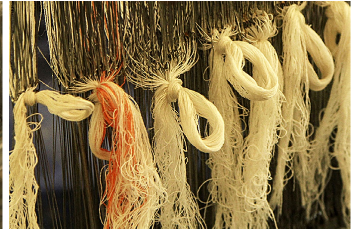
Yarns are tied together after drawn through the eye of heddle wire.
