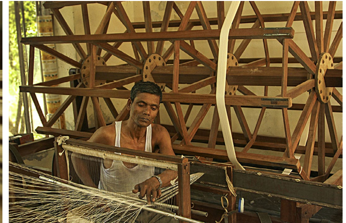
Craftsmen observes the passage of each yarn to the warp beam.
