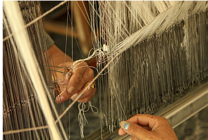
Each yarn is drawn through the eye of the heddle wire separately.
