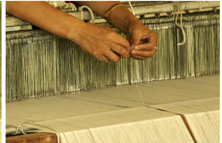
Missed yarns are located and knotted.
