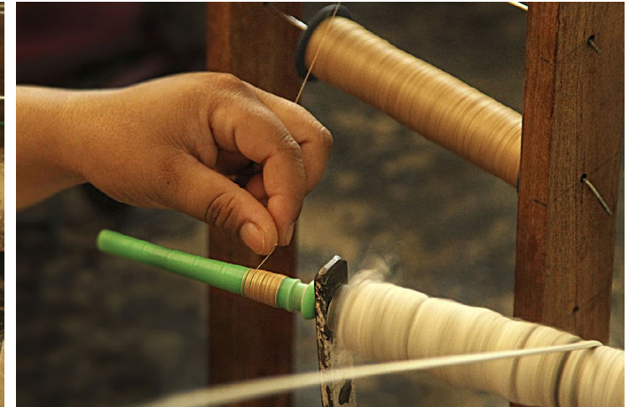
Yarns are wound to pirns from bobbins.
