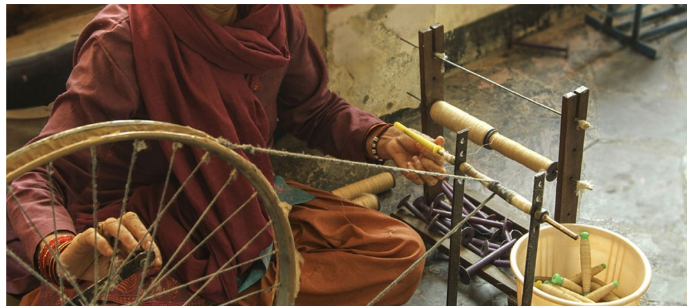
Yarns are generally wound on pirns by Charkha equipment.
