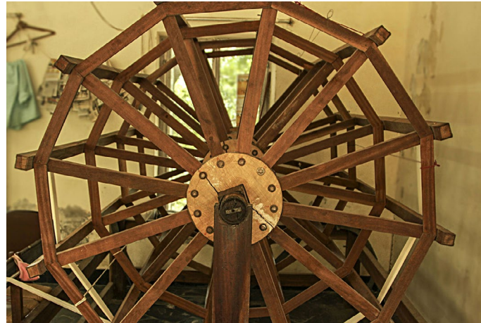
Warp beam made with wood is preferred for warping.
