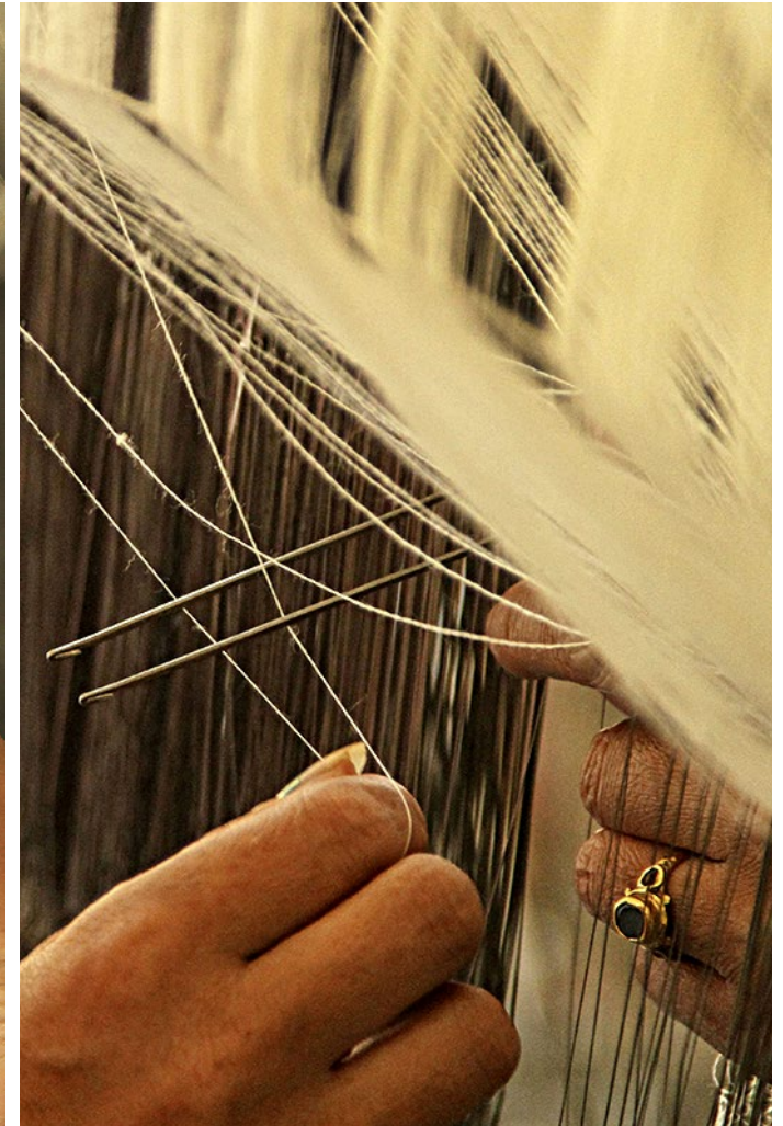
As per the pattern of design, yarn is drawn through wires.
