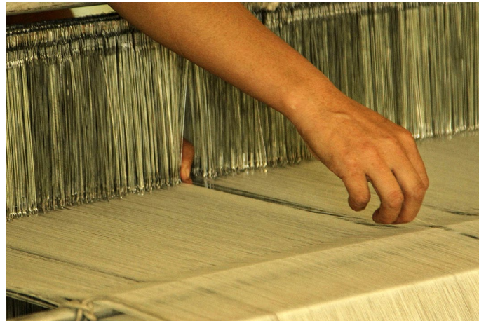
Before the loom begins, passage of the yarn is checked.
