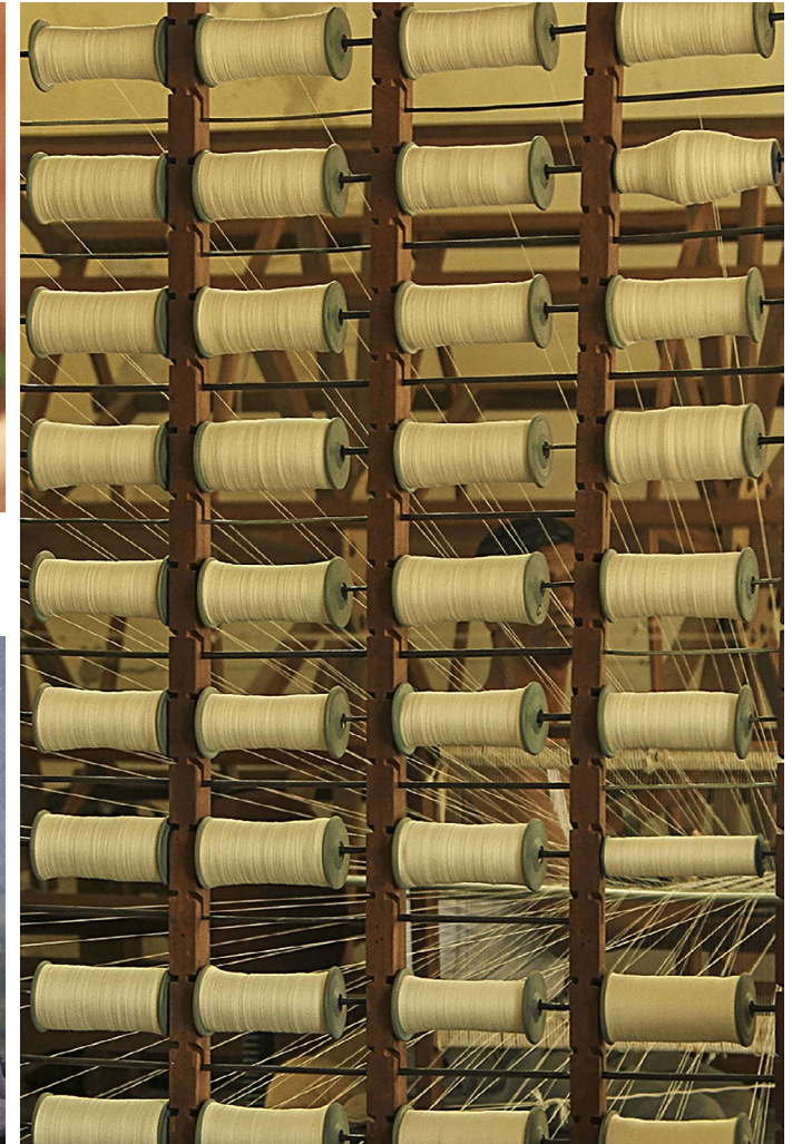
Wooden creels are generally used for warping.
