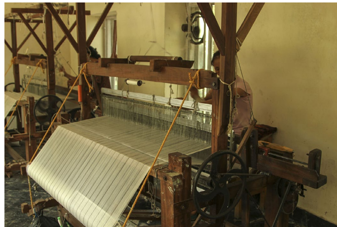
Traditional pedal loom is used for weaving the thick Tibetan fabric.
