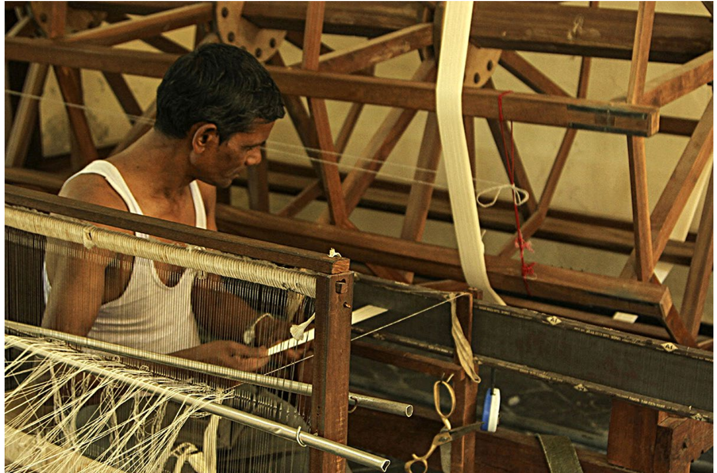
Breakages are rectified by the craftsmen and continued warping.
