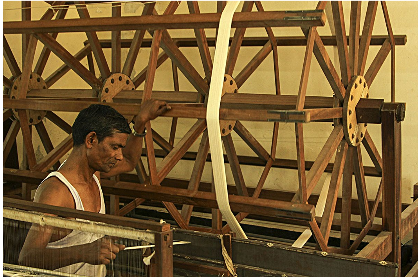
At the beginning wooden warp beam is rotated manually.
