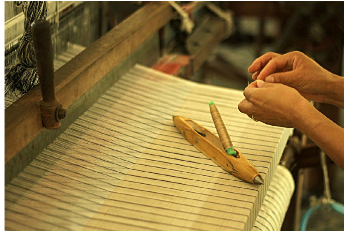
Fully wound pirns are inserted into the fly shuttle for weaving.
