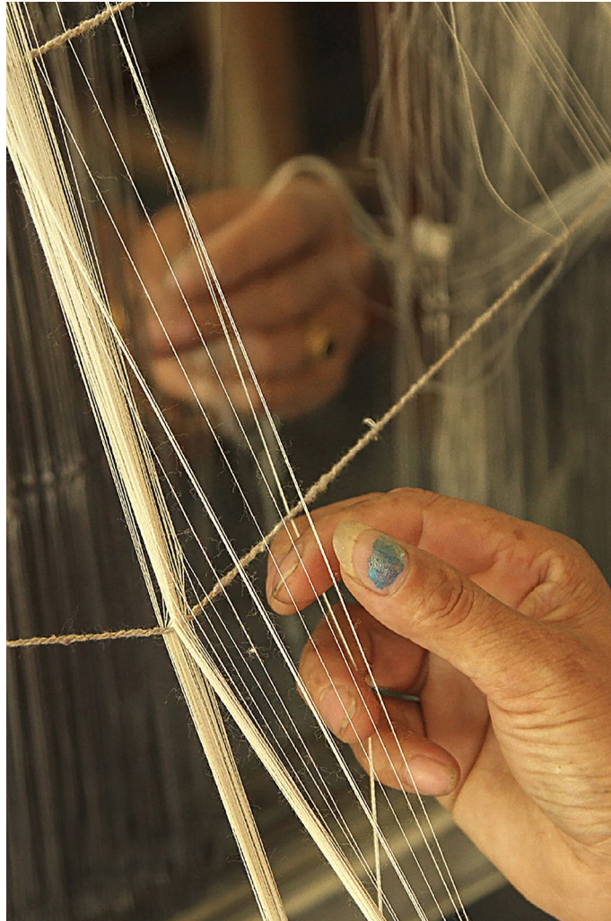
Each yarn is segregated and drawn through separately.
