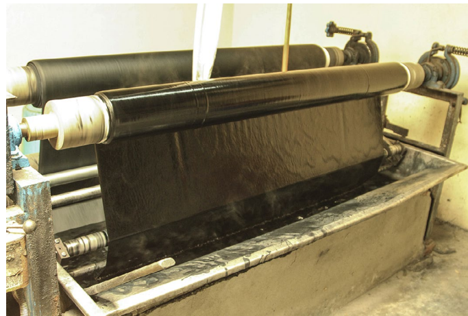
Dyeing machine with handle that operates the flow of the fabric.
