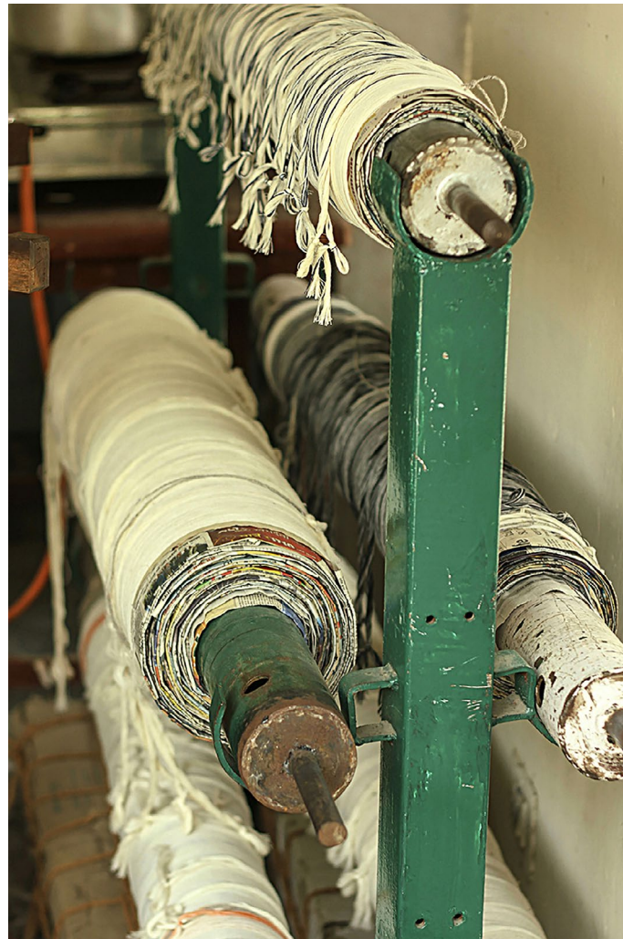
Wound warp beam ready to be inserted to the loom.
