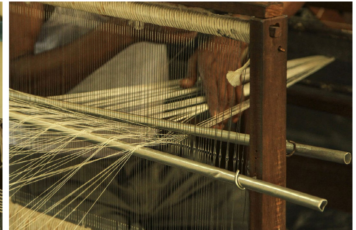
Each yarn is segregated through the eye of heddle wire.
