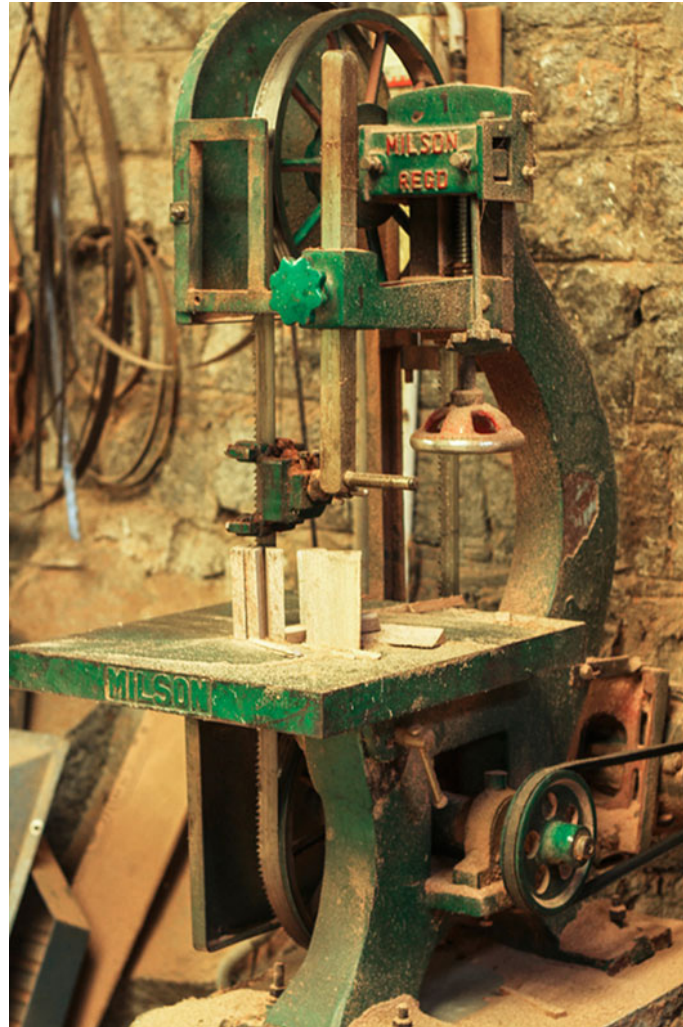
Band saw is used to cut wood into desired size and shape.
