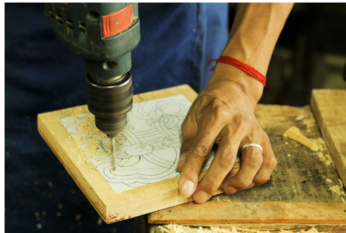
Unwanted areas on plank are removed using hand driller.
