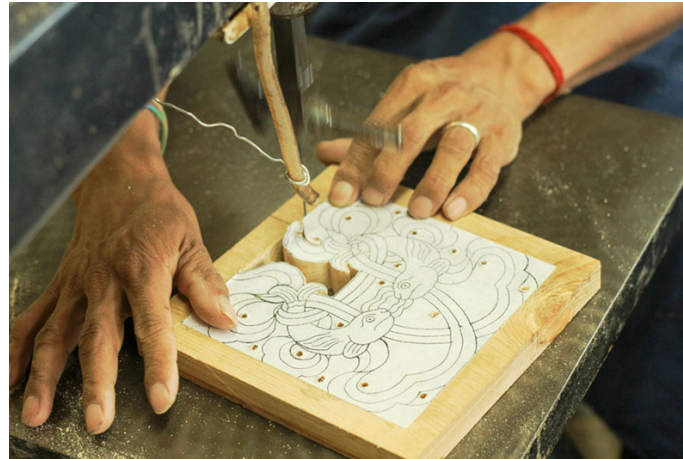
Thin wire is used to cut the unwanted areas of the wood according to drawn motifs.
