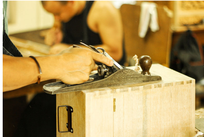
Surface of the article is leveled by scraping as a final process.
