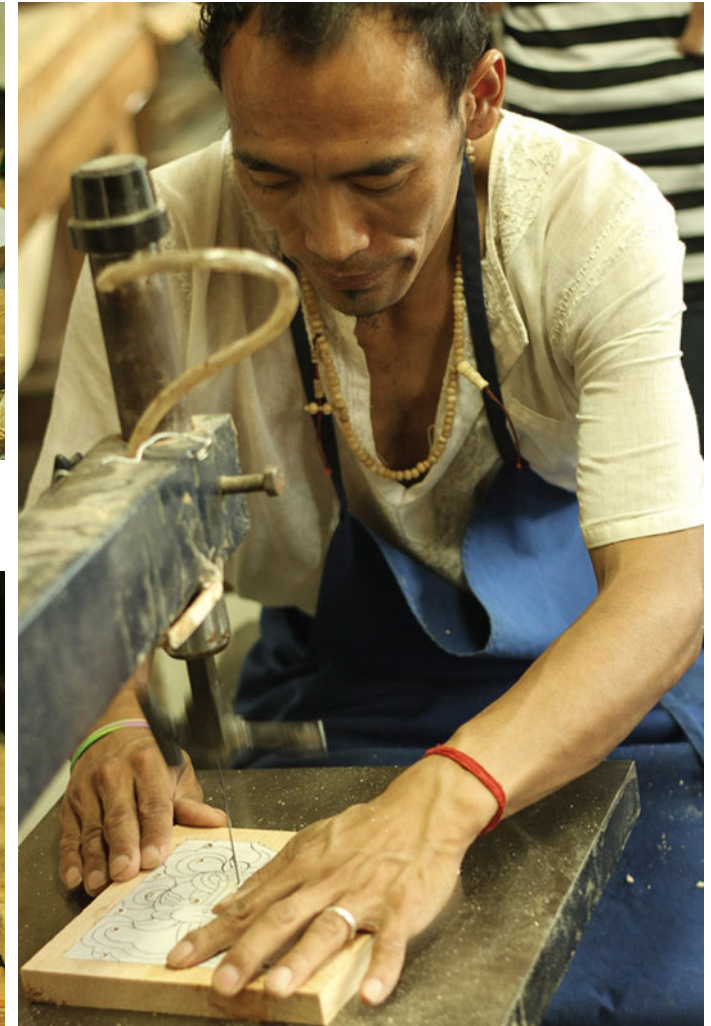
Through the drilled holes, coping saw wire is passed.
