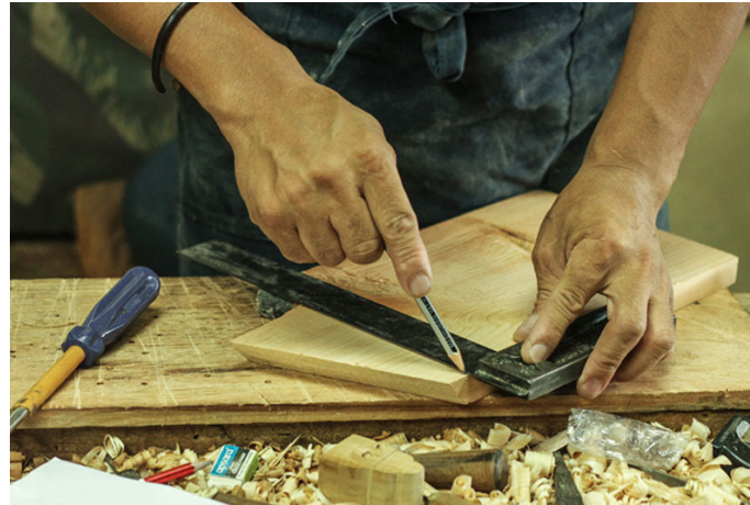
To make wooden boxes the wood is first measured and marked using tri-square.
