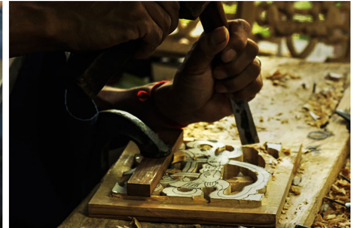
With curved chisel, the edges of the wood is carved.
