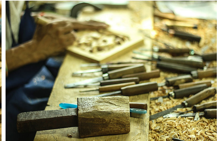
Chisels are hammered using wooden mallet.
