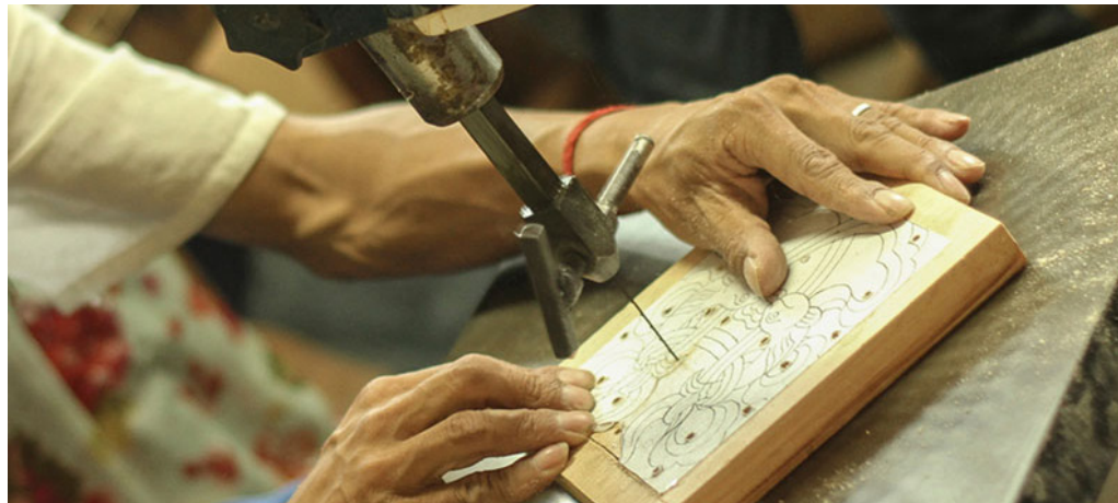
Motorized coping saw is used to cut and extract the wood between the patterns.
