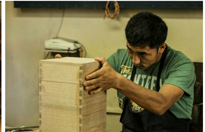
The parts of the wood are joined with the help of wood adhesive.
