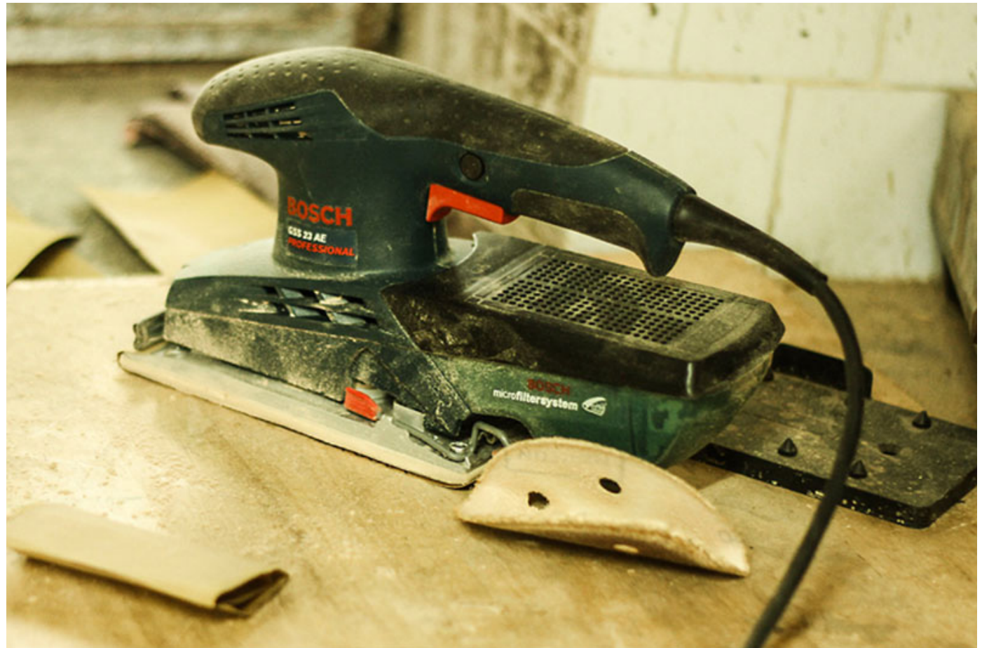
Orbital sander is used to smoothen the wood surface.
