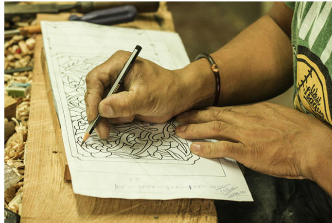
Carbon sheet is placed below the sheet to trace the motifs on the wooden plank.
