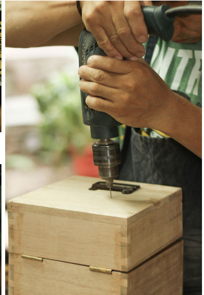
To fix the handle, exact position is marked and holes are drilled.
