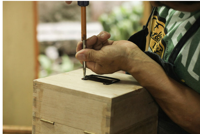
Handles are fasten with help of screw.
