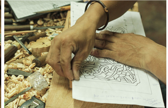
The reference design sheet is attached to the wooden plank using cello tape.
