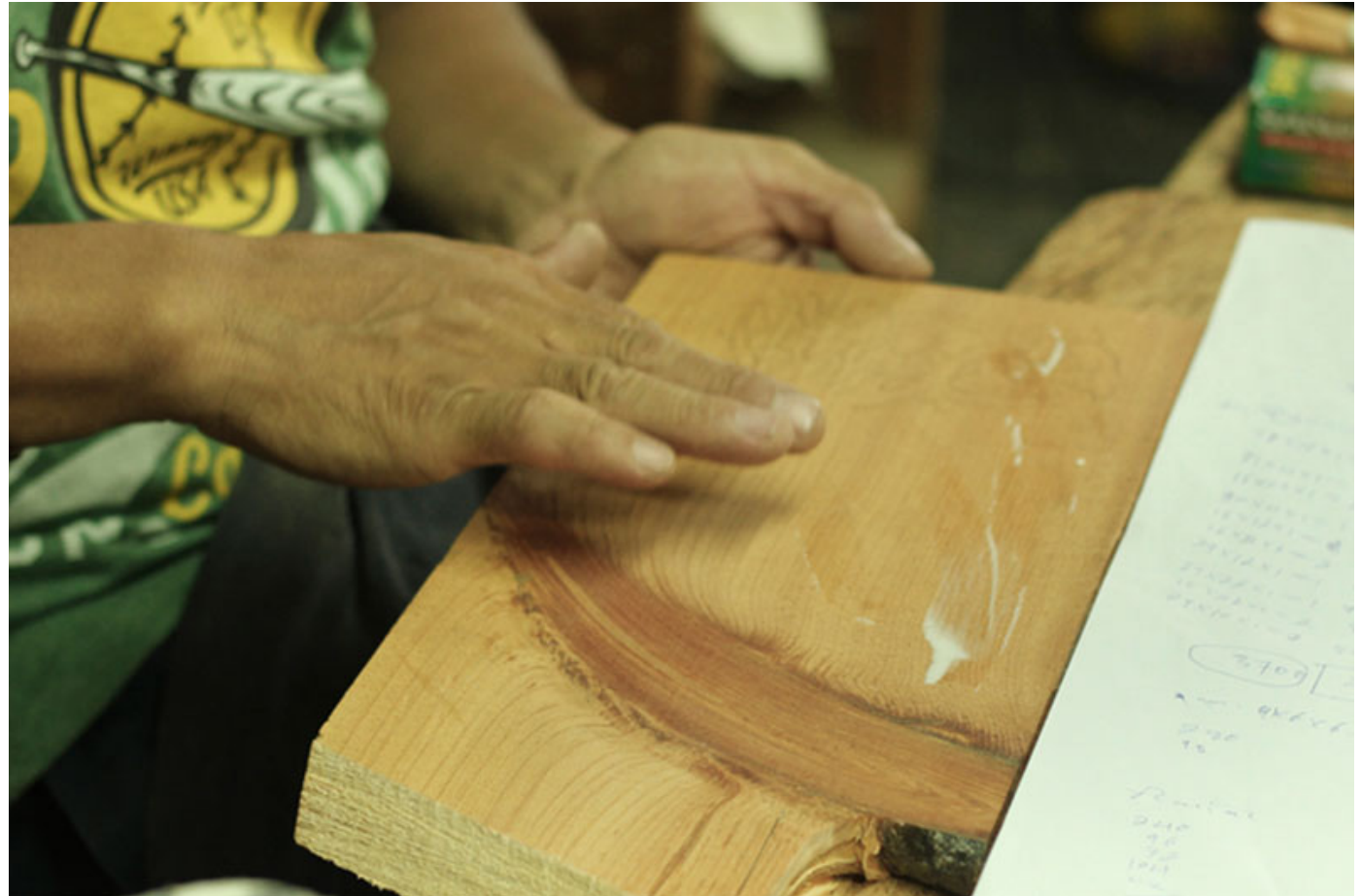
Wood adhesive is applied on the wood plank to paste the reference design sheet directly.
