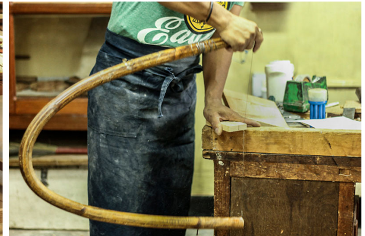
Bah (Traditional tool, Hacksaw)- used to cut the unwanted wooden part.
