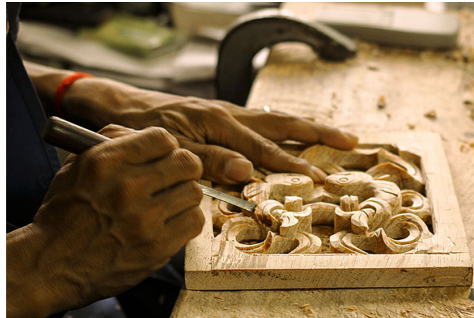
Flat chisel is used to carve and remove small chunks of unwanted wood.
