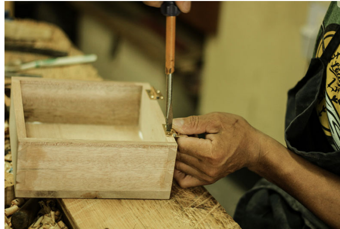
Butt hinge is fixed to attach top and bottom half of the box.
