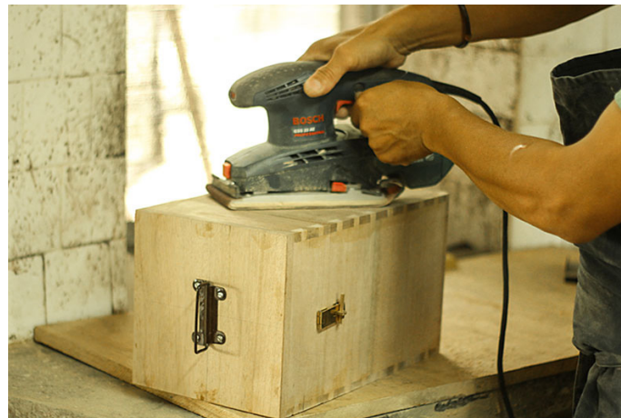
Surface of the box is smoothen using an orbital sander as final process.
