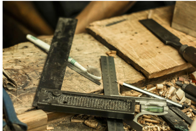
Tri square is used for measuring and marking on the wood.
