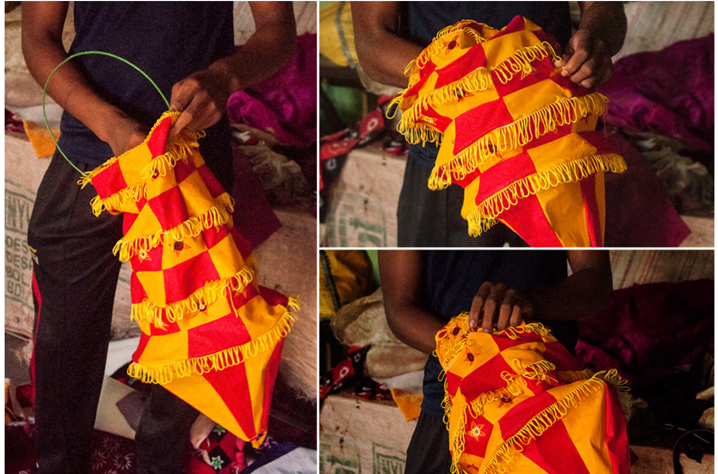
Metal wire with a plastic piping is inserted inside for the steadiness of the lamp.
