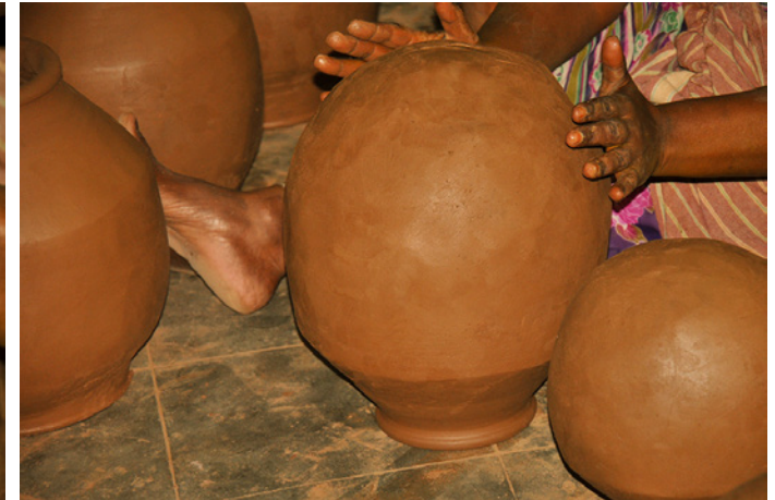
Artisan giving dome shape manually to ghatam at the back side.
