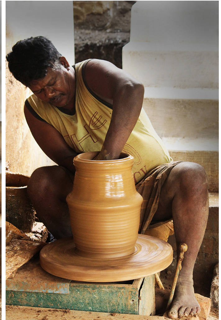
Maintaining wall thickness inside & outside.
