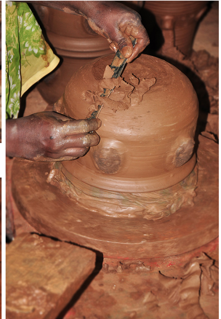
The Artisan takes to help in blade scraping the pot bottom.
