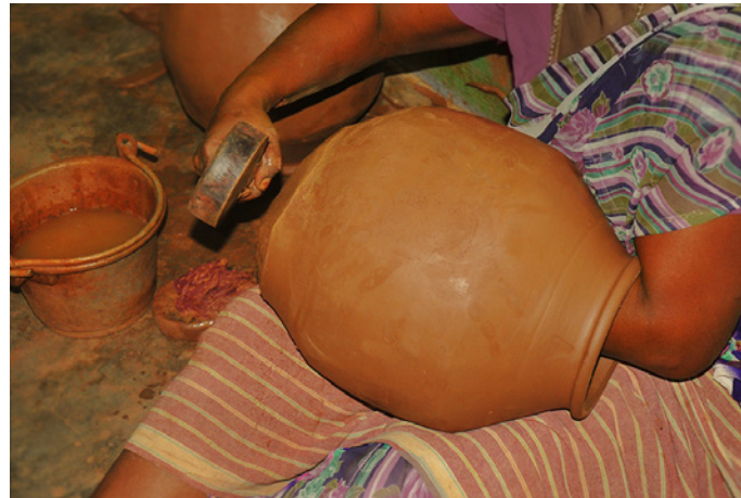
Beating the surface using wooden spatula from outside and a flat stone is supported from inside to make hard and to gain strength.
