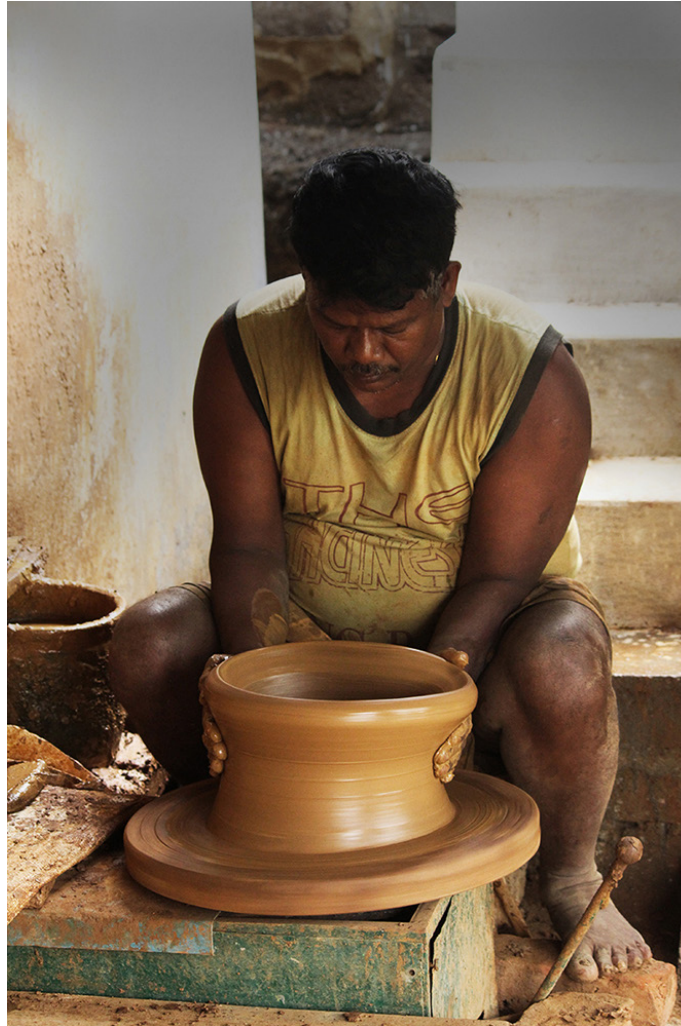
Raw clay lifted up to maintain the height.
