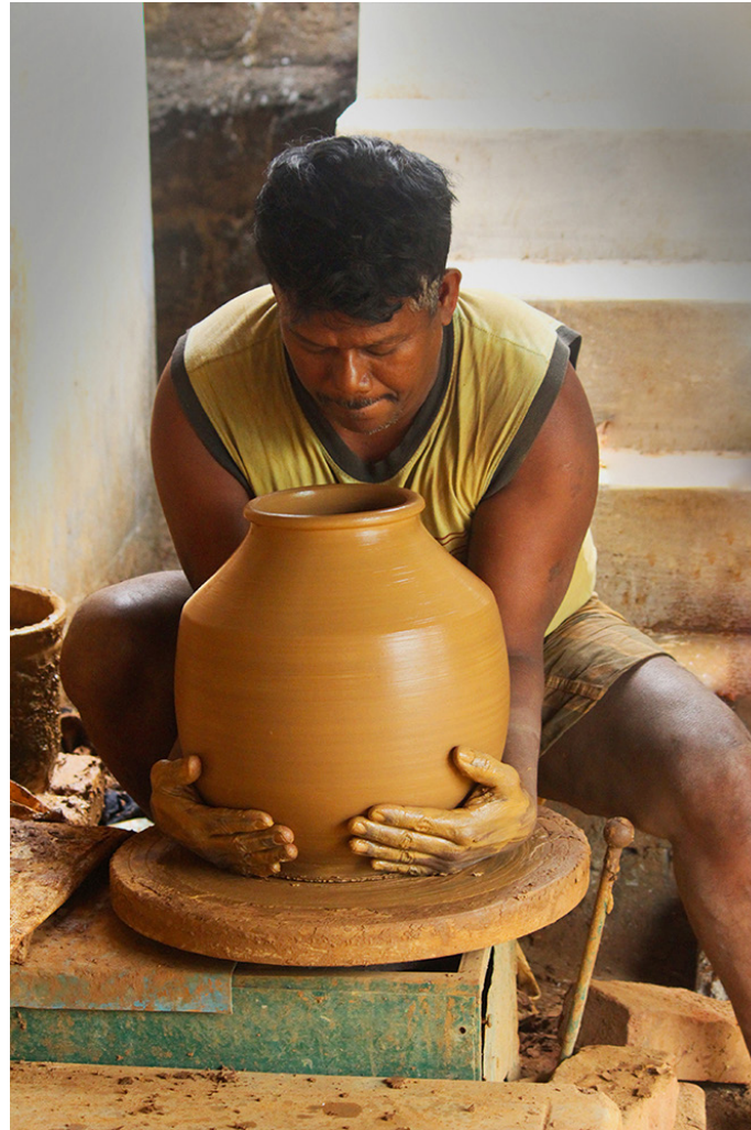
Artisan uses both hands to lift the pot from spinning wheel.
