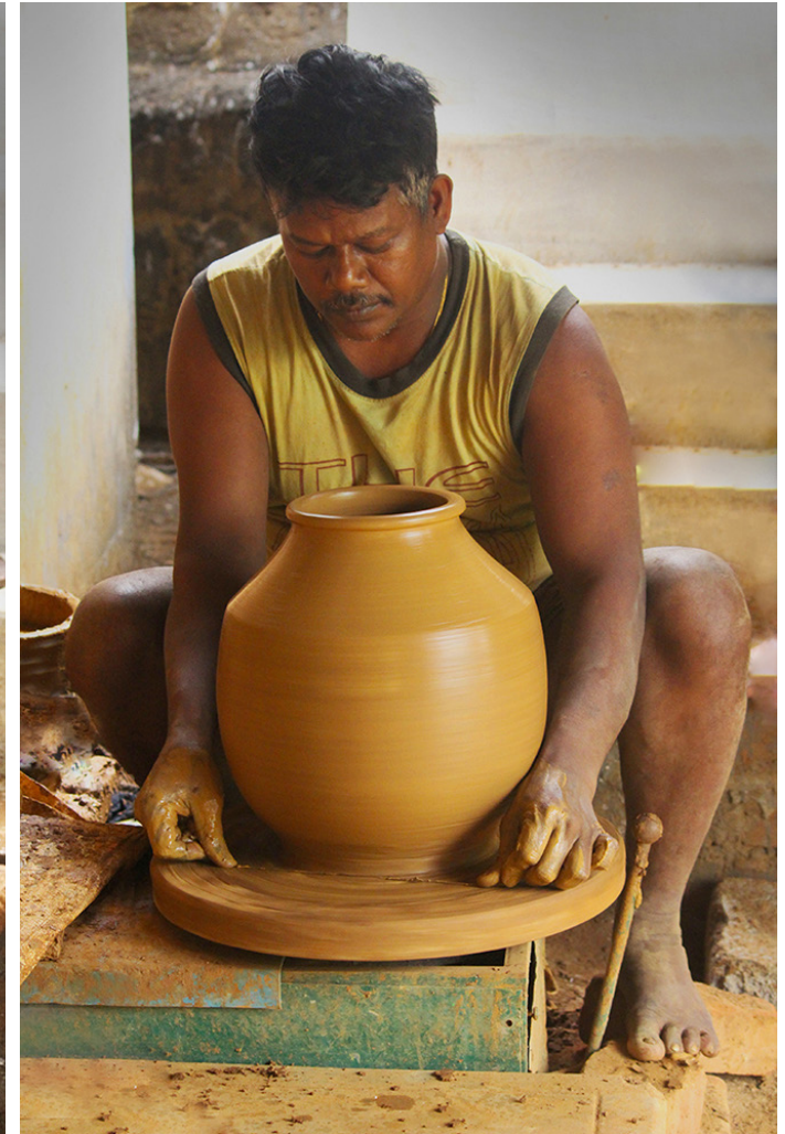
A finished pot is being removed from the wheel using the thread from bottom.
