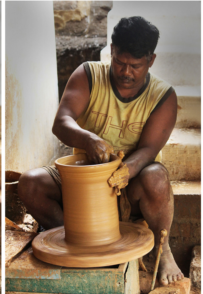
The artisan has to give the shape of pot neck.
