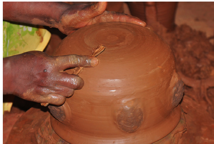
The Artisan take help in strip to scraping the pot bottom.
