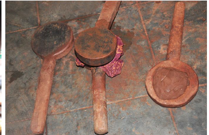
Wooden tools used to shape and give facets to the Ghatam pots.
