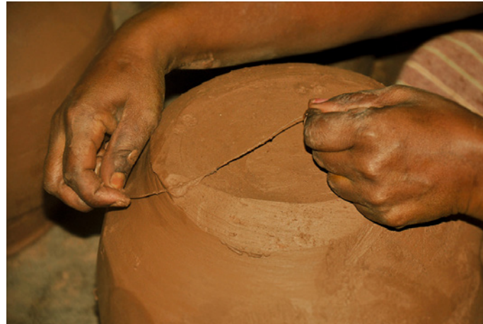
Unwanted clay is scraped at the base using cotton thread as backside is flat.
