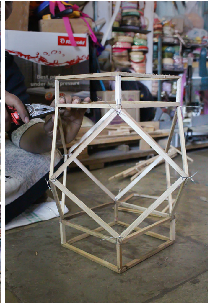
The excess binding wire is being cut with a cutting plier.
