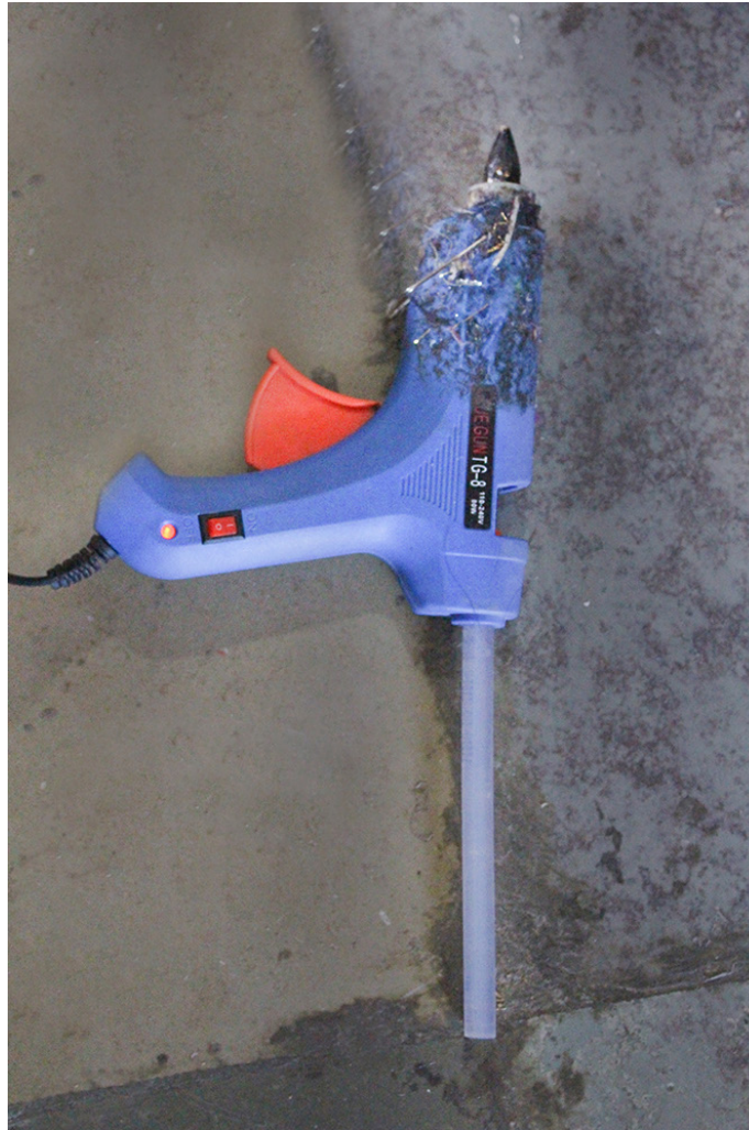
Glue gun: Glue gun is used to stick cloth and lace.
