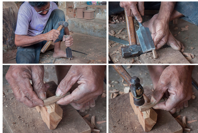
Arms for the idol are inserted by hammering the nails.
