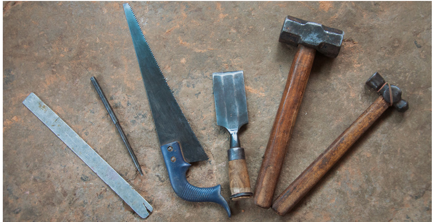
Wood carving tools – metal scale, handsaw, bull point and flat chisel and mallets.
