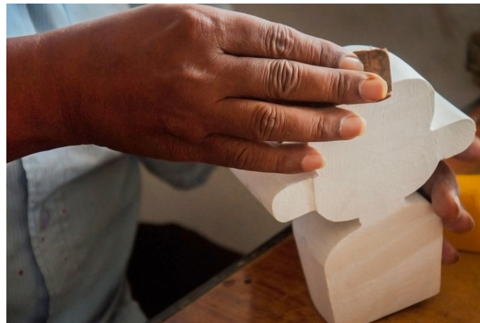
Emery paper is used to smooth the uneven surface.
