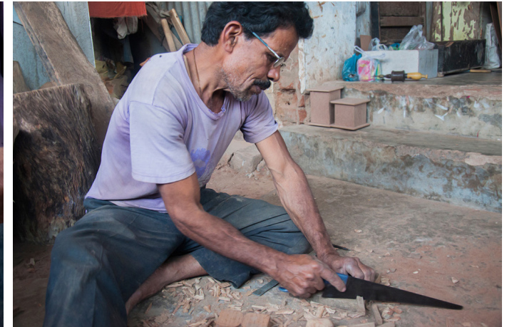
Handsaw is used to cut the wood according to the required size.
