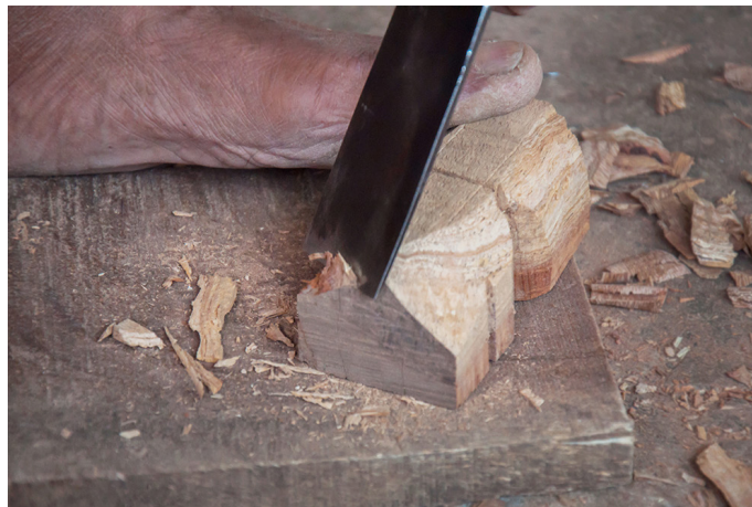
Wooden handed flat chisel is used to carve the wood.
