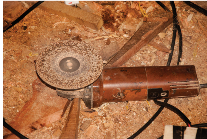
Electric hand buffing machine to smoothen the surface of the plank.
