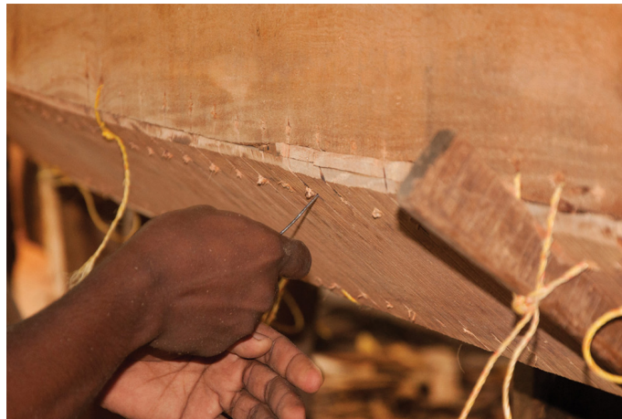
The plastic wire is stitched with big needle into corresponding groove holes made, like tying shoelace and the wire sits inside the groove line made.
