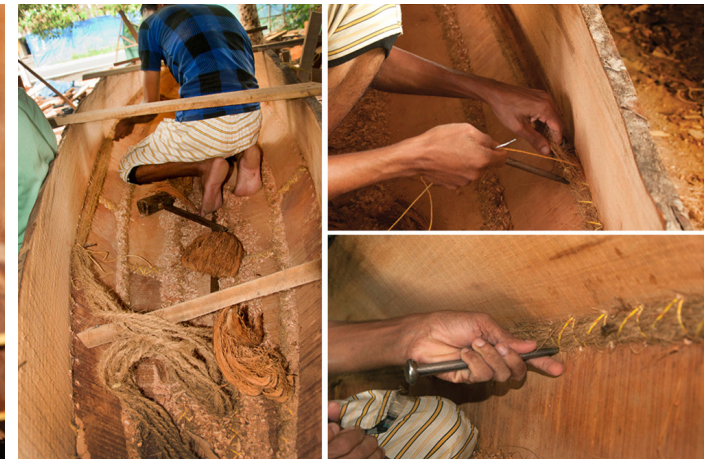
On the internal side of the boat the gaps between the planks are packed with coconut fibre threads and stitched upon it.
