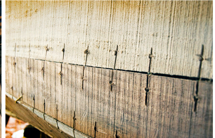
Groove lines and holes are correspondingly made on two different planks outside the boat to conceal the plastic wire woven onto it.
