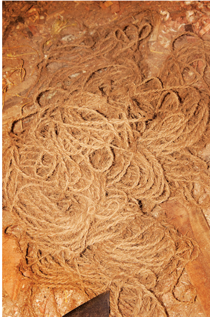
Thread made out of coconut fibre for binding and filling the gap between two planks while connecting.
