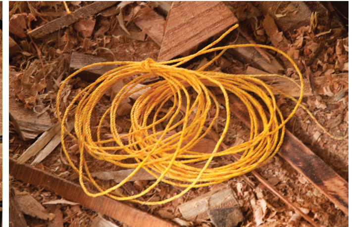
Plastic thread used in stitching the two planks together.
