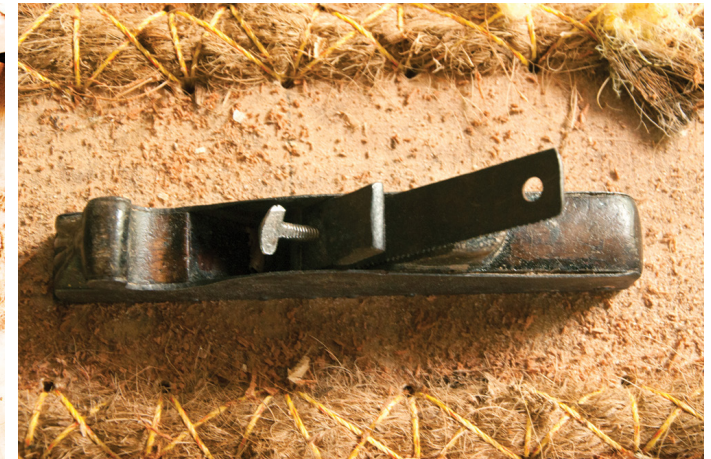
Block plane is used to flatten the plank and in finishing process.
