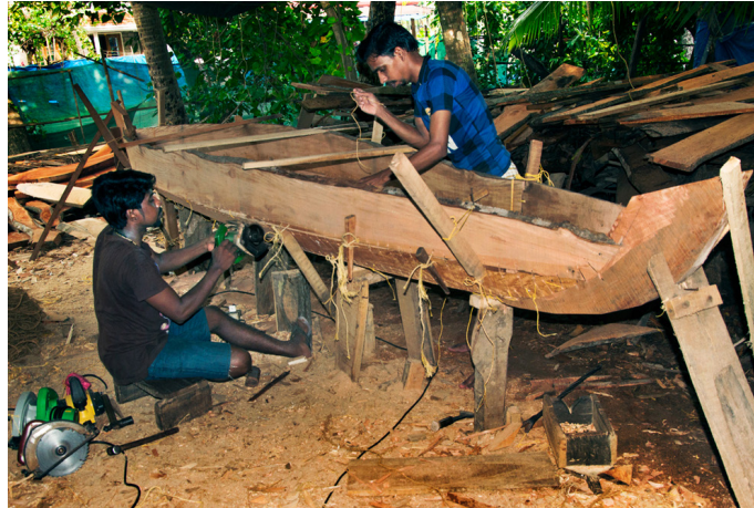
Artisan makes groove lines and holes with electric circular saw and a round bull point Chesil.
