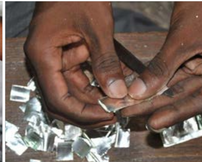
Silver strips are cut into square pieces in equal size.
