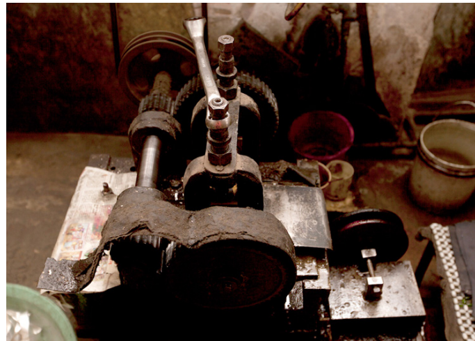
Machine to make silver or gold strips.
