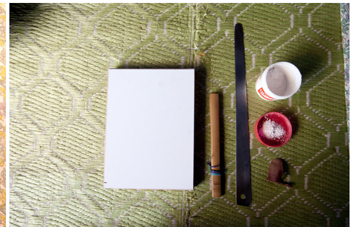
Takhti, white color flat piece of wood covered with mica to keep Varakh. Bamboo strip, cheep is used to hold the auzaars, iron cutter called as Phalua, helps in cutting the silver or gold strips, Makol, fine powder and small leather piece called as paibandi.
