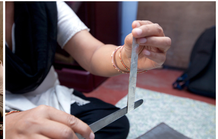
Strip is cut into smaller pieces (one inch) using Phalua.
