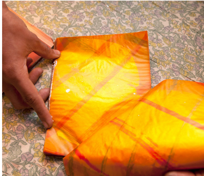
Silver piece hammered and stretched to obtained the size.
