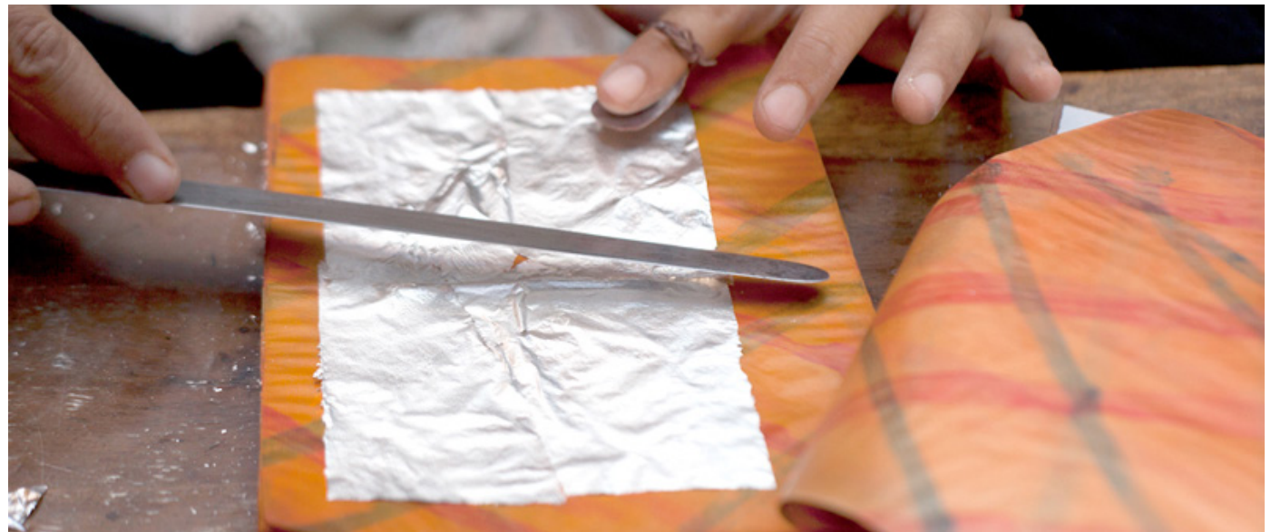
Small gaps are filled with Varakh taken from the waste Varakhs.
