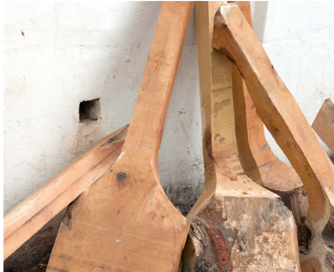
The basic rough shape of veena. Initially, the carving is done to get the precise shape for the veena.
