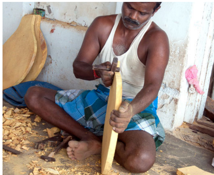
The side wall of wooden plate is smoothed.
