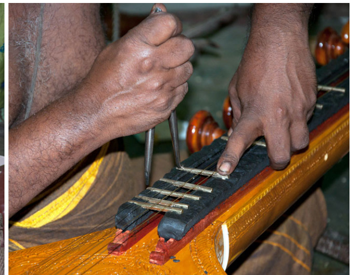
The metal frets are placed and fixed on the black dough.
