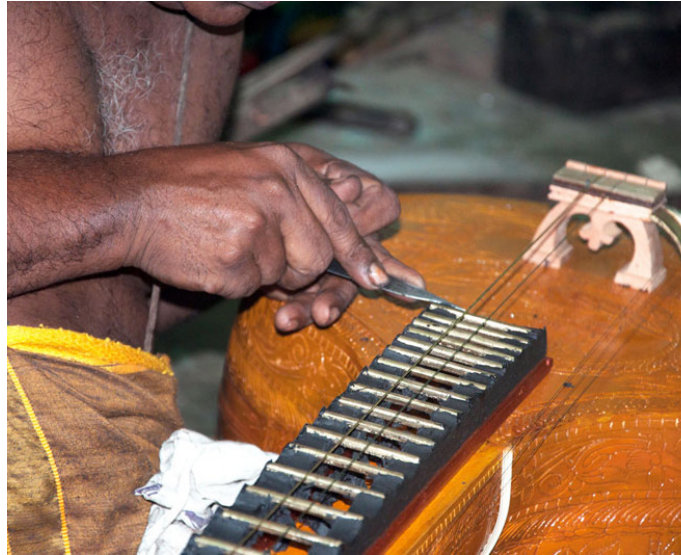
The 24 frets are fixed and adjusted.
