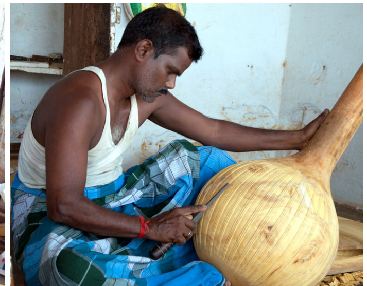
The design is created using chisels.
