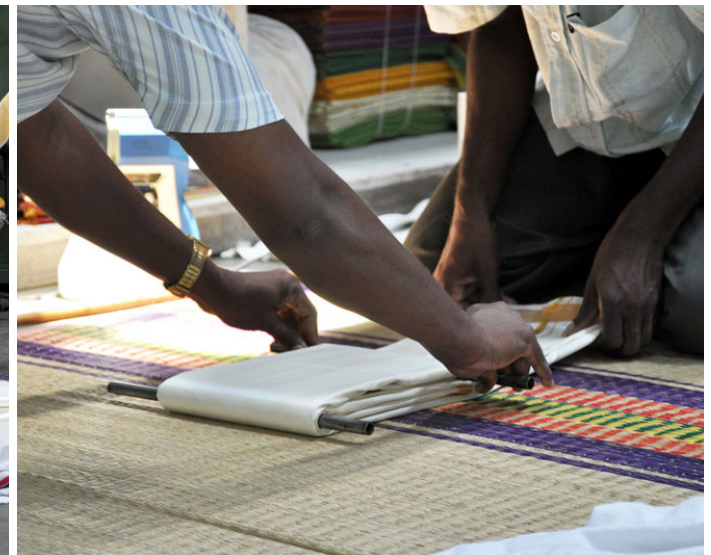
Rods are used to make crease and for folding the veshti properly.
