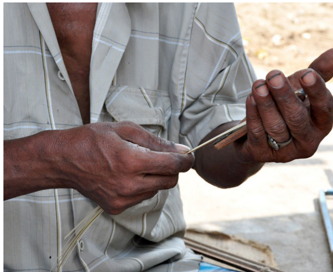
A wooden tool with blade at one end is used to measure size and eventually cut strip of equal sizes.
