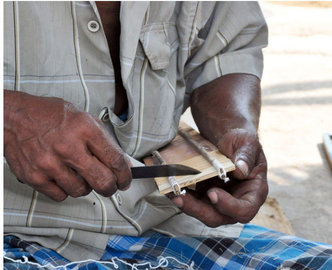
Proper gaps are made between the strips.
