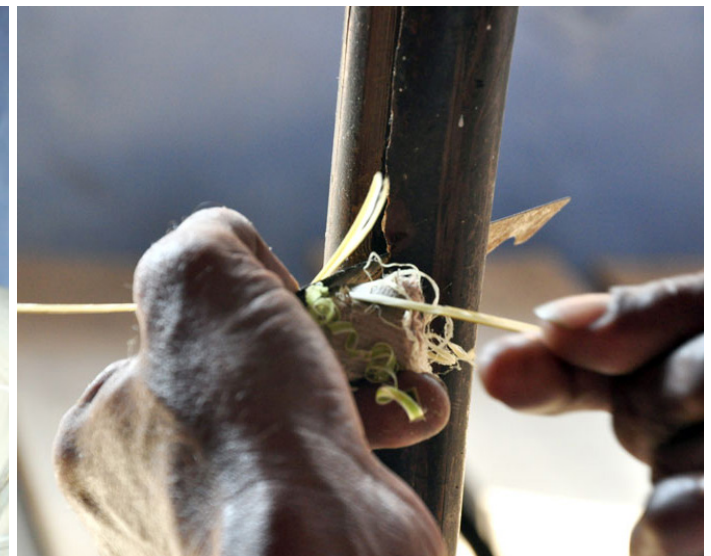
A locally made tool with blade fixed on it is used to scrap the layers of bamboo and convert it into thin smooth strips.
