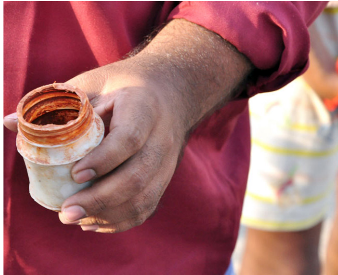
Plastic weft winding pin to be used inside the shuttle.
