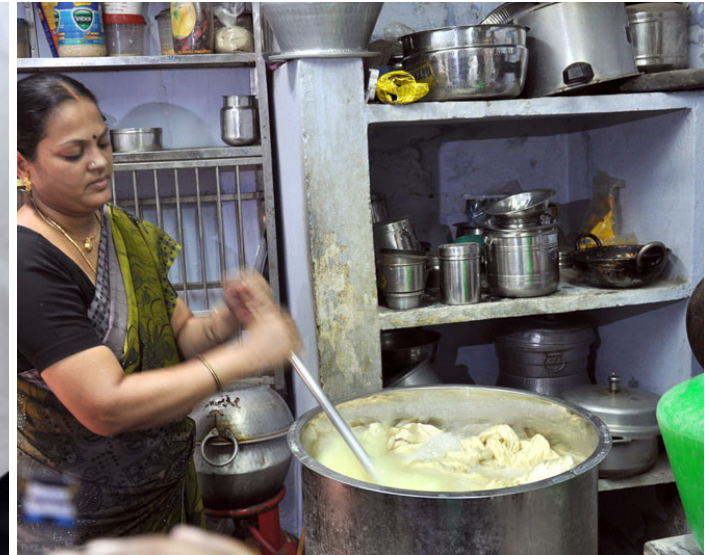
Yarns when bought from the market are boiled in bleaching powder to make it white.
