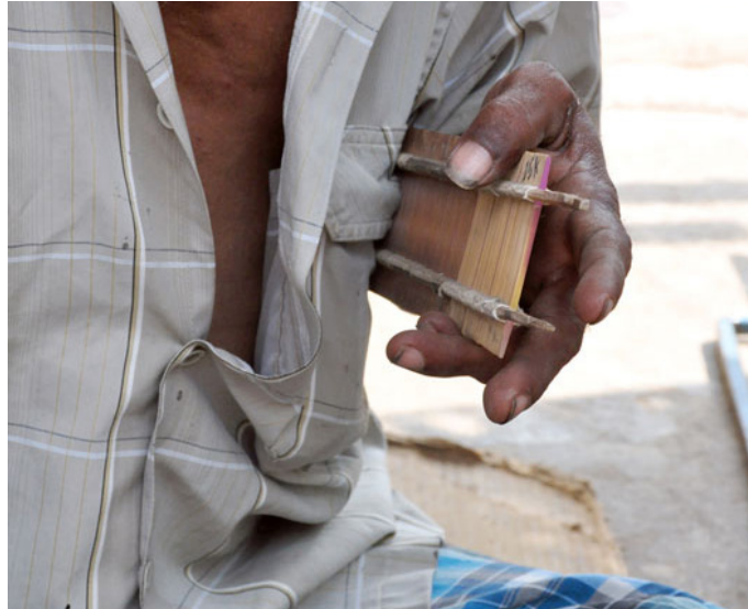
Thin bamboo strips are fixed between two parallel bamboo sticks.
