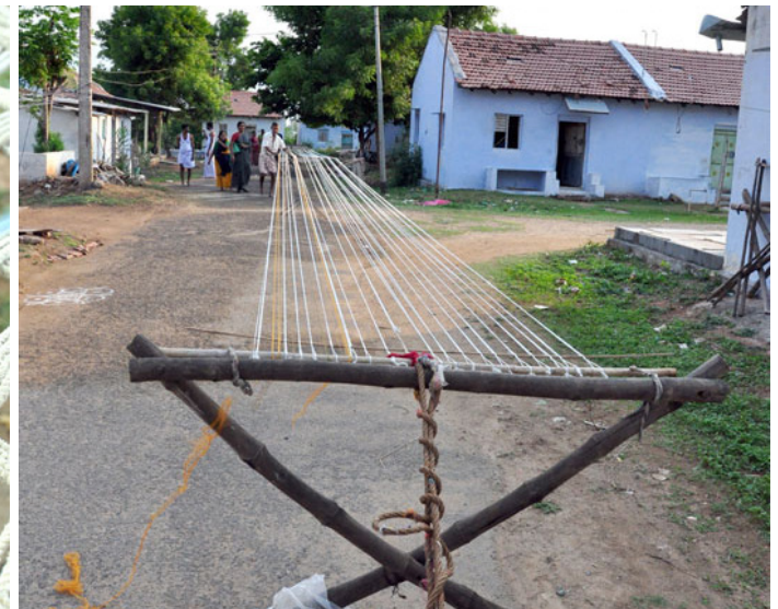
Artisans set the warp on the streets. The process is carried out early morning to avoid the heat of sunlight.
