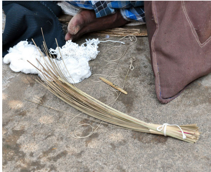
Bamboo strips and cotton thread are main raw materials used to make reed.
