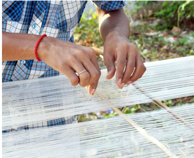
Tangles and breakages in the warp are removed by hand. Two ends of the broken yarn is tied together manually.
