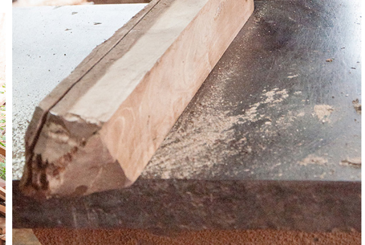
Then the wood is cut in linear motion to the required measurements in re-saw machine.
