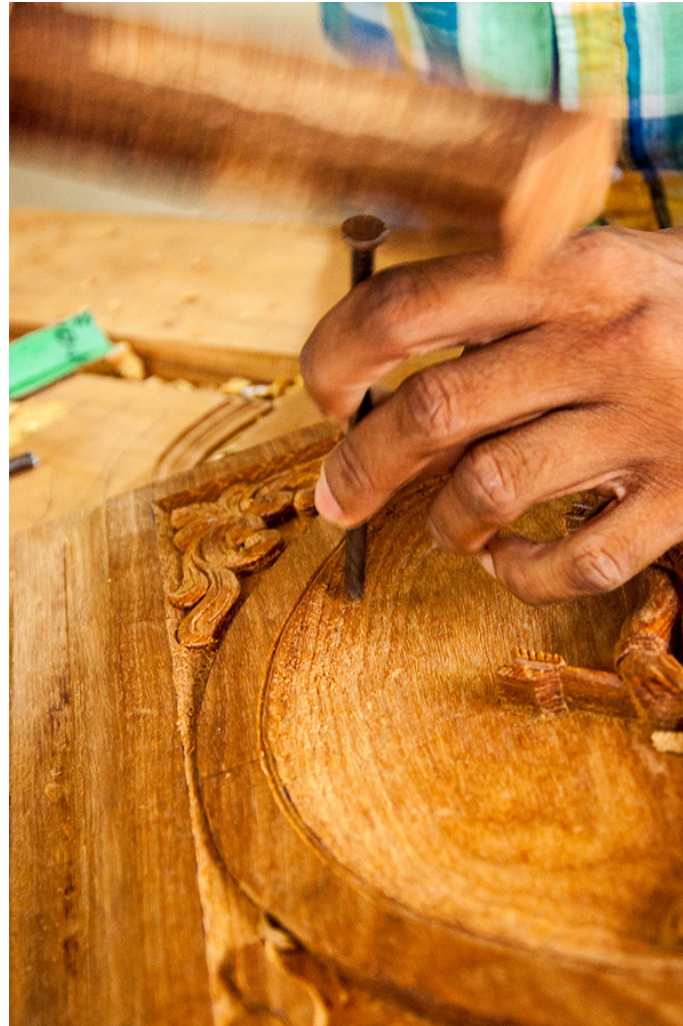
The designed screw bottoms are used for making an impression on the wood for the decorating purpose.
