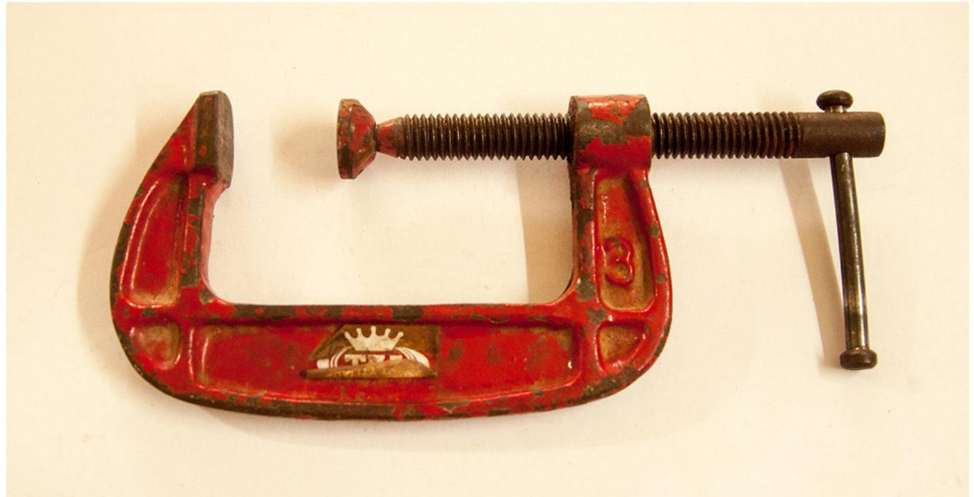
C-clamp tool used in holding the two things organized firmly.
