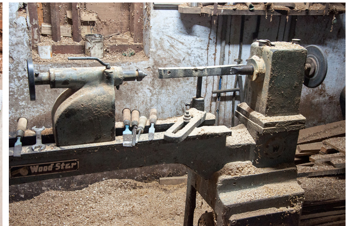
Lathe machine used for crafting the wooden log in symmetry in the axis of rotation.
