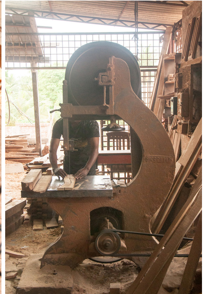
Re-saw machine that is used for cutting of the logs.
