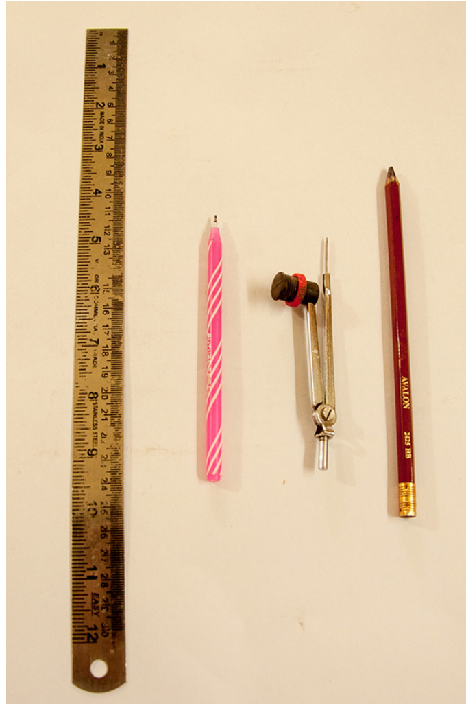
Scale, pen, compass and pencil are used in drawing of required measurements on the wooden log.
