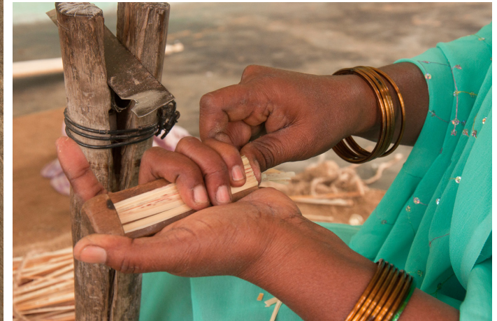
This tool helps to cut the strips into equal length.
