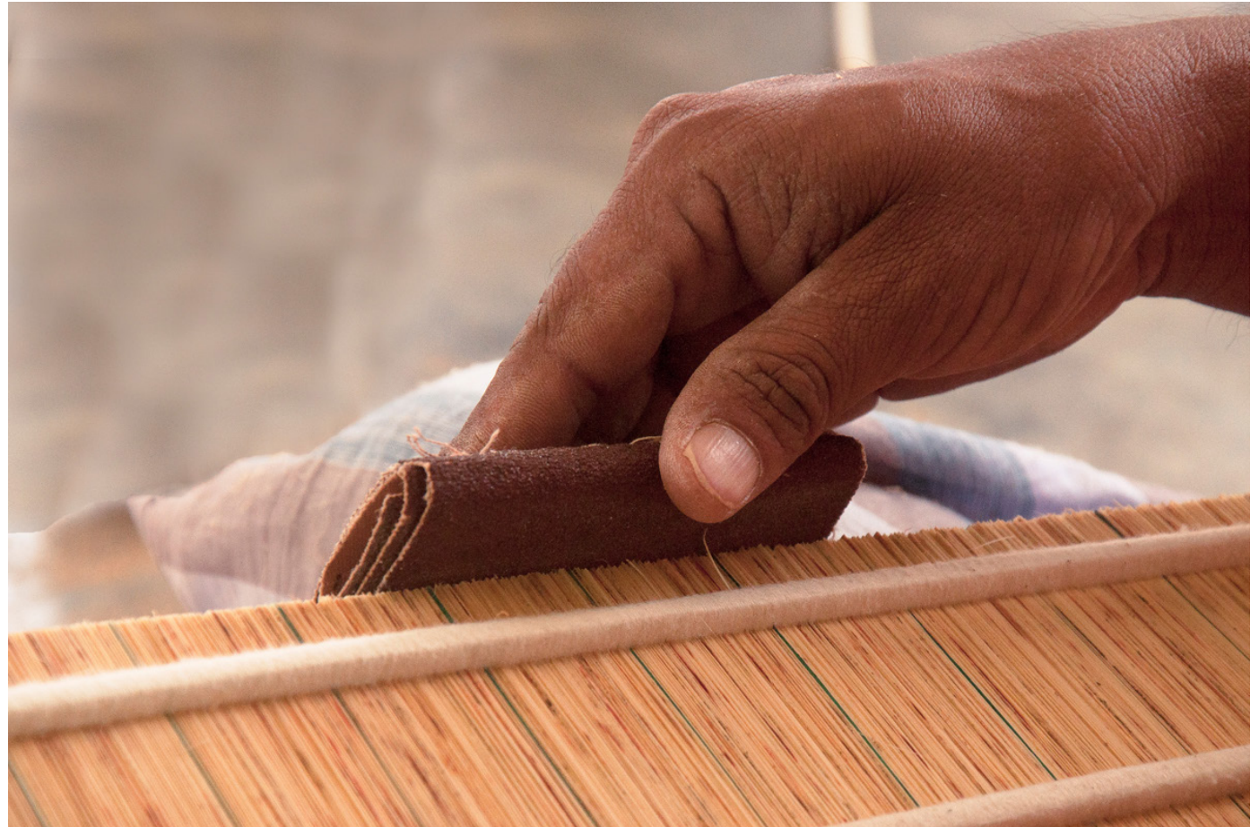
Reed is been rubbed by sand paper to smoothen the rough edges.
