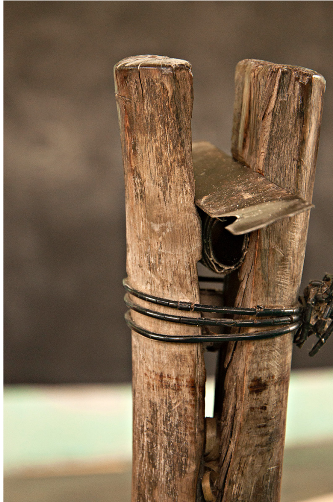
Tool locally called as Gutam is used to cut the Jowar stems into thin strips.
