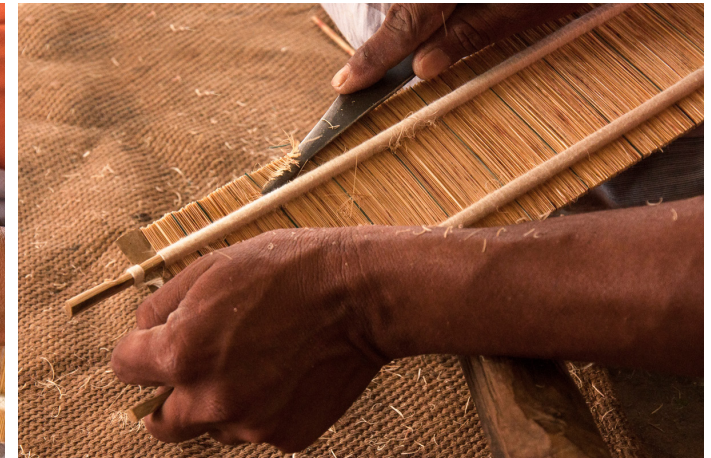
Knife is used to scrape out the rough edges and to make it even.
