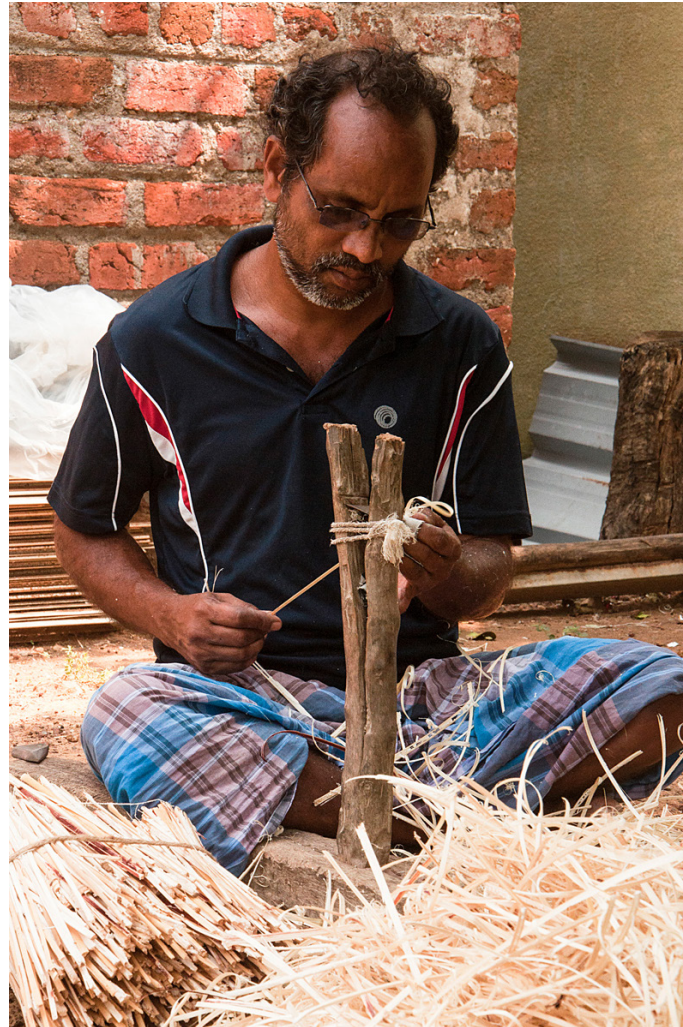
Jowar stems are cut into thin strips, which is weaved into reed.
