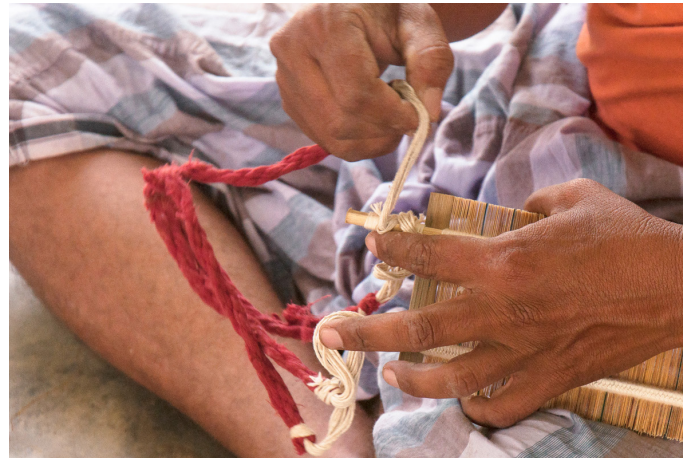
Finished reed is removed from the wooden frame and it is tied using cotton threads.
