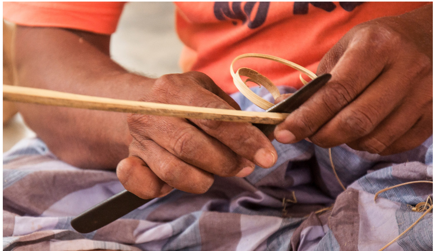
Bamboo sticks are scraped and the rough edges are removed by using a knife.
