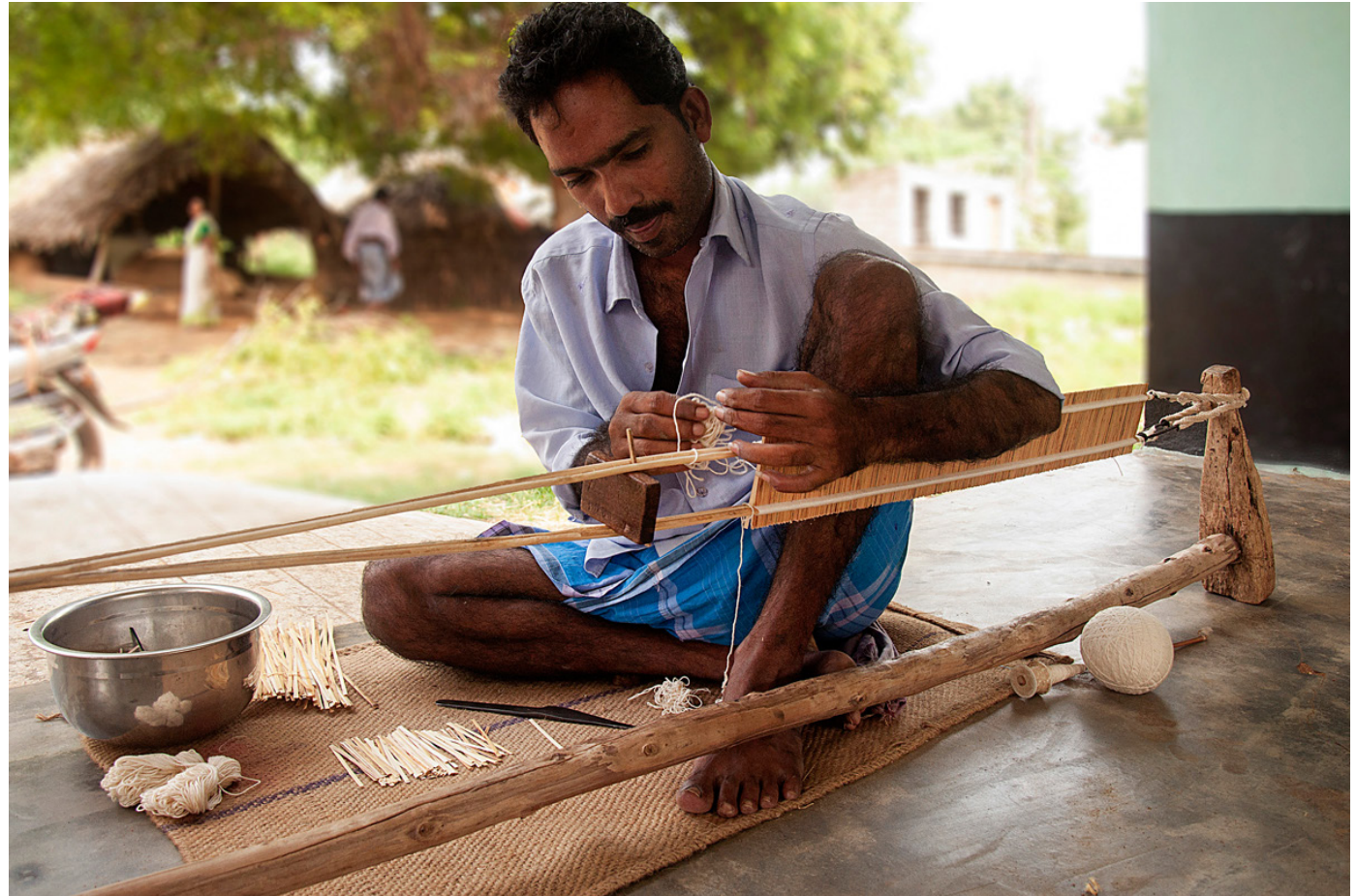
Skilled worker focuses in aligning the strips to custom the reed.
