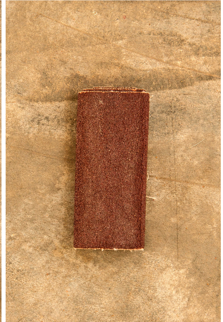
Sandpaper is used to smoothen the rough edges of the reed.
