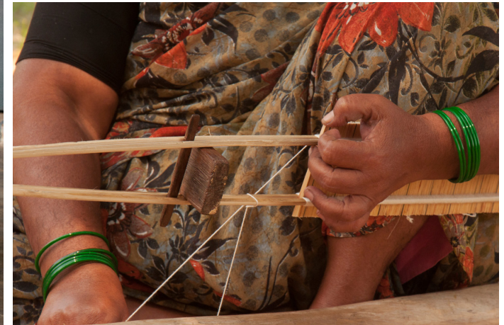
After each strip is inserted it is been locked by tying it with a cotton thread.
