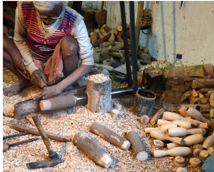
As turning begins, outer surface gets cleaned up.
