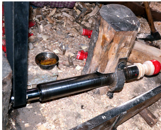
Lathe to turn the wooden blocks.
