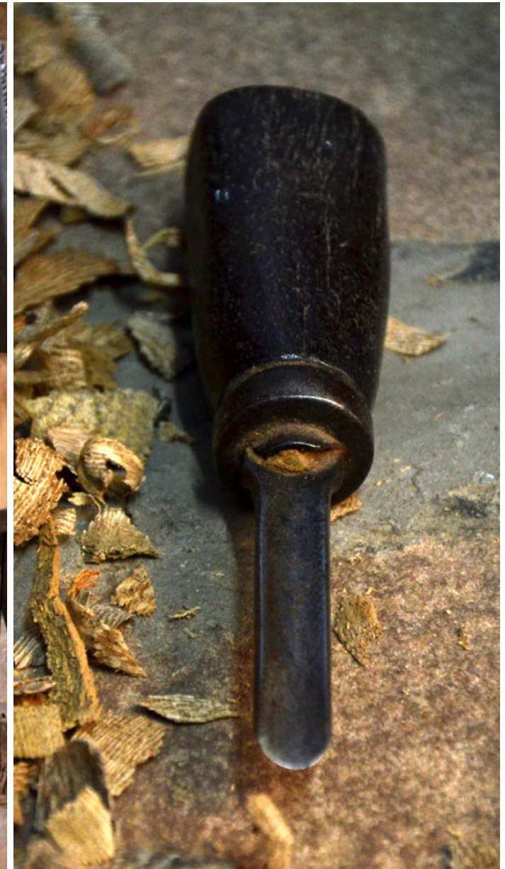
A round blade tool used to shape surfaces in curve.
