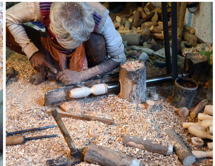
The block is reduced to the shape throughout and not at a point.
