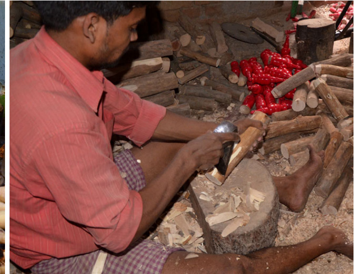
The wooden block is scraped to the closest possible form shape.
