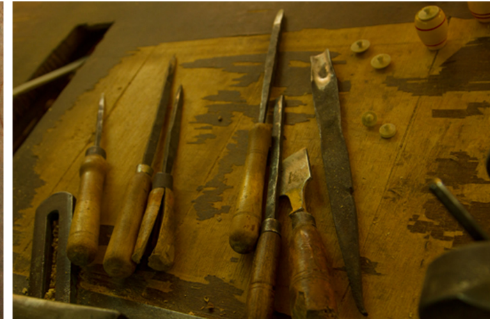
Chisels are used to carve the wood to desired shape.
