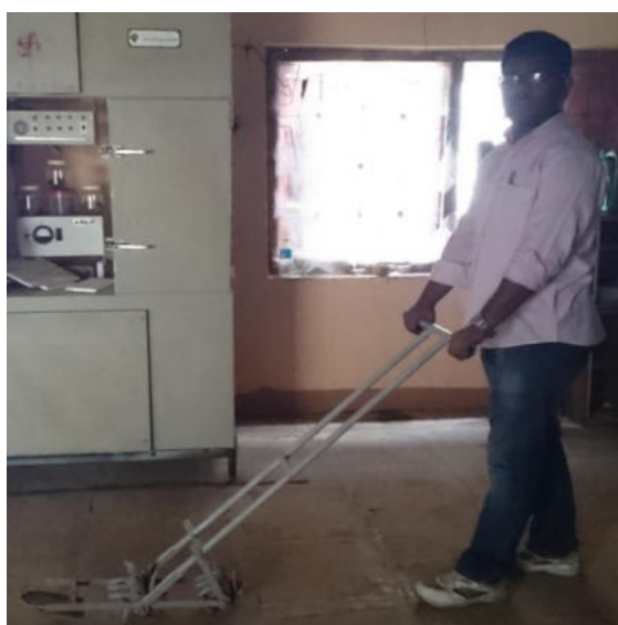
Figure-4.2: Rotary weeder developed by Rural Communes under SRI
