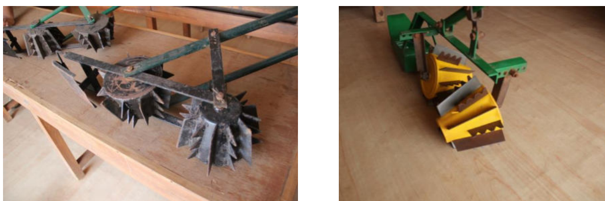
Figure-4.7: Cone detail of DBSKKV weeder and TNAU weeder
