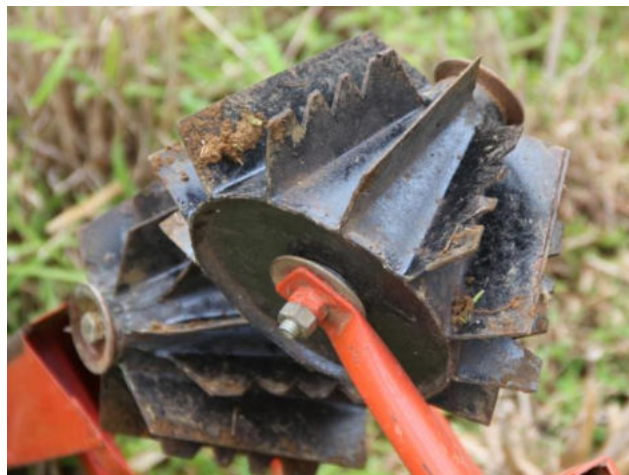
Figure-4.10: CIAE weeder cone and blades detail
