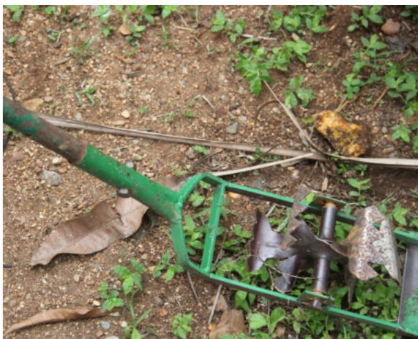
Figure-4.13: CIAE weeder wheel arm detail
