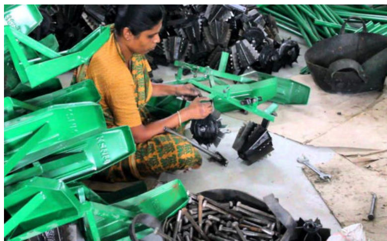
Figure-3.11: Assembly of conoweeder at KSNM factory
