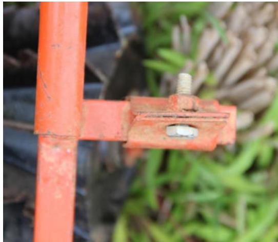
Figure-4.12: CIAE weeder wheel arm detail
