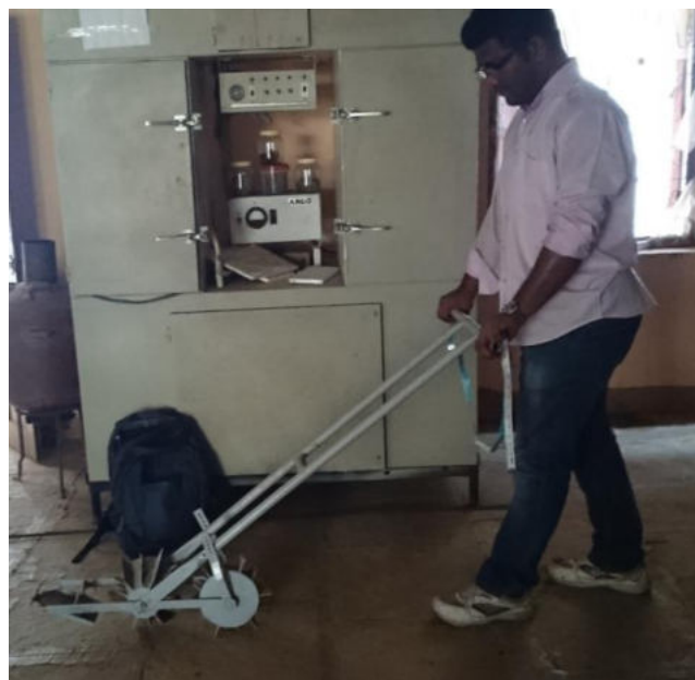
Figure-4.4: Conoweeder developed based on Japanese weeder
