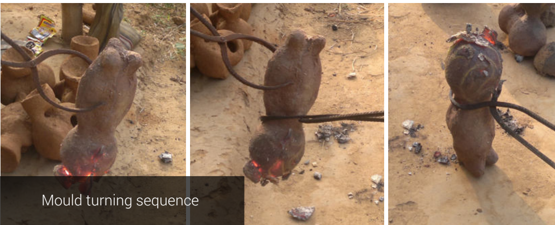
Mould taken out of kiln
