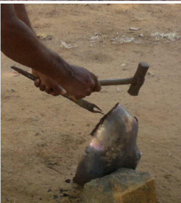
Breaking metal utensils and putting pieces in crucible
