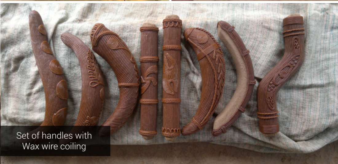
Wax coiling on clay core
