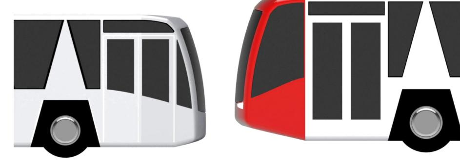
In this variation, the FRP part meets the body ahead of the door frame, giving a much sharper corner at the top. Also, the two front headlamps are joined together be a black plastic strip.
