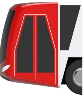
In this Variation, the chamfer length is decreased to visually balance the glass and FRP areas, as well as to allow for a wider opening of the door.
