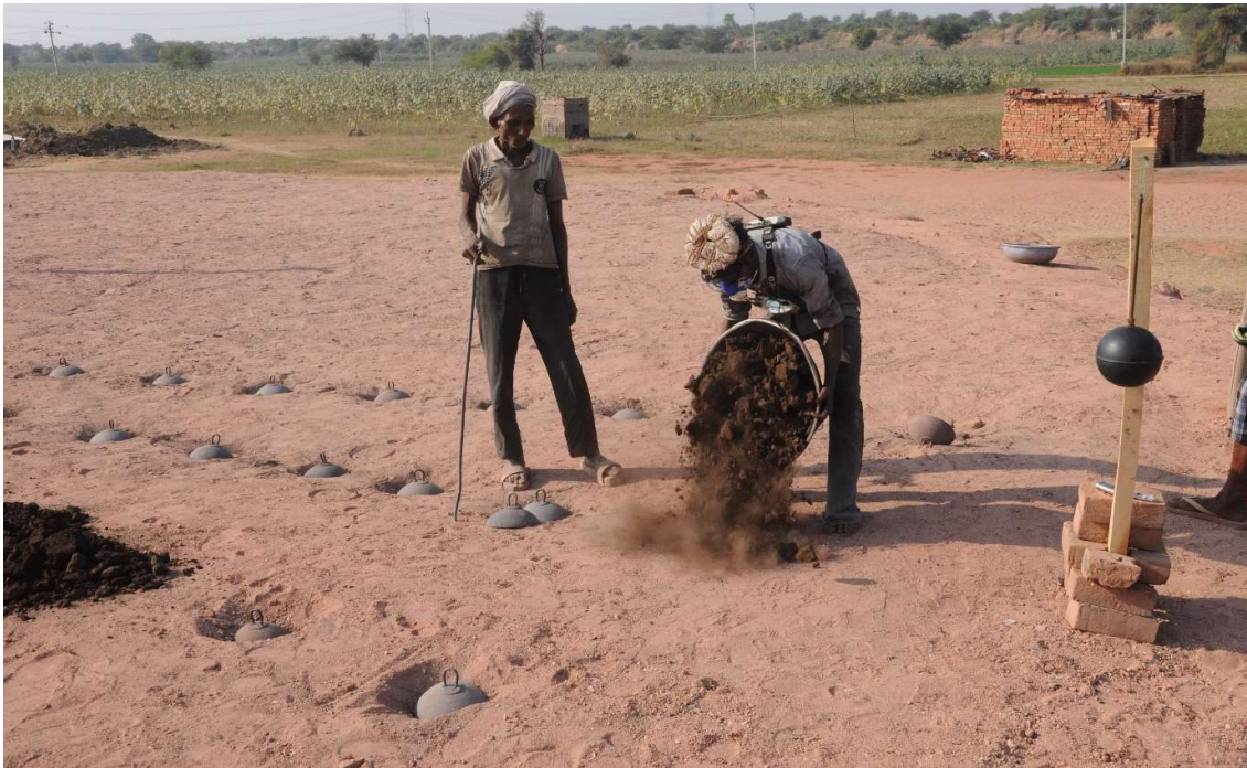
Figure 6-24: Coal charging through the peephole
