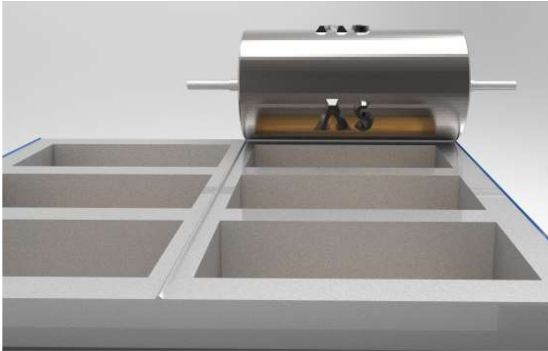
Figure 6-19: Proposed embossment pin for brick-moulding machine
