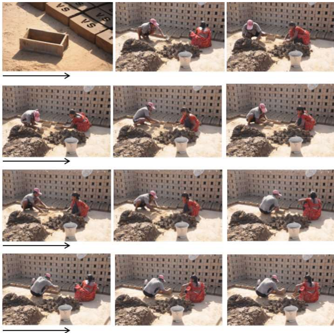
Figure 5-9: Sequence of the brick moulding operation
