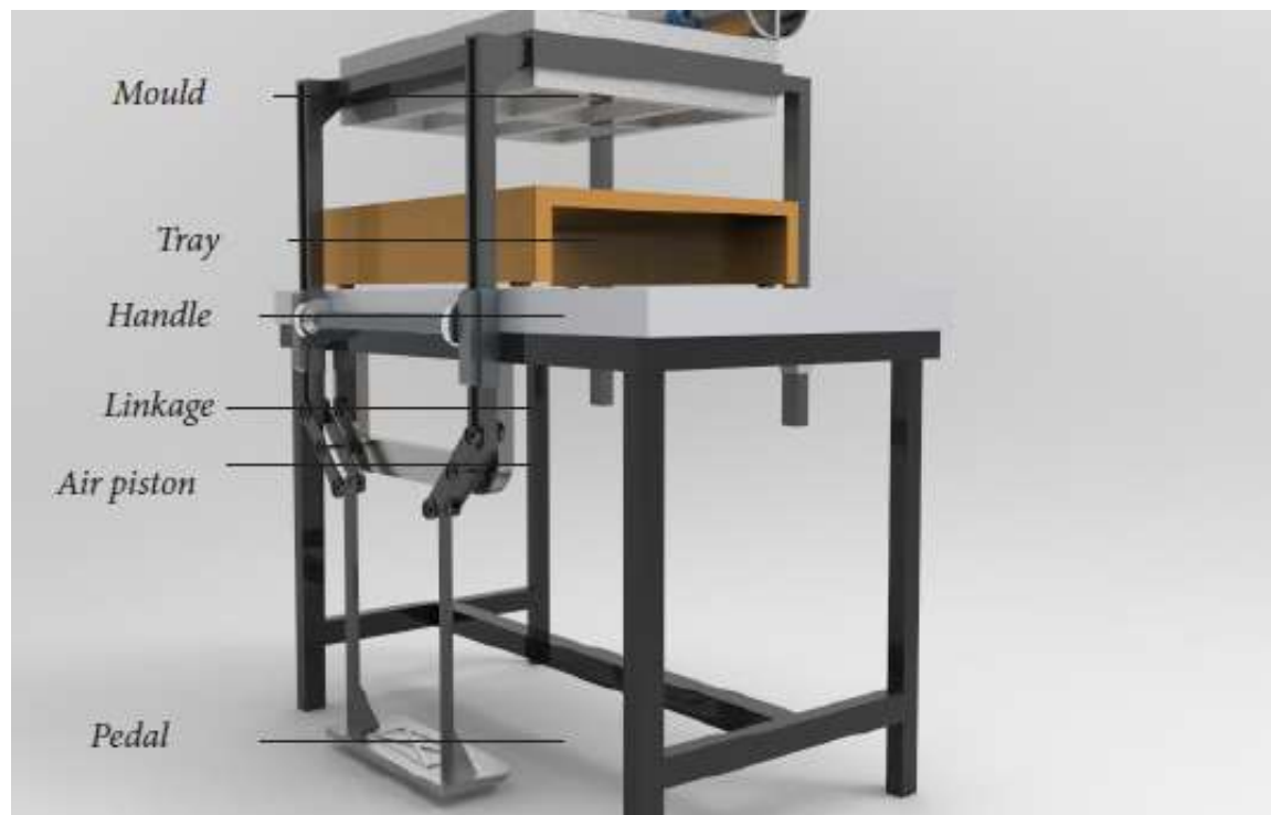
Figure 6-17: Concept model of the brick moulding machine
