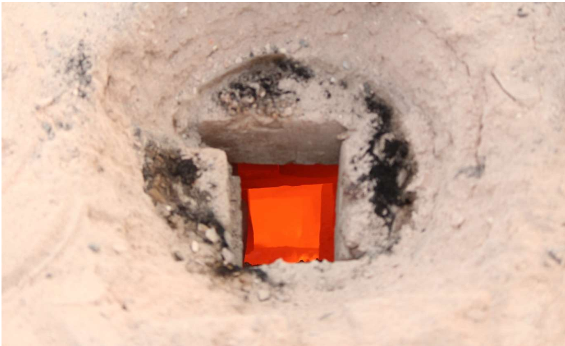
Figure 6-25: Peephole, on the top of the brick kiln
