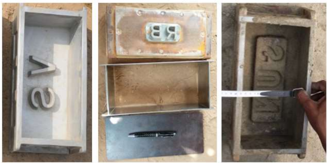
Figure 6-11: Different types of brick-moulding tool
