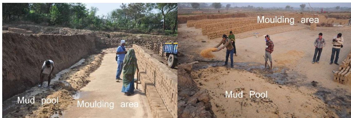
Figure 6-3: Mud pool concept in RB brick kiln industry and VS brick kiln Industry
