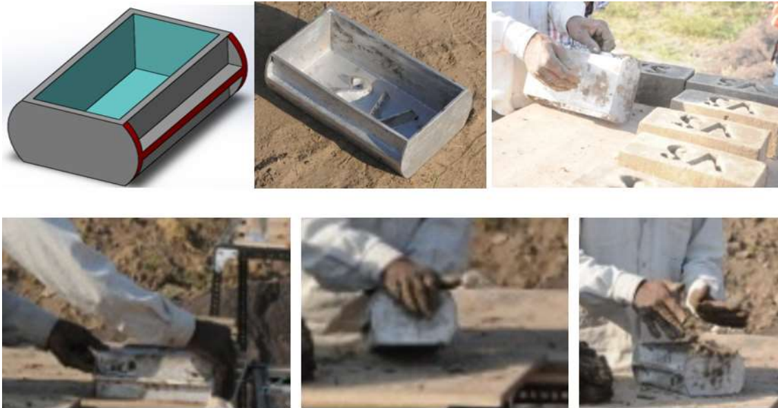
Figure 6-15: Prototype & Solidworks (3D) model with additional grip and high fillet and Actual field testing of prototype
