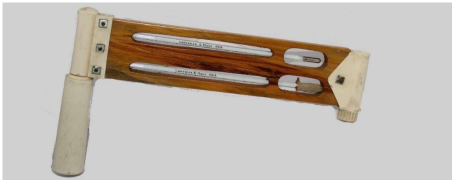
Figure 4-11: Sling psychrometer (Dry bulb thermometer and wet bulb thermometer)
