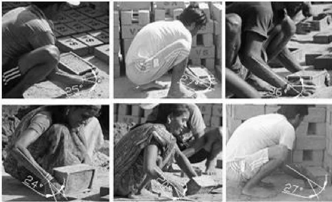
Figure 6-12: Degree of wrist bending during moulding activity of different workers
