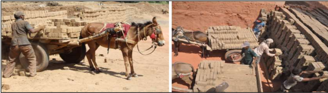
Figure 5-20: Bharai activities in RB brick kiln Industry, Gujarat
