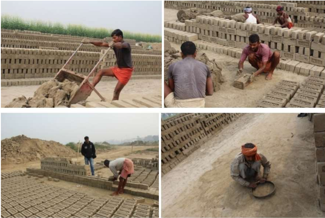
Figure 5-26: Mud transfer and moulding activity in Bihar SUN brick industry, India (Mud Loading in Cart, Mud Transfer by Cart, Toppling of Cart/Unloading mud, Brick Moulding, Stacking the Sun-dried bricks & Ground cleaning activity)
