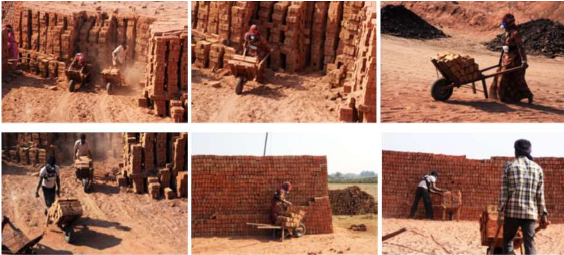
Figure 5-16: Removal of bricks from the kiln
