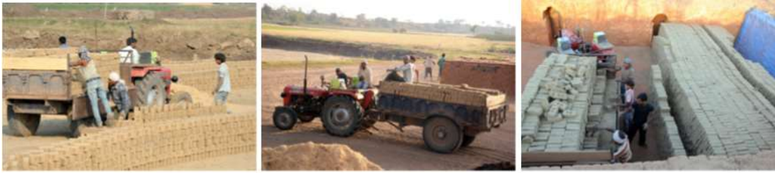
Figure 5-11: Different elements of the brick transfer activity in VS brick kiln Loading of bricks (Left), Transfer of bricks (Middle), Unloading of bricks (Right)
