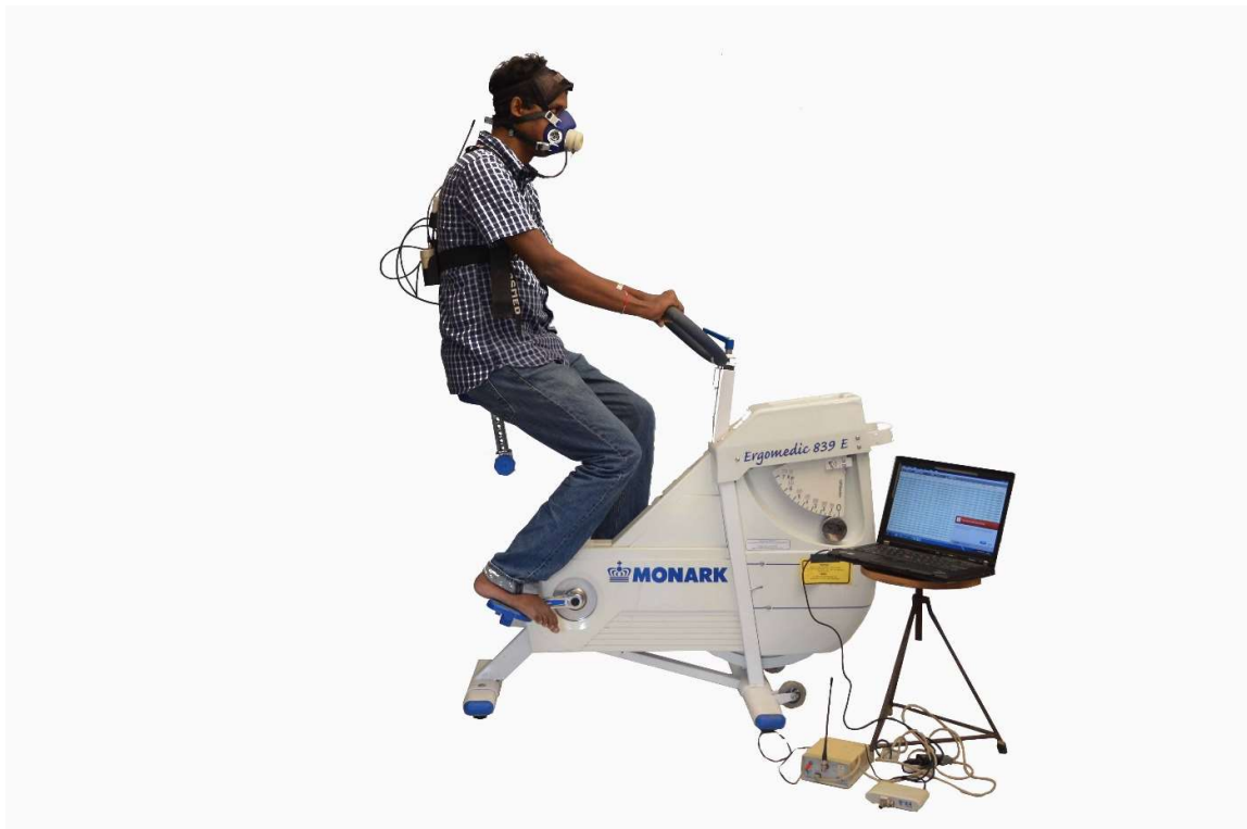
Figure 4-6: K4b2 gas analyser mounting procedure (in Laboratory simulation)
