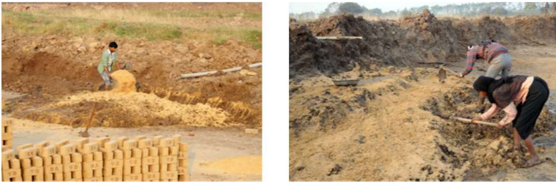
Figure 5-6: Sprinkling of paddy husk (Left), Mud mixing by shovel (Right)
