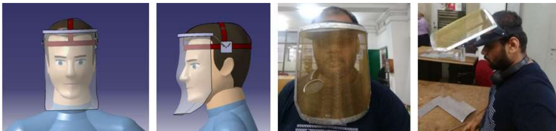
Figure 6-26: Newly designed headgear for brick kiln (Jalaiya) worker (Front & side view)
