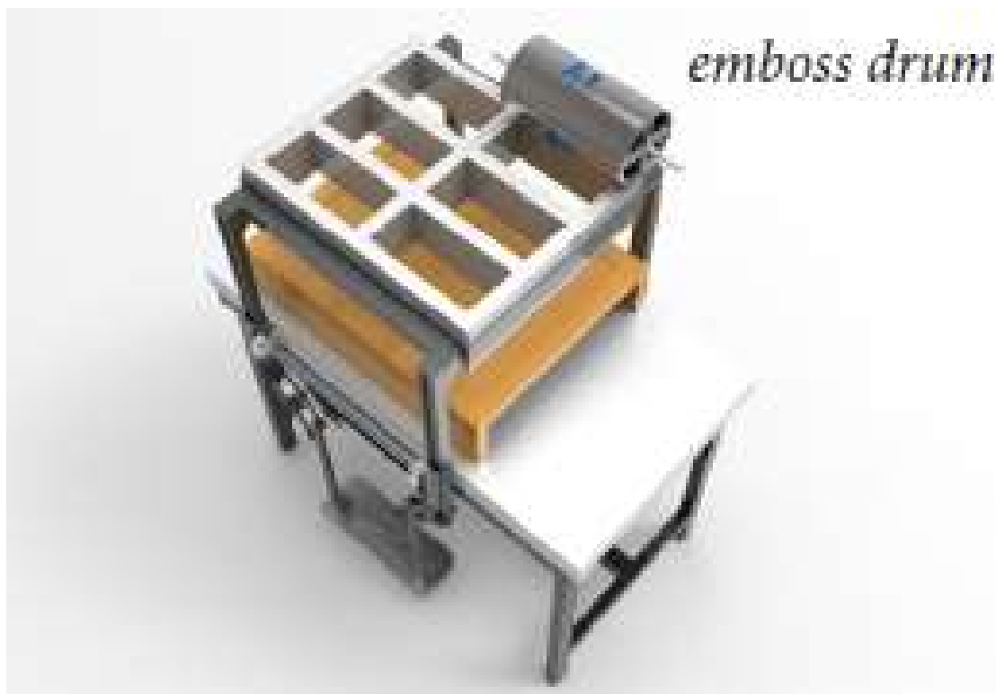
Figure 6-18: Concept model of the brick moulding machine
