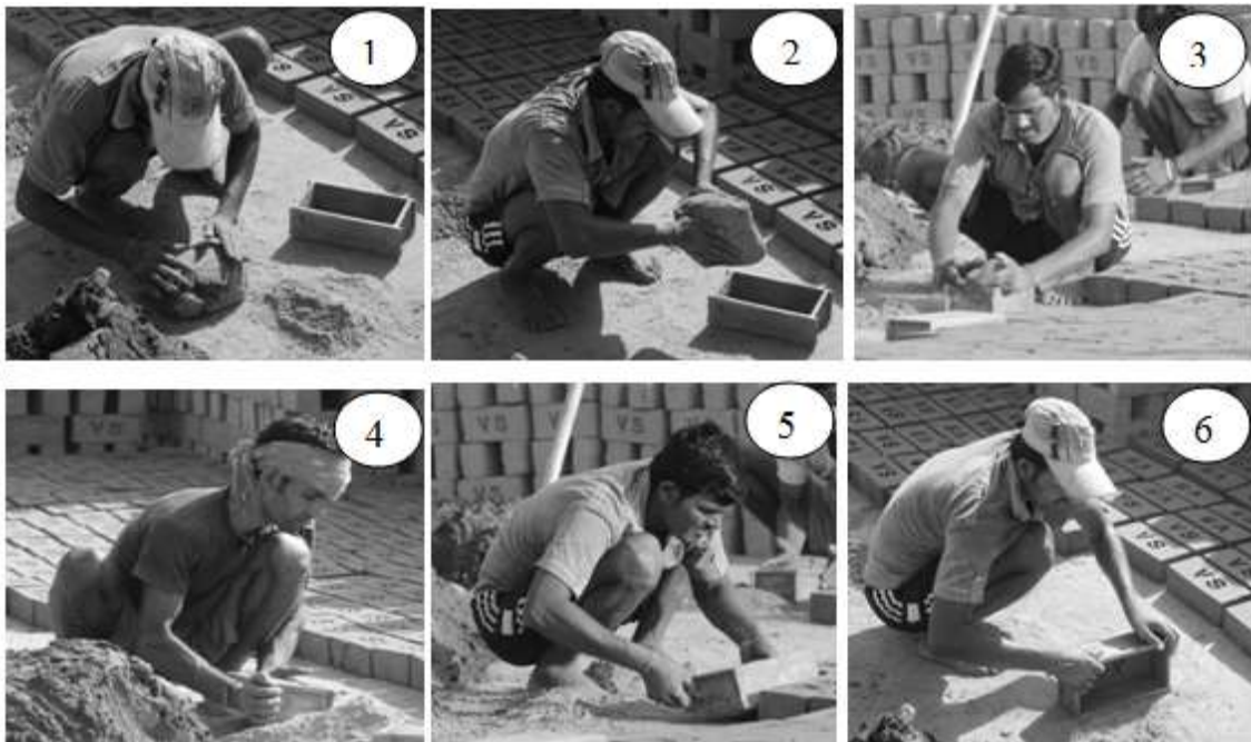
Figure 6-10: Steps of brick moulding
