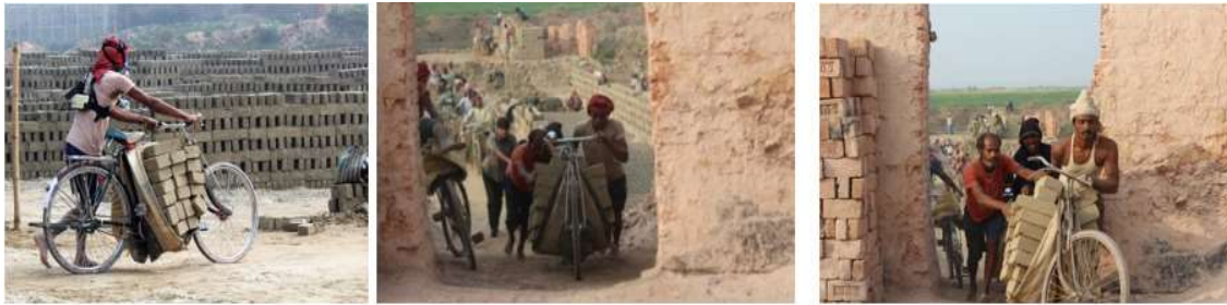
Figure 5-27: Brick transfer (Bharai) activity in SUN brick kiln industry, Bihar
