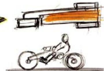
A triangular vehicle platform with three wheels at three corners which can fold to turn into a bike.
