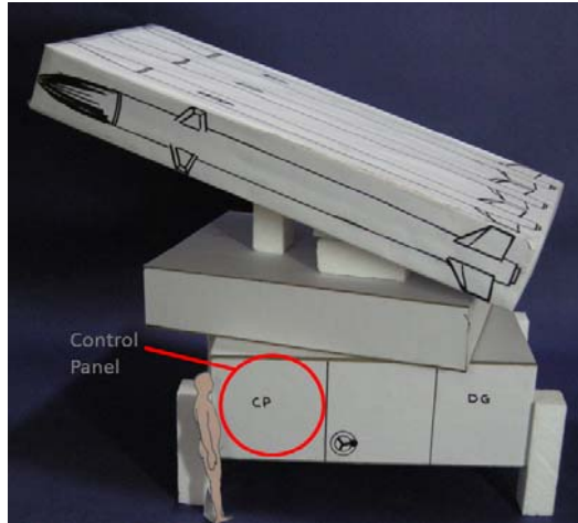
Control Panel on external side of the launcher
