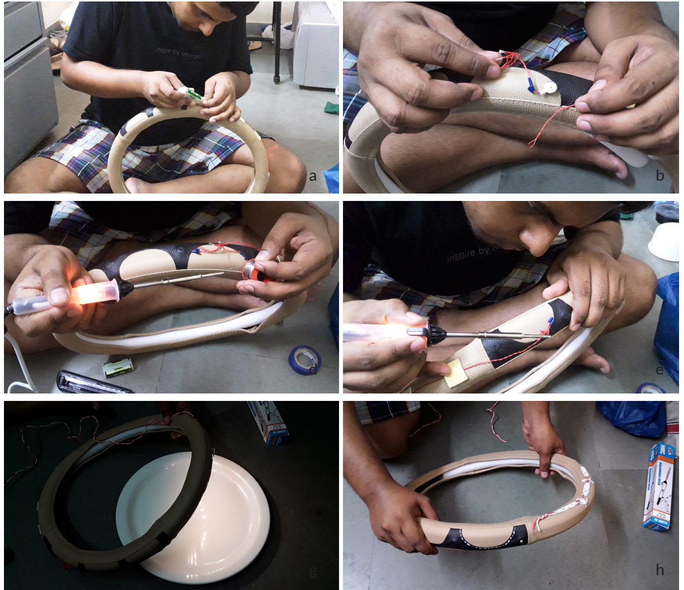
Image 7.19(a-h) - Prototype for Steering Wheel Cover with Vibration Modules & LED Light
