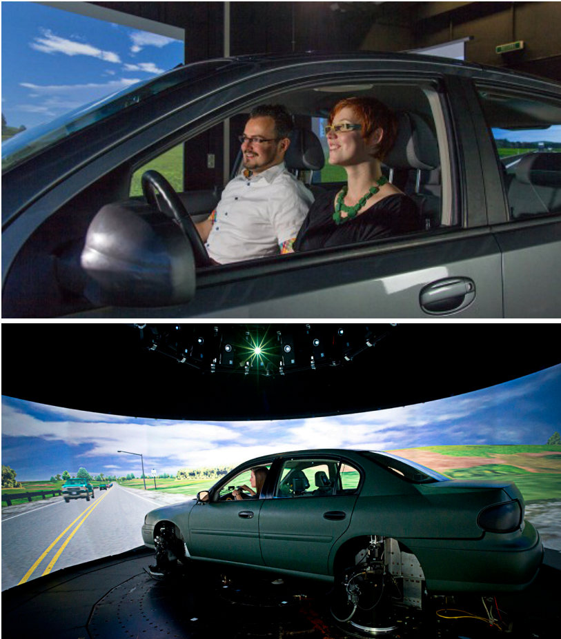
Image 4.3 - Driving Simulator with 180 degree viewing screen
