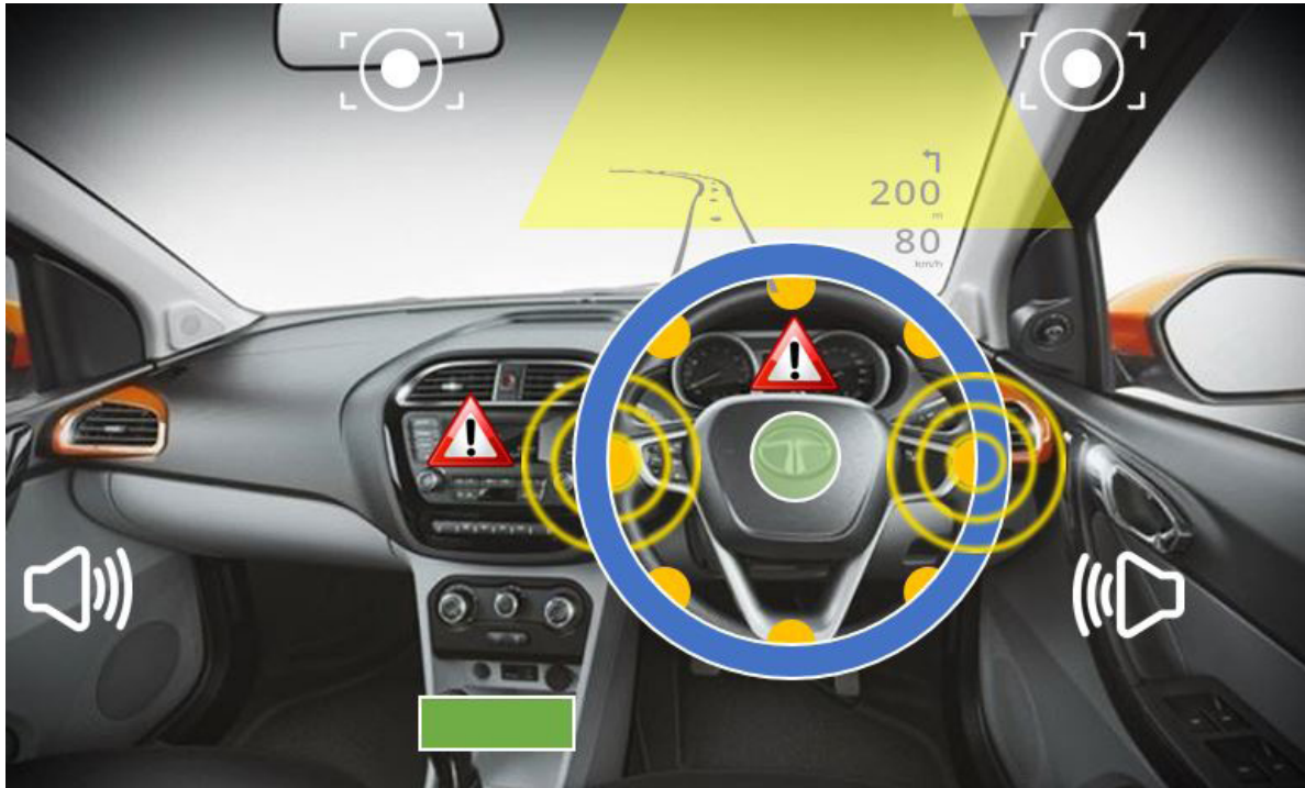
Image 7.7 - Graphical representation of the Drowsiness Prevention System with tentative positioning in the car
