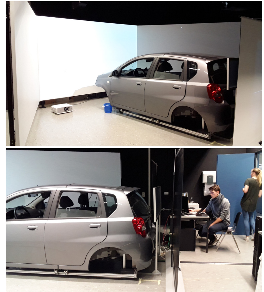
Image 4.4(a) - Driving Simulator at IAD, TU Darmstadt
