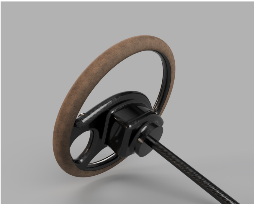
Image 7.23(b) - Steering Wheel Cover with Vibration Units (Rear)
