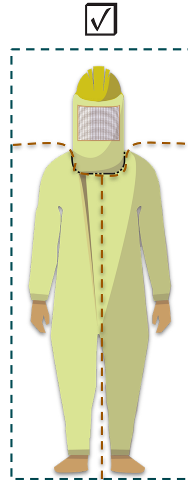
Veil hood attached to the suit using connectors. An 'Unified suit'
