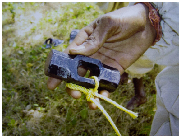
1 Securing a rope for tree climbing by using string and hammer
