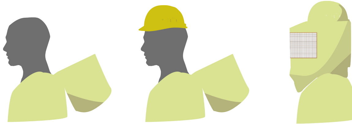
Sequence of wearing the head part of the protective suit
