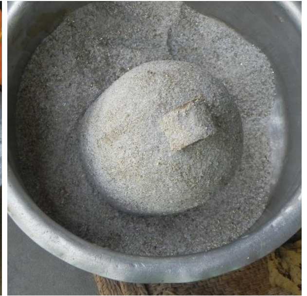
Brass mixture coat on full body of the bell
