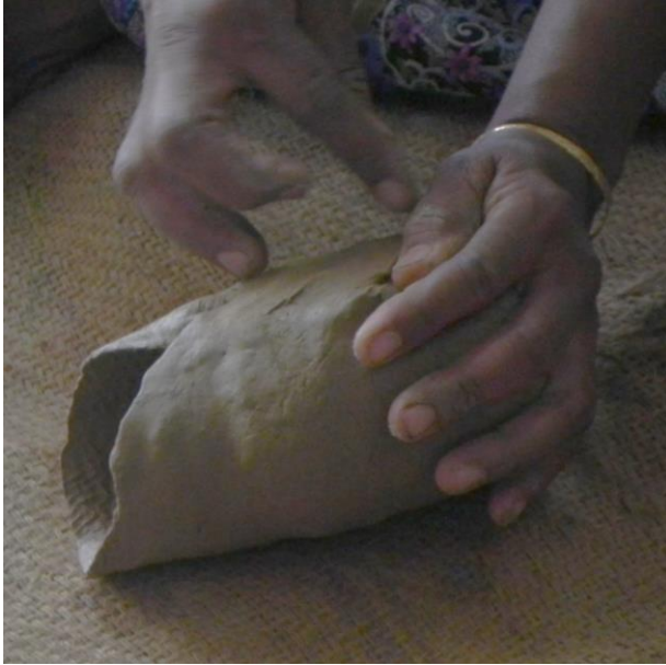
Rolling the bell body over the clay chapati
