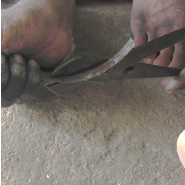
Cutting the kadi from MS metal sheet
