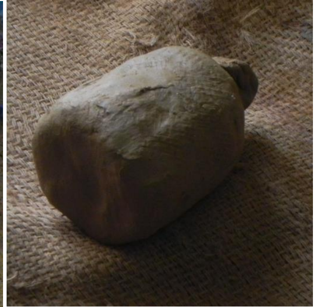
Mud coated bell ready for firing
