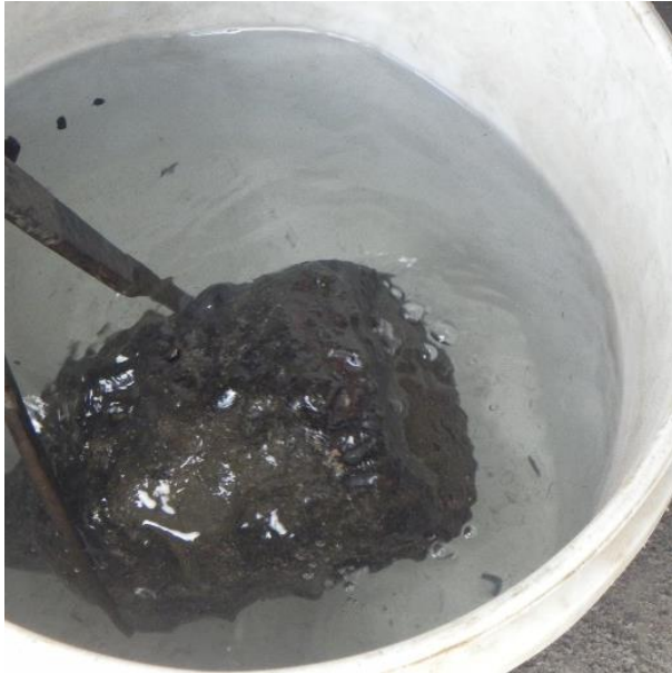
Dipping the bell into normal water to cool it and hence quench
