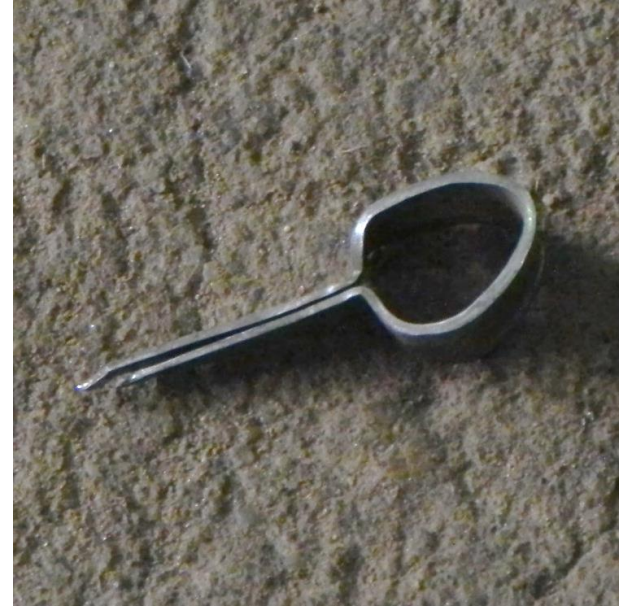
Shaping the sheet into circular hook shape
