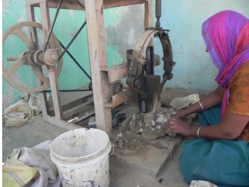
Cotton and mud mixed together using power hammer to get a uniform mixture dough
