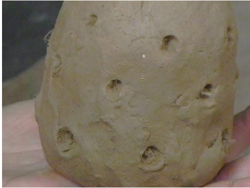
Holes were too small for the bell to burn at that place
