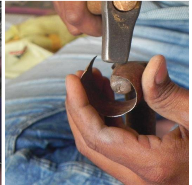
Shaping by hammering on a stone mold using round hammer
