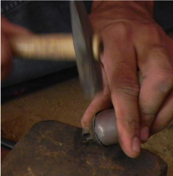
Inserting the kadi in the hole pierced on the topi
