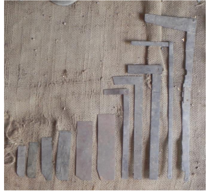
Standard measurements of bhabris of a range of bell numbers
