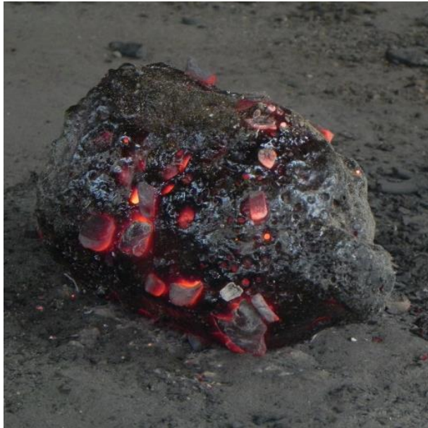
Bell just taken out of the furnace has red hot coal particles stick on its surface
