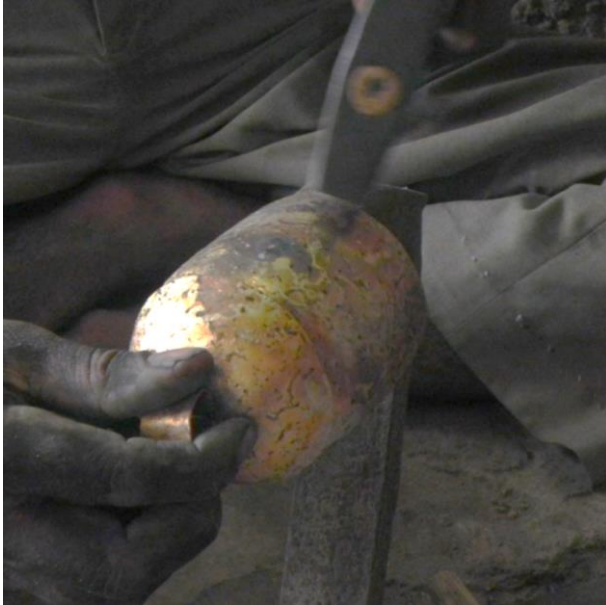
Hammering near the edges
