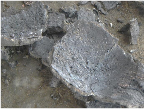
Residual Brass left on the burnt clay
