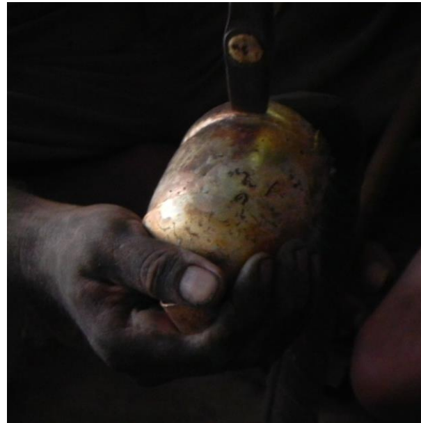
Hammering the crease and checking the sound
