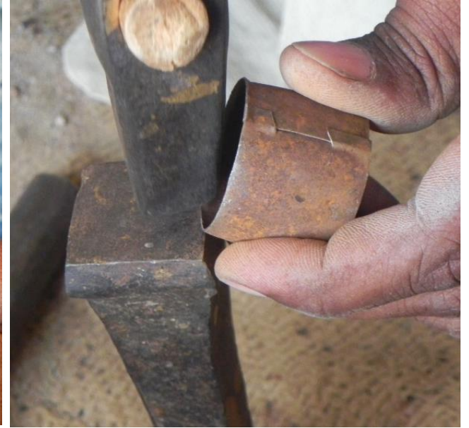
Locked notch made a cylindrical babri
