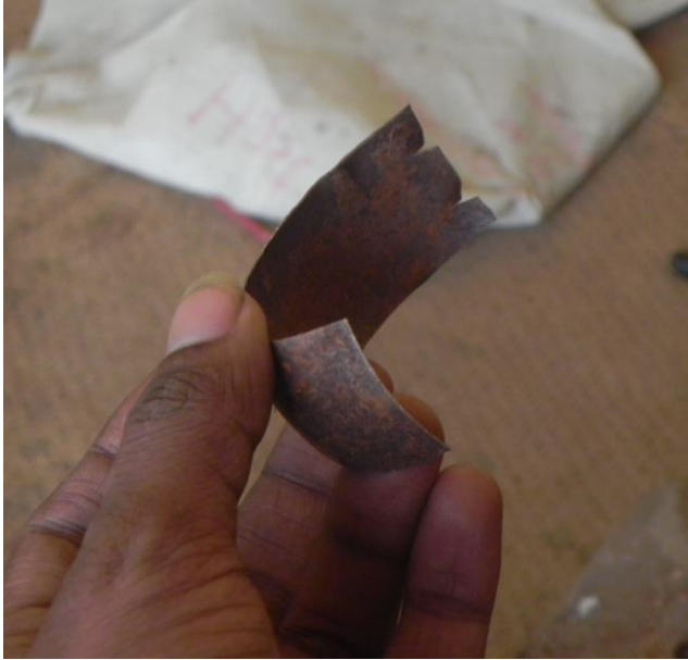
Cutting the notch on babri
