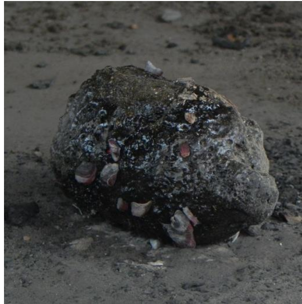
Coating becomes black after keeping for sometime on room temperature
