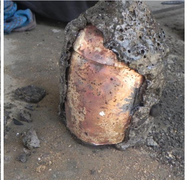
Cracking open the bell coating
