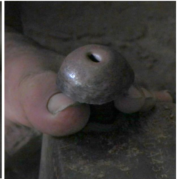
Making a hole in the the topi (Space for putting kadi)
