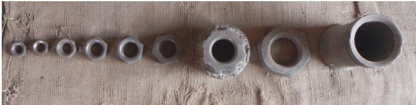
Nuts are used as a mould for making topis
