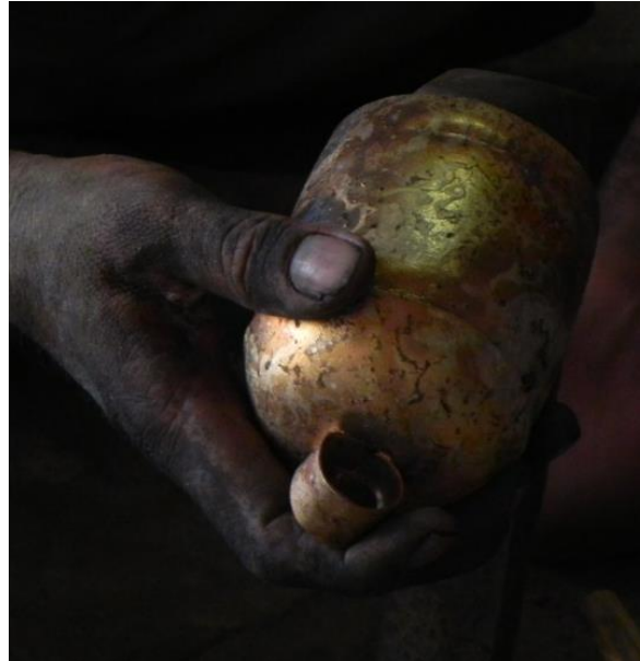
Making a crease at a distance of about 10-15mm from edge
