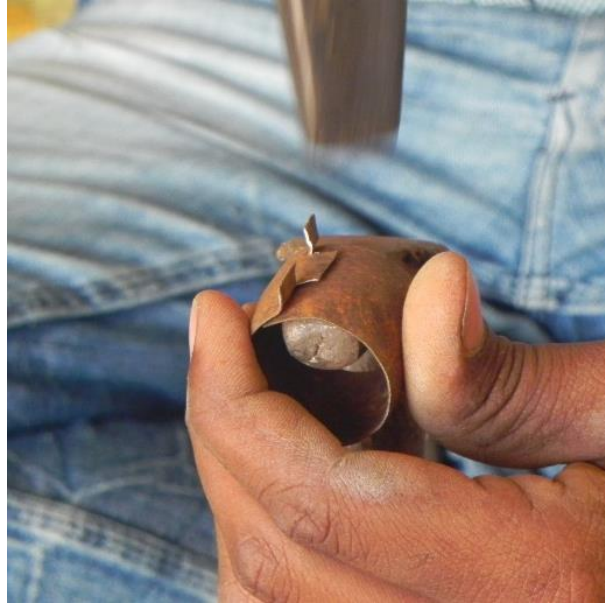
Technique to lock the notch
