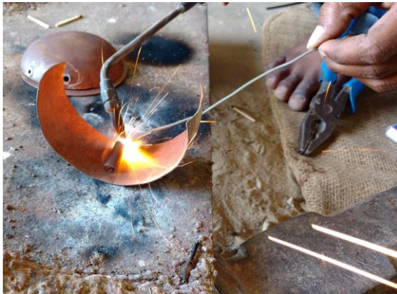
The table bell consists of a swivel base and semicircle bhabri parts. The topi base is of no. 10 and the legs are bhabri parts, having dimensions 1.5*7 inches.
