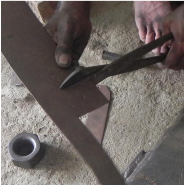
Cutting a circle from metal sheet for topi
