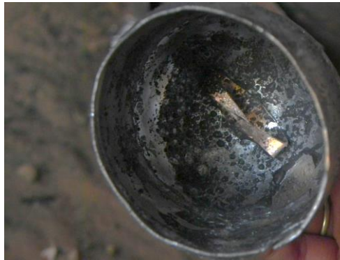
Flux residues stuck inside the bell
