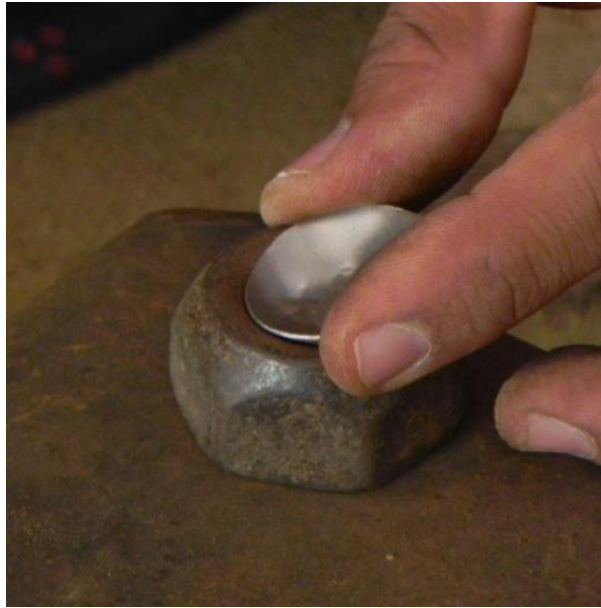
Hammering it to get hollow hemispherical shape
