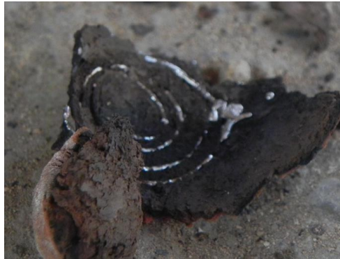
Flux residues stuck inside the bell
