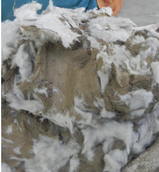
Cotton and mud mixed together using power hammer to get a uniform mixture dough
