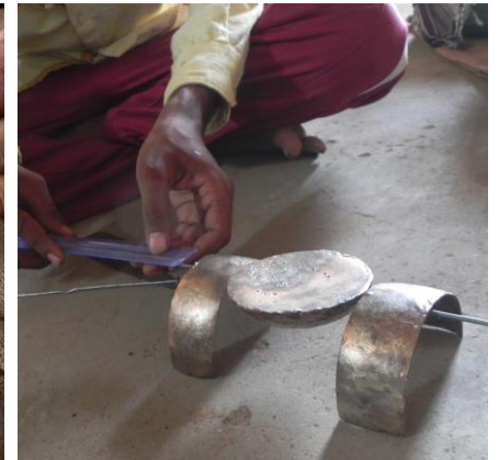
The table bell consists of a swivel base and semicircle bhabri parts. The topi base is of no. 10 and the legs are bhabri parts, having dimensions 1.5*7 inches.
