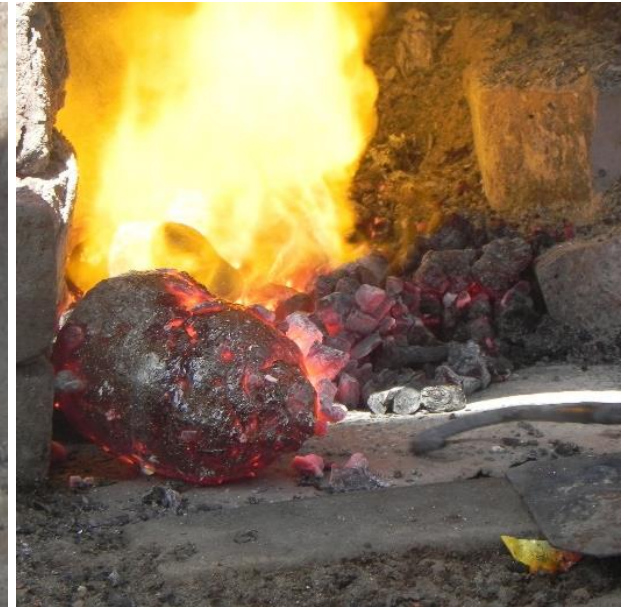
Mud coated bell ready for firing
