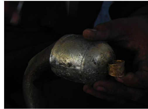
Tuned bell does not ring due to loose joints between its parts
