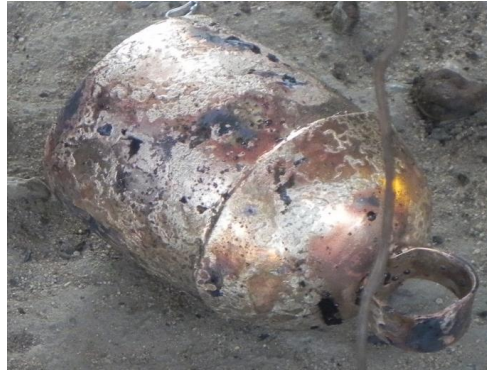
Water went inside the clay cover while quenching resulting in white spots
