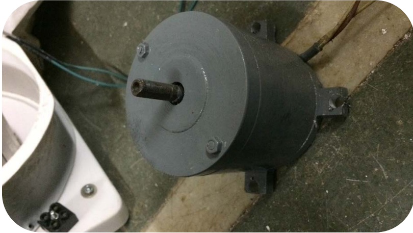
Figure 20: Sample motor shown by the manufacturer, 0.25 hp. AC induction motor
