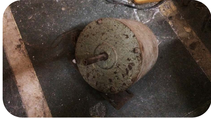
Figure 22: 0.5 hp. AC induction motor
