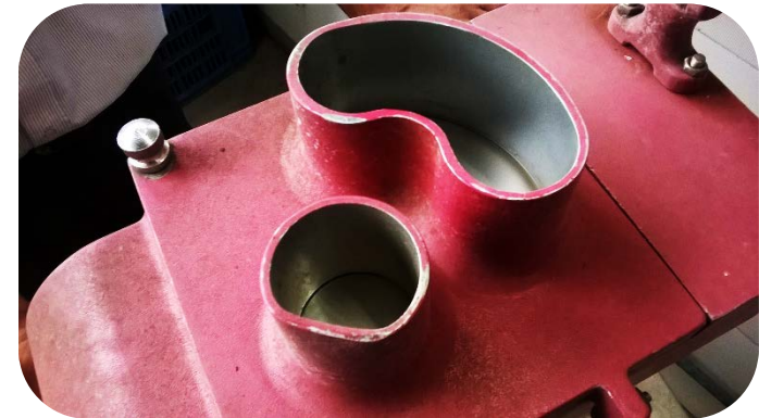
Figure 16: Cast Aluminium Lid of the Vegetable processor showing the inbuilt hopper
