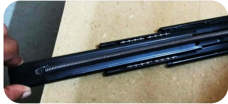
Figure 45 a, b – Sliding Mechanism in drawers with spring
