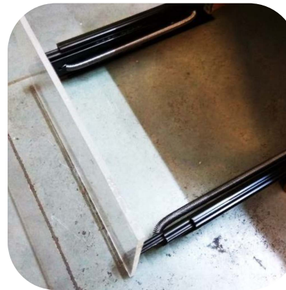
Figure 46 a, b – Spring mechanism tried on mock up model
