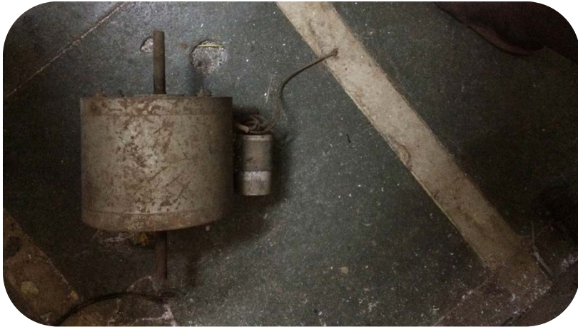
Figure 20: Sample motor shown by the manufacturer, 0.25 hp. AC induction motor
