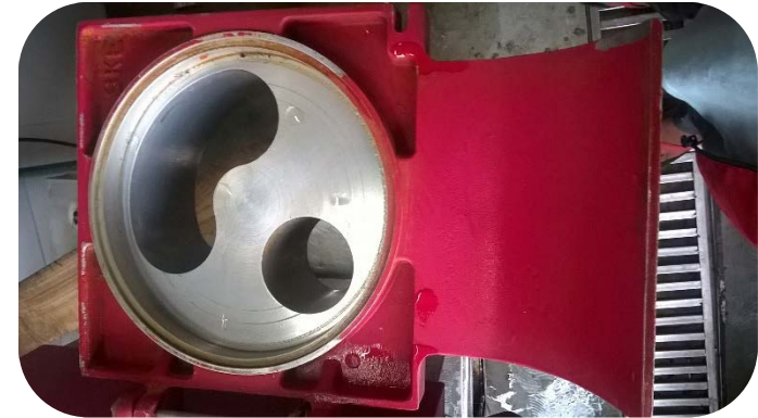
Figure 16: Cast Aluminium Lid of the Vegetable processor showing the inbuilt hopper
