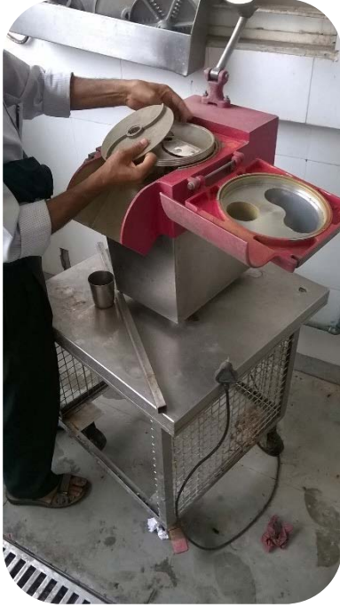
Figure 13: a, b – Demonstration of existing products in Hostel 15, IIT Bombay A basic set of blades come along with the product which includes, one for slicing, one each for slicing and dicing, one for julienning, one for grating and one for French fries. These are stored in a tray provided along with the product.
