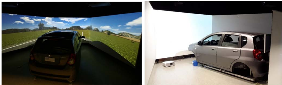
Figure 4.1: Driving simulator IAD (IAD TU Darmstadt)
