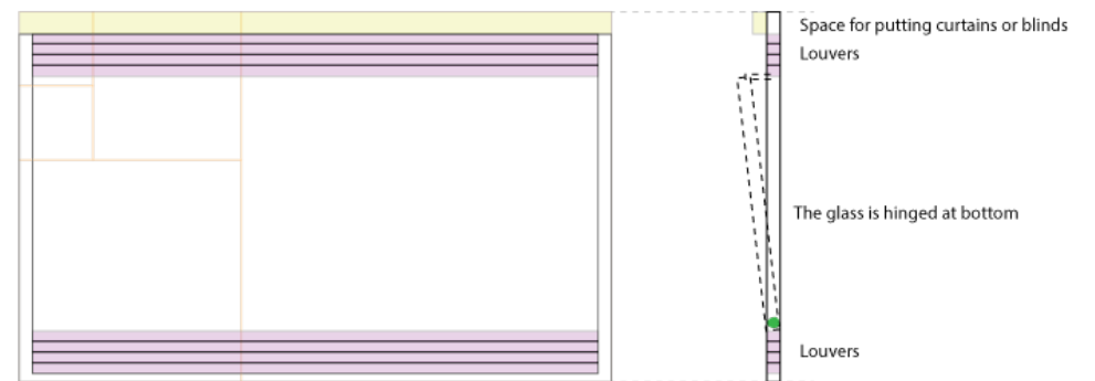
Fig 39: Horizontal pivoted window (at the end)
