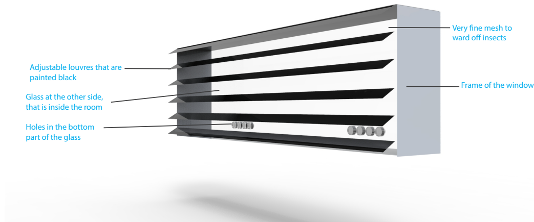
Fig 35: Air-flow in the house with louvered windows
