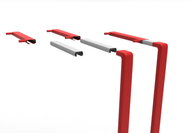
Fig 65: Assembly of the window pane frame
