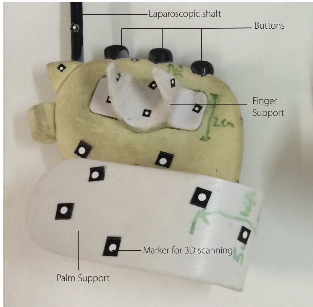
Fig. 29: 1:1 scale mock-up for 5th percentile palm
