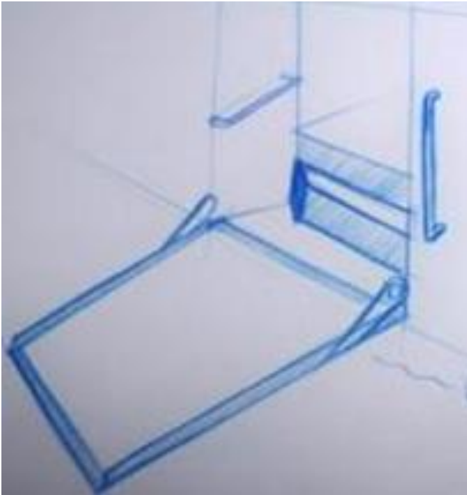
Door convert into ramp
