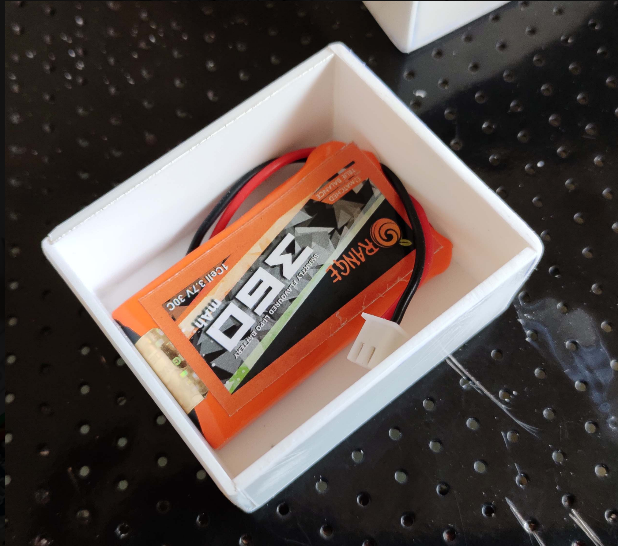
Casing—material: styrene—made for the prototype
