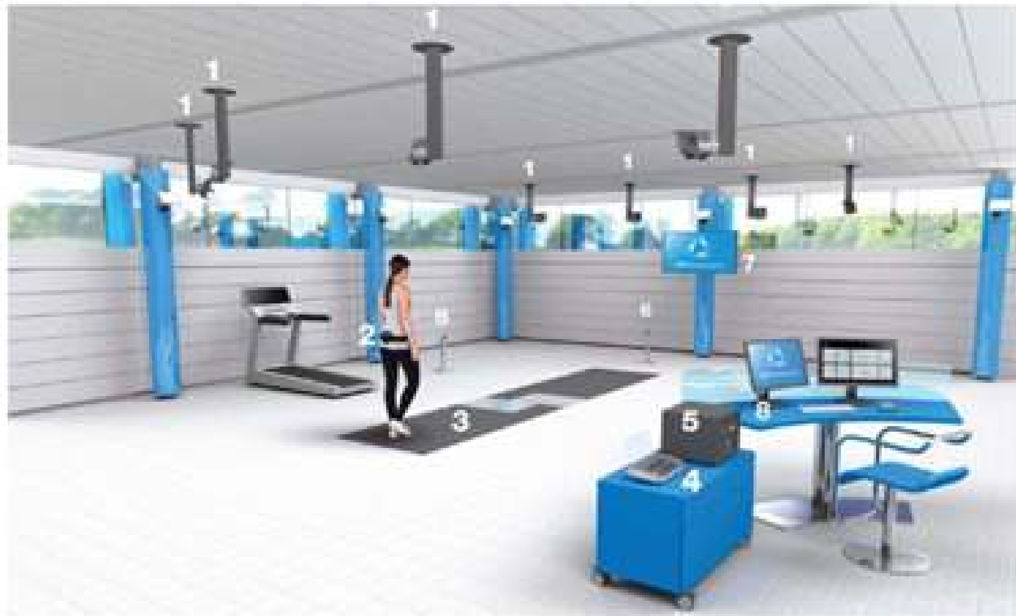
Figure 11. Example of NWS system: BTS GaitLab configuration. (1) infrared videocameras; (2) inertial sensor; (3) GRF measurement walkway; (4) wireless EMG; (5) workstation; (6) video recording system; (7) TV screen; (8) control station. Reproduced with permission from BTS Bioengineering.
