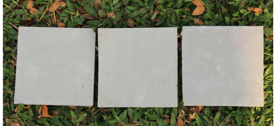
So either press them by keeping some weight on the corners or reverse the tiles at regular interval of an hour to prevent them from curving. Then leave them for drying. They are supposed to be handled very carefully as even slightest jerk could break them. They are very fragile till they are bisque fired.
