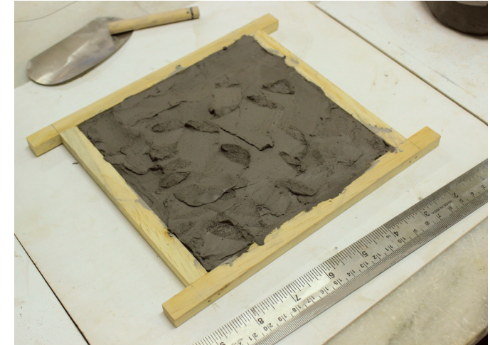
Keep the frame on a foam board or on a newspaper and fill the frame with the kneaded clay.
