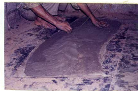
Preparing the clay slab, on the jute surface
