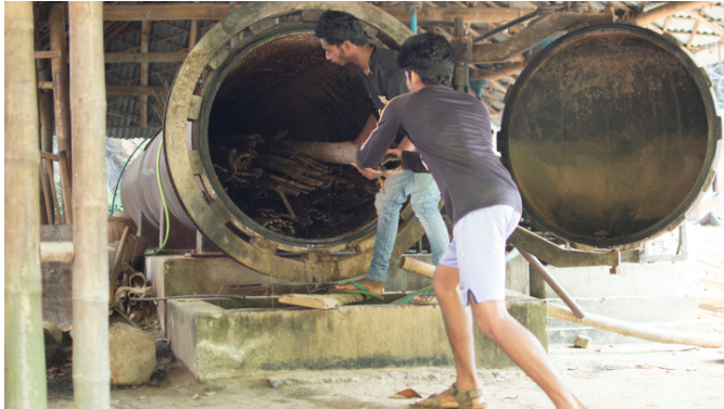
Fig.33: Gas pressure impregnation
