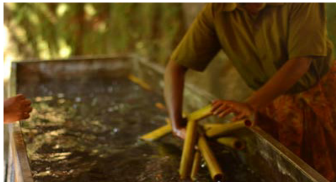
Fig.35: Hot dipping - retrieving treated bamboo
