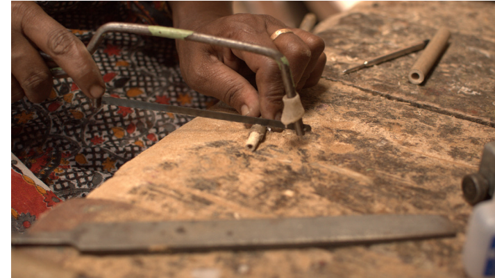
Fig.48: Cutting the snug fit part
