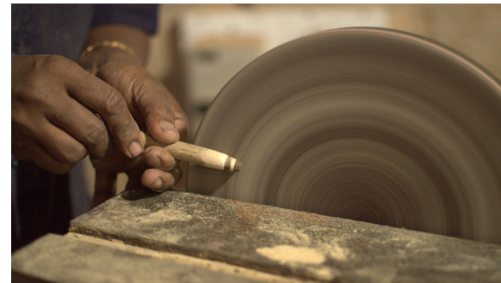
Fig.49: Sanding for finish near grip area
