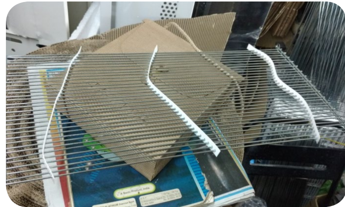
Teflon strips helps in keeping conducting rods equidistant and they are resistant to high current/spark. A gap of 6-5mm has to be maintained between
